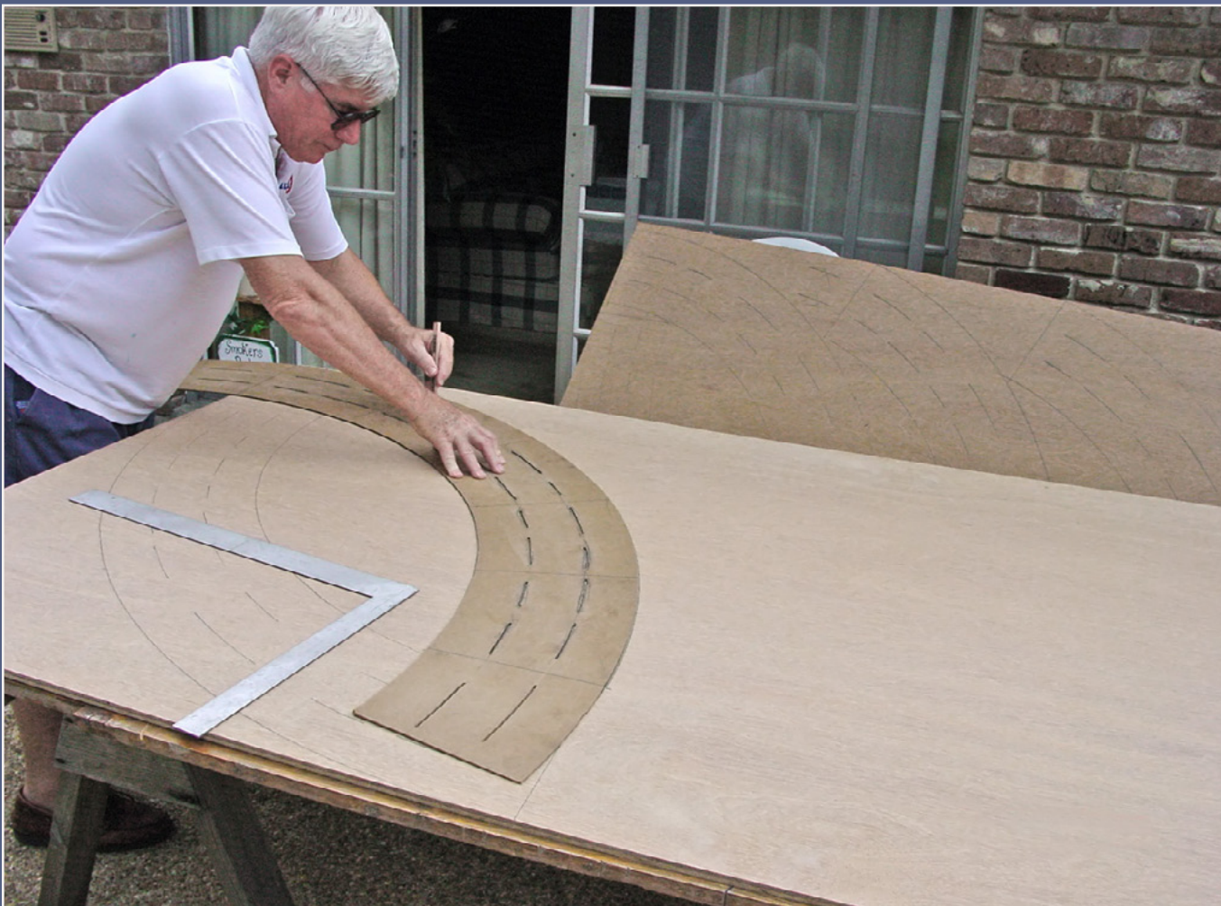
Figure 4: Assistant Dave Abramson marks the 1/4" lauan plywood with all the sub-roadbed pieces, using the template as a guide.
