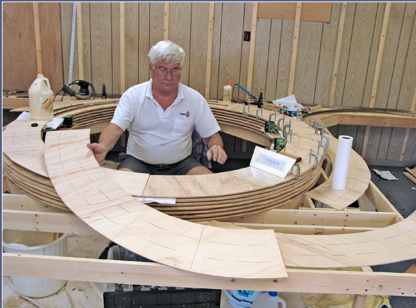
Figure 7: Able assistant Dave Abramson laminates each tier-loop, leaving the one laminate joint between each tier-loop unglued to allow easy disassembly of each loop later for doing the trackwork. Notice how Dave is offsetting the joints between the two 1/4" laminated layers by about 50%. The result will be a strong 1/2" helix sub-roadbed with no splice plates.
