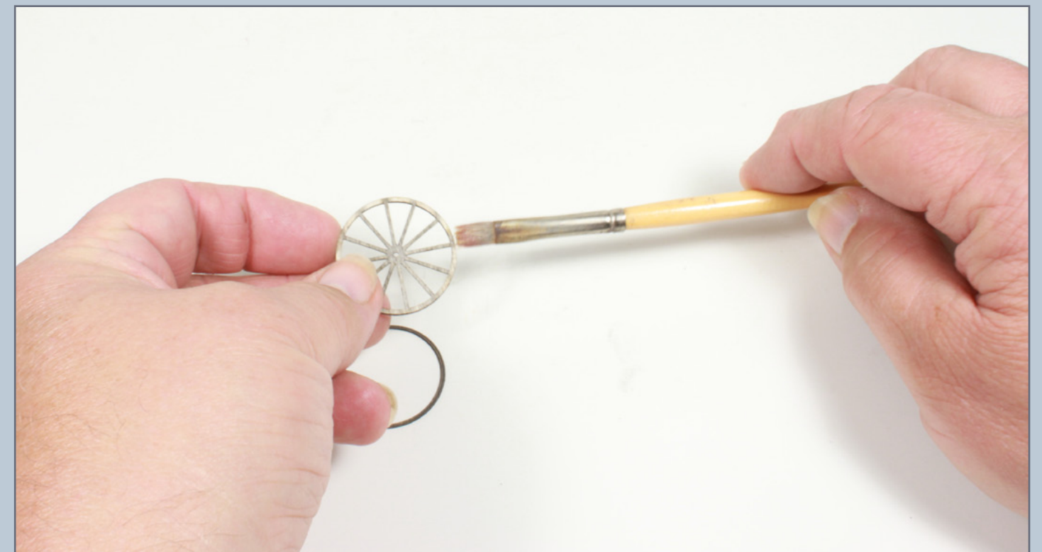
Figure 8: A very light coating of dilute white glue will permanently attach the rims to the wheels.
