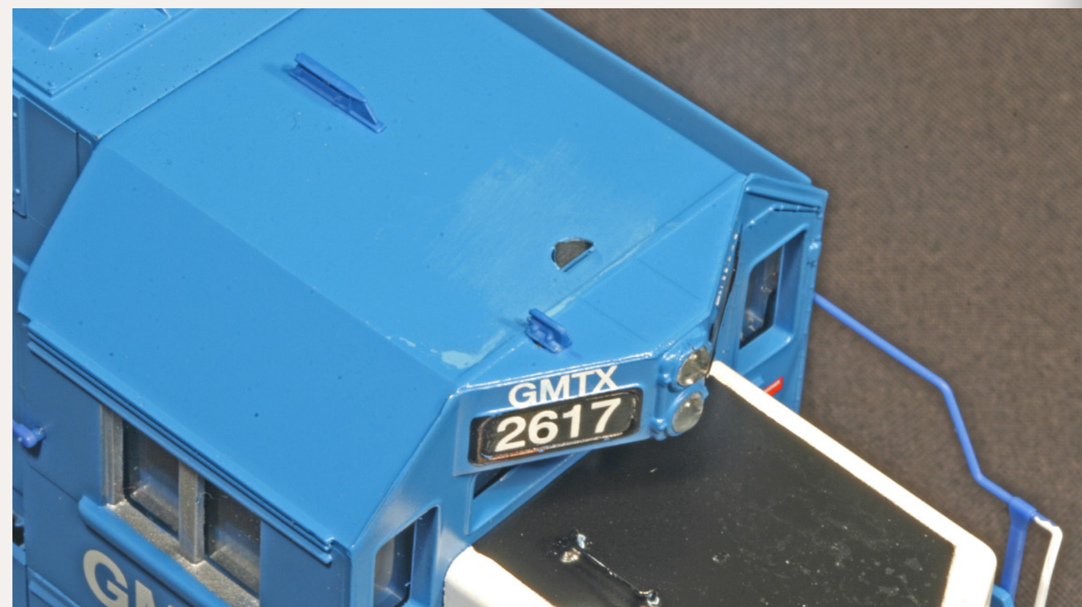
Figure 5: After cutting off the factory air horn, Matt left the mounting stem in the hole to fill it. A little putty and paint will hide the hole completely.
