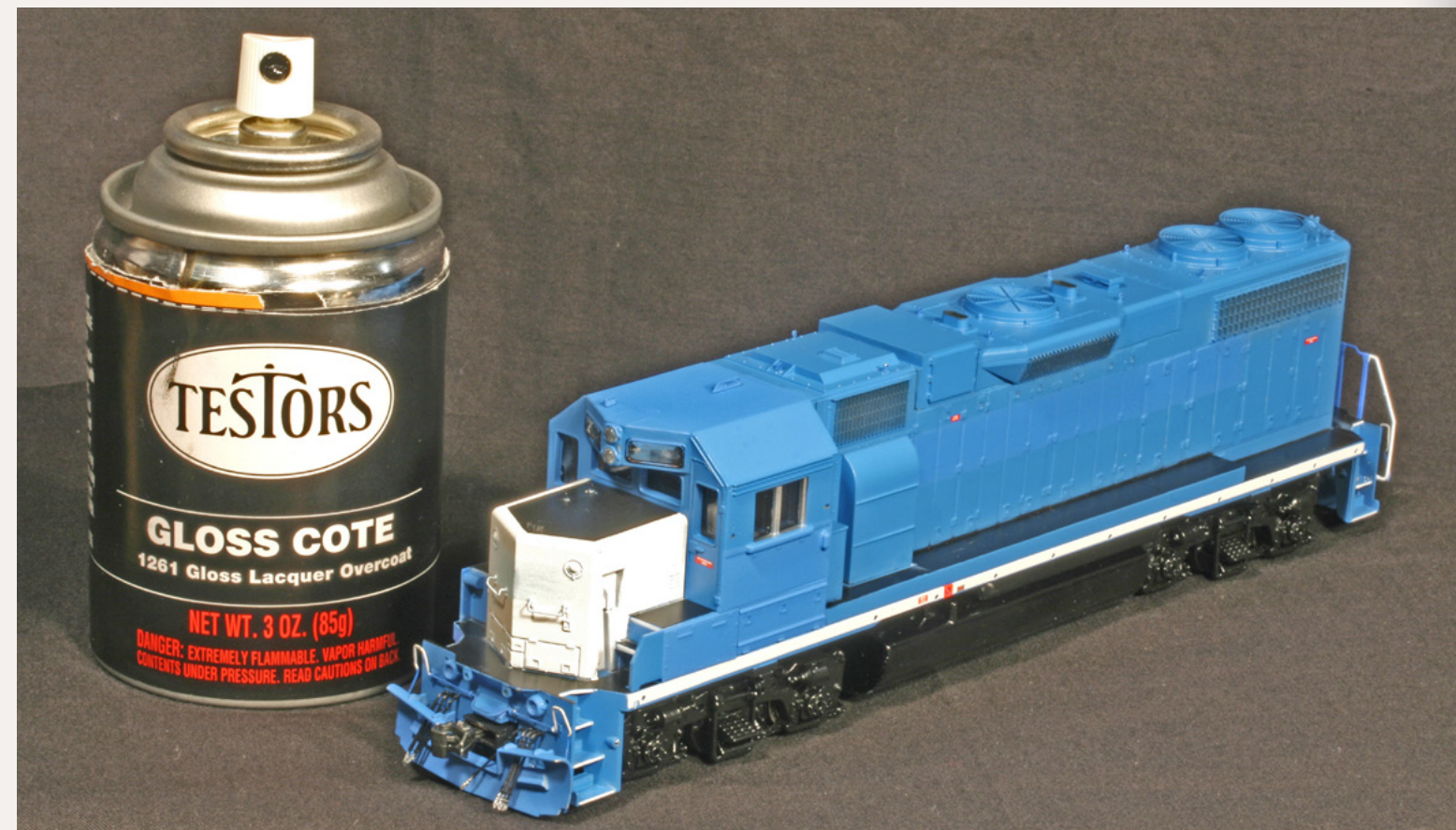
Figure 19: Matt sprayed the model with Testors’ Gloss Cote to prepare it for decaling.
