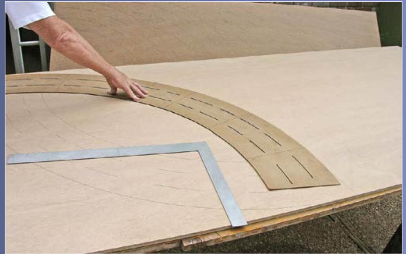
Figure 3: Art added marks every 22.5° to the template to aid in making curve sections as long as needed on the plywood.
