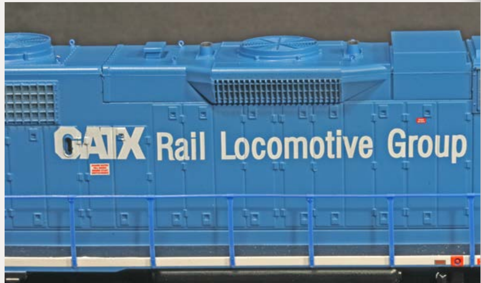
Figure 10: Removing the lettering from the hood area using the sandpaper strips is more challenging, since the body shell is so uneven.
