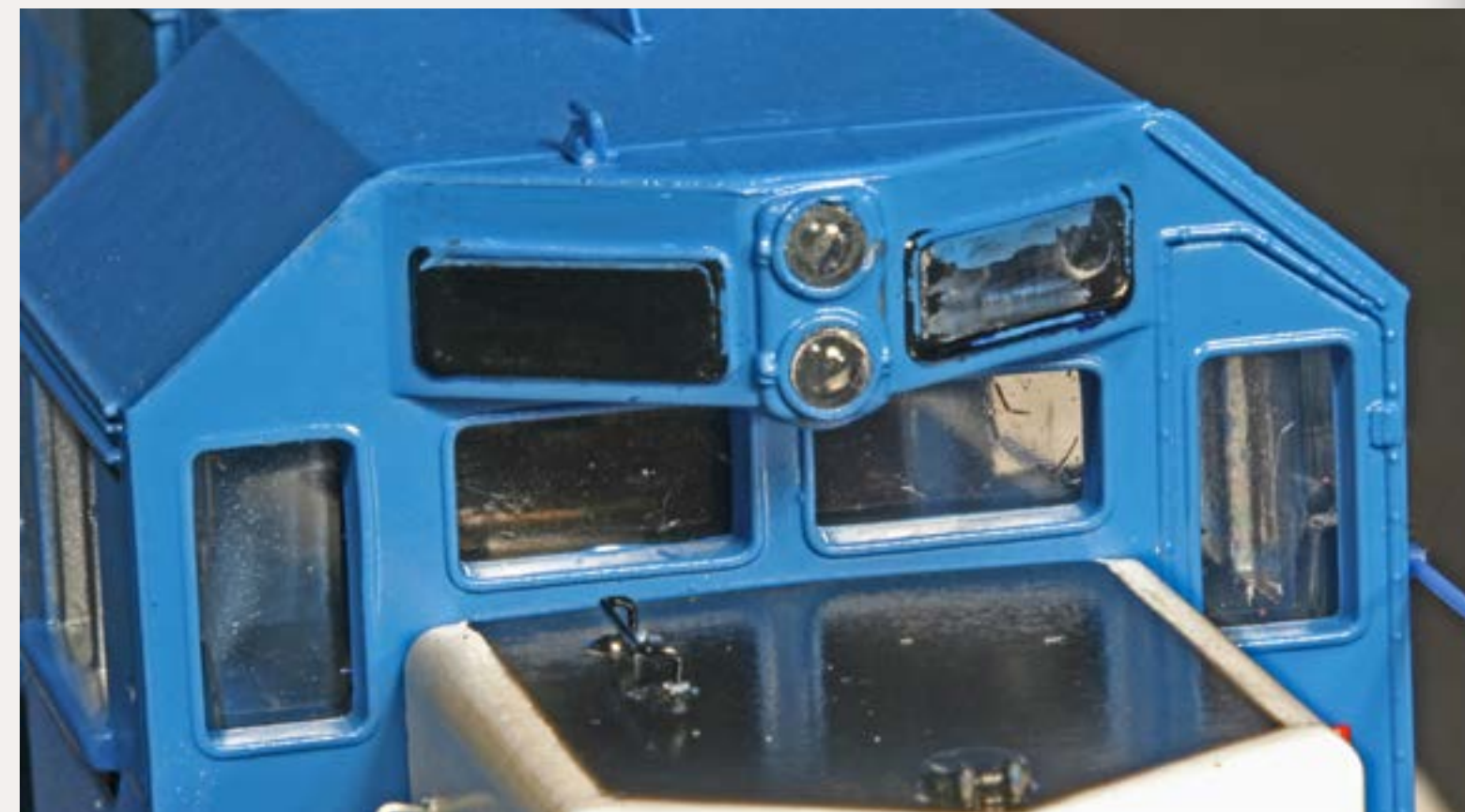
Figure 20: On evening three, Matt applies Shellscale numberboard decals to the loco’s number boards.
