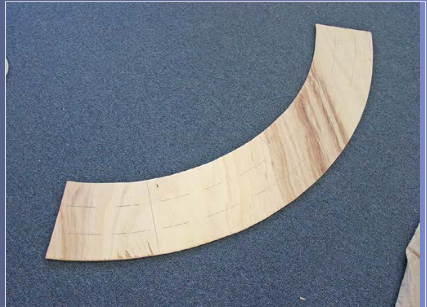
Figure 5: A section of cut out sub-roadbed for the helix. Art cut 81 such pieces of sub-roadbed for this 10-turn helix.
