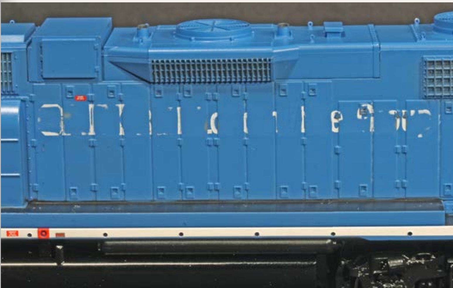
Figure 11: Here's the result after Matt wet-sanded the hood sides with the 1500 grit sandpaper. Remnants of the original lettering remain.
