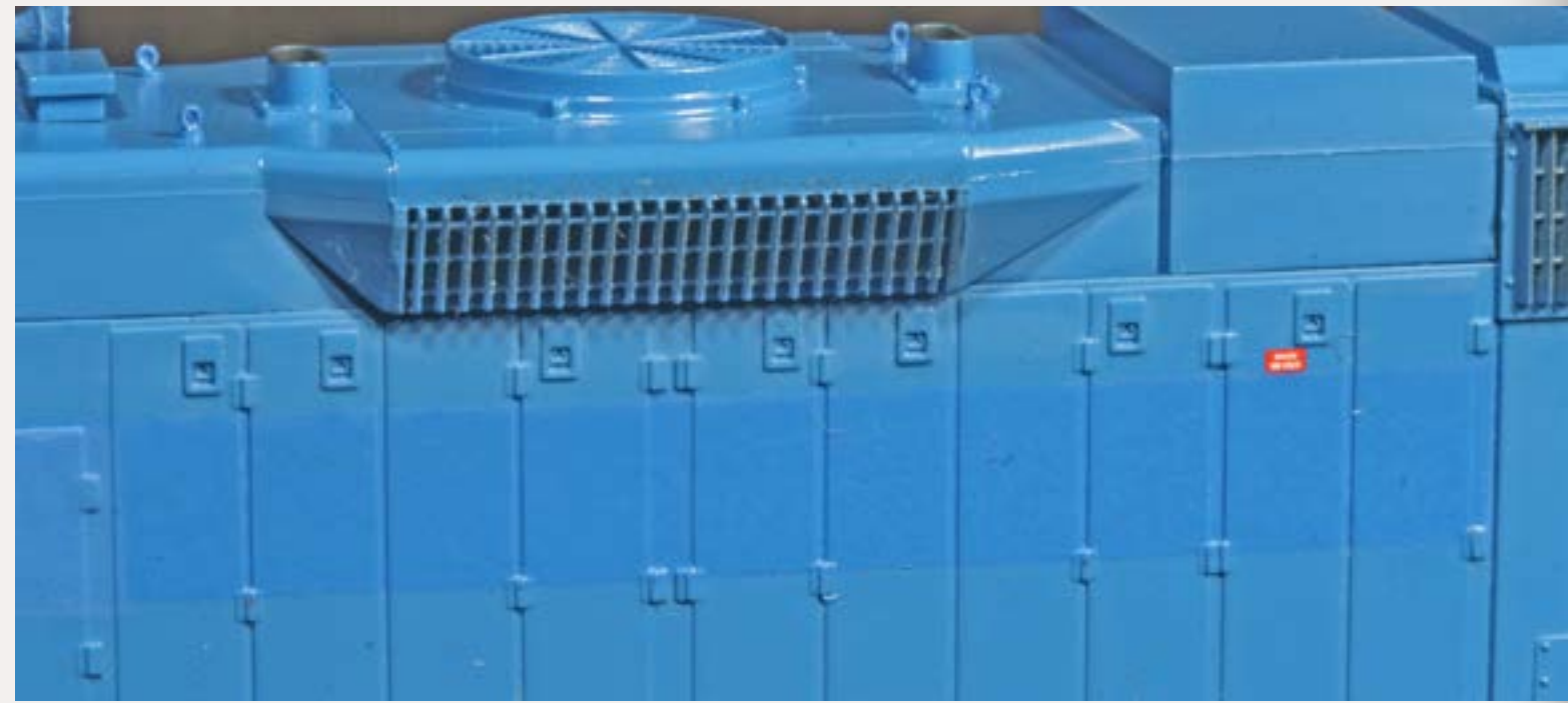
Figure 16: After masking and spraying the hood side, here's the result. Matt deliberately used a paint one shade darker than the model to get the hasty patchwork look of the prototype paint job.
