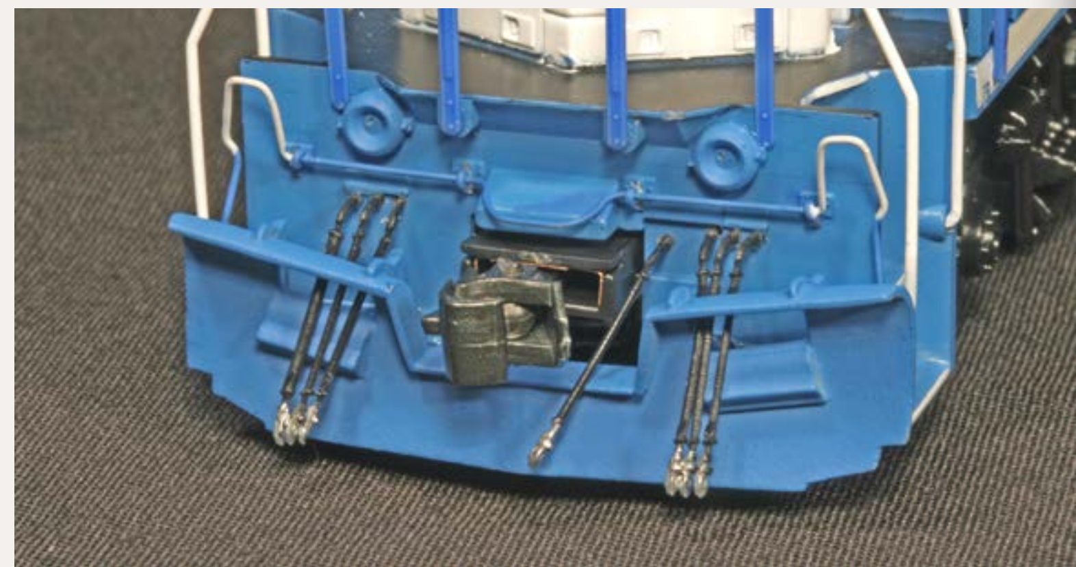
Figure 7: Matt installed ditch lights, coupler lift bar, train air line and MU hoses to the loco pilot – transforming this model into one specific to the BNSF prototype.
