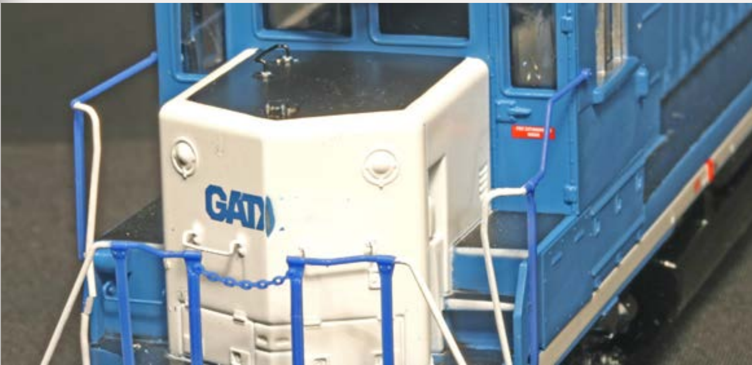
Figure 14: Wet-sanding the nose to remove the lettering also works quite effectively, with little if any damage done to the factory paint.
