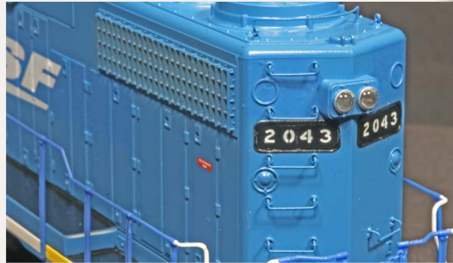
Figure 22: Matt applied number decals onto the black Shellscale number board backgrounds.
