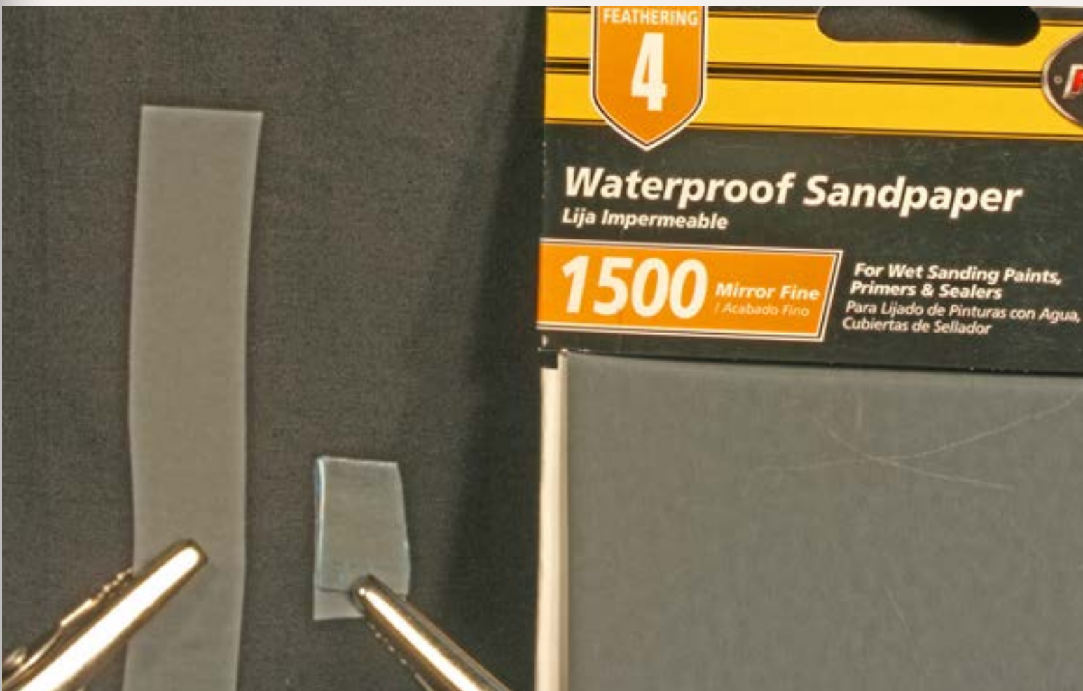
Figure 8: Matt cut narrow strips of 1500 grit automotive sandpaper to use for evening two's paint removal tasks.
