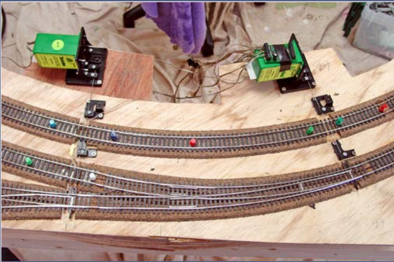
Figure 10: You must side-mount switch machines in a helix, since there's no room under the sub-roadbed for them.
