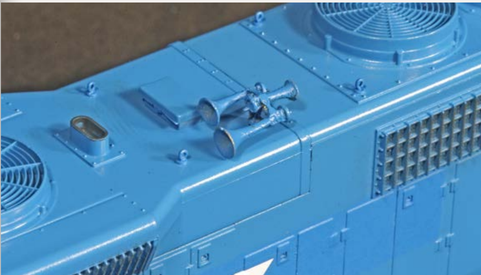
Figure 6: Matt added an after-market air horn mid-hood to match the BNSF prototype. Matt also added lift rings to the hood.
