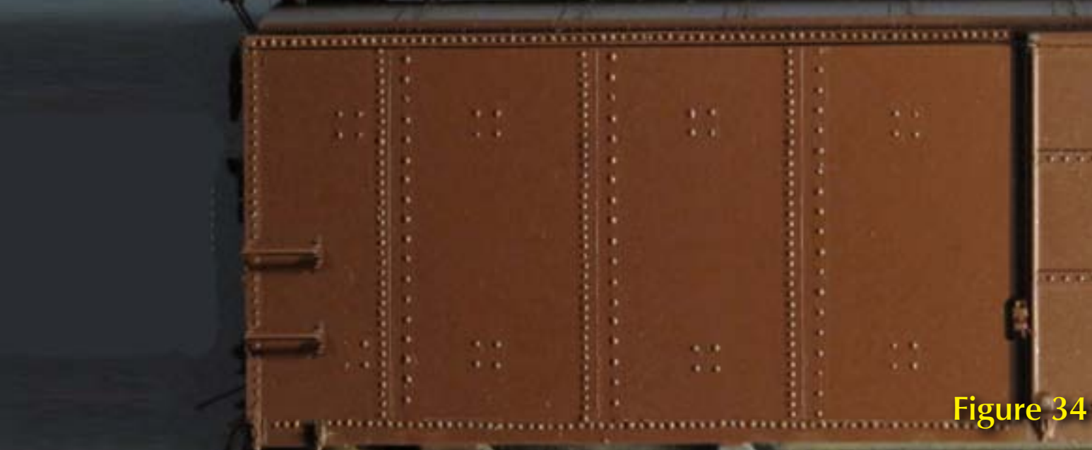
Figure 34: Micro-Mark rivets on an 8-panel boxcar conversion.
