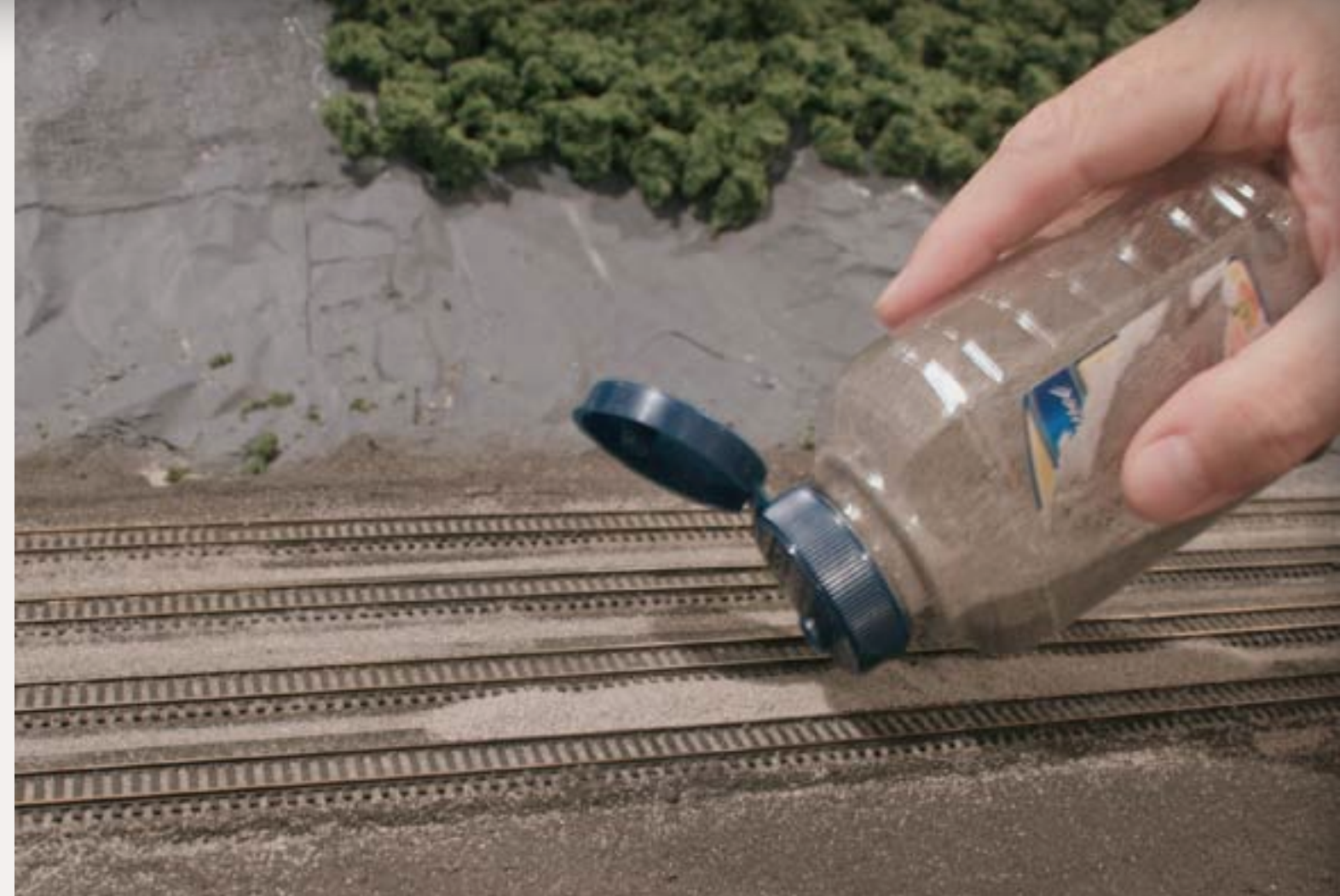
Figure 3: Ballast can be applied using a small bottle, folded index cards or with a variety of commercial products.
