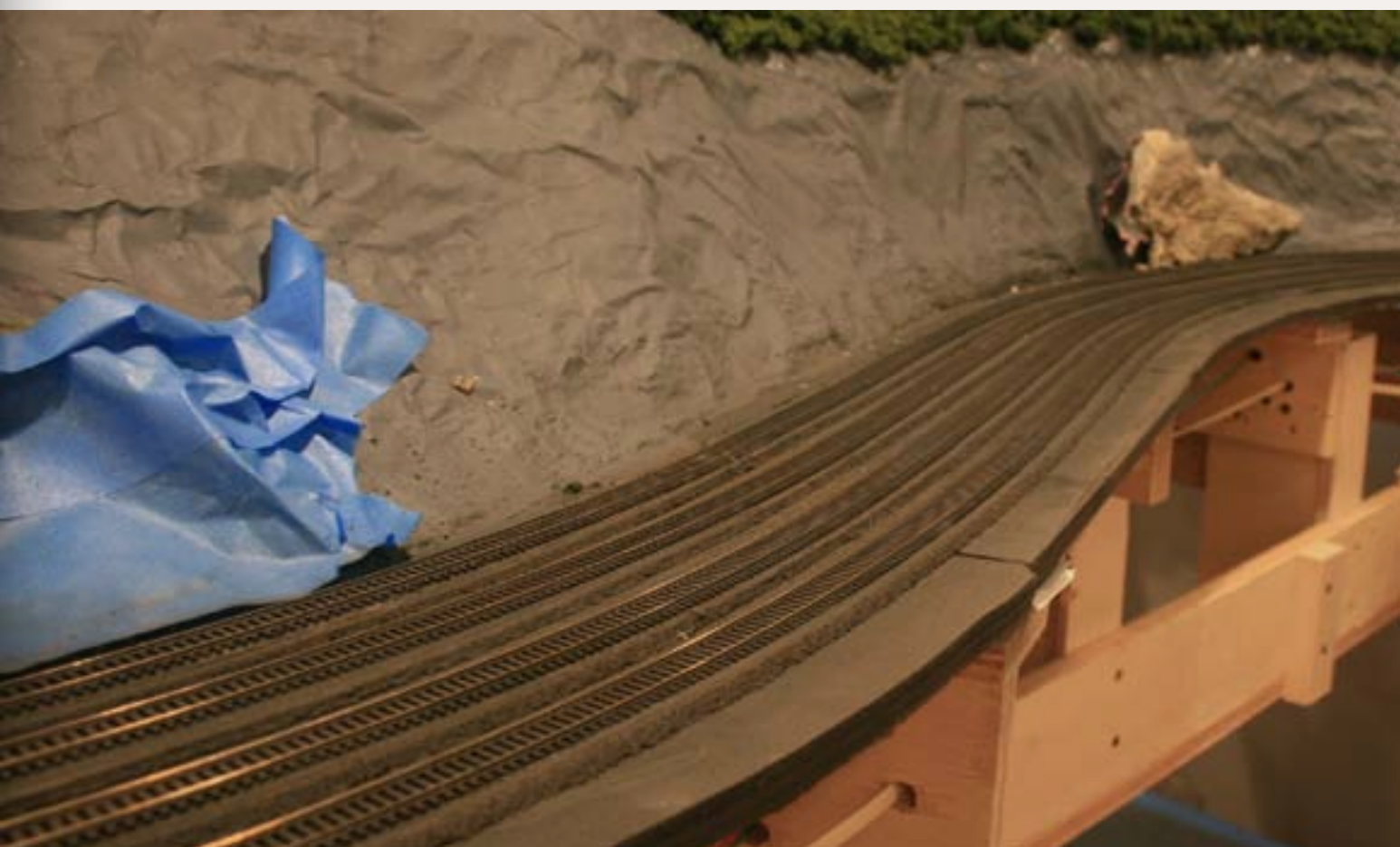
Figure 2: Several light airbrush passes of your favorite “track color” ensures an even, thin, smooth coat.
