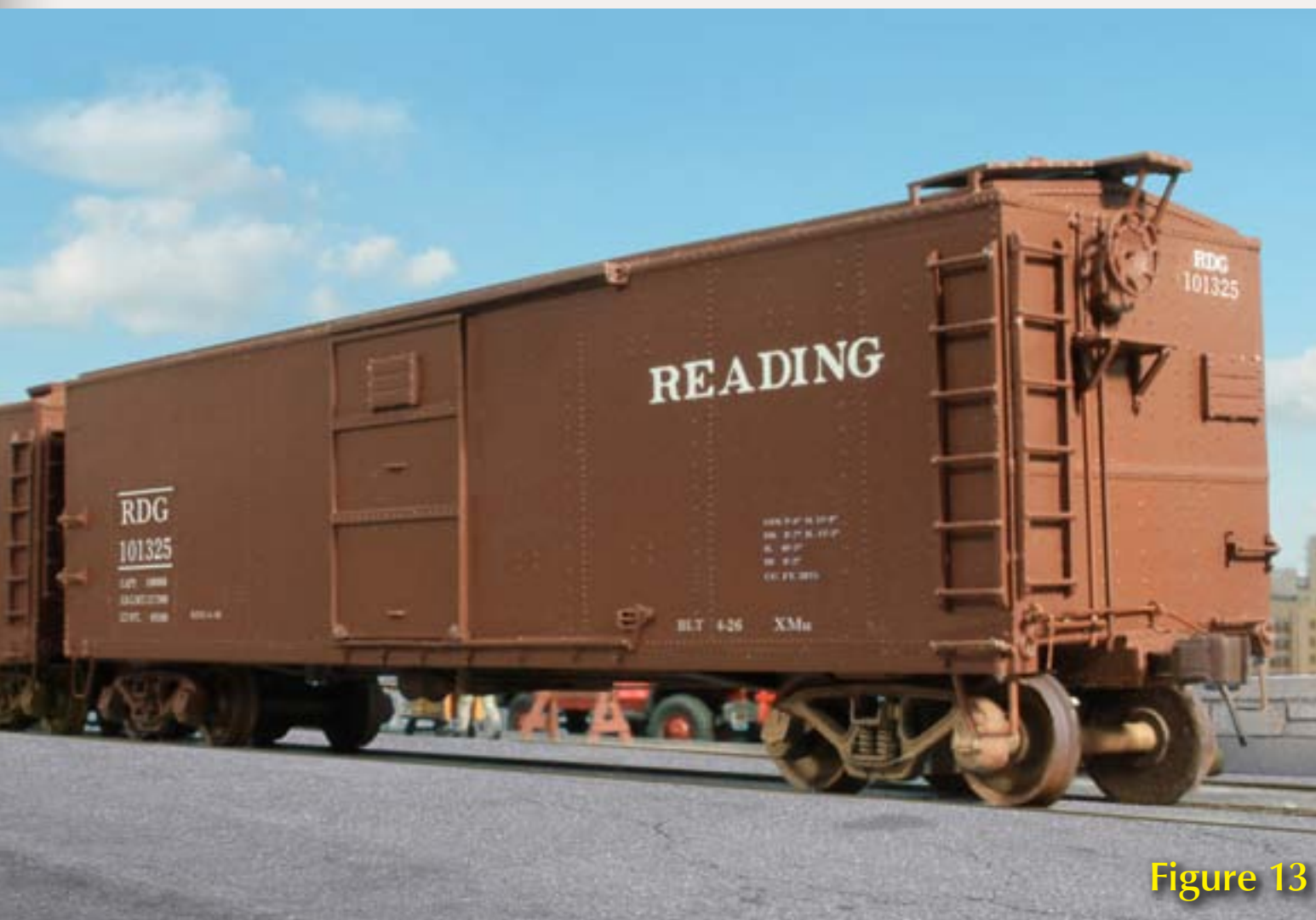
Figure 13: “B” end of Red Caboose Models X29 converted to Reading XMu class boxcar using Archer rivets. The body was made taller using part of a second body.
