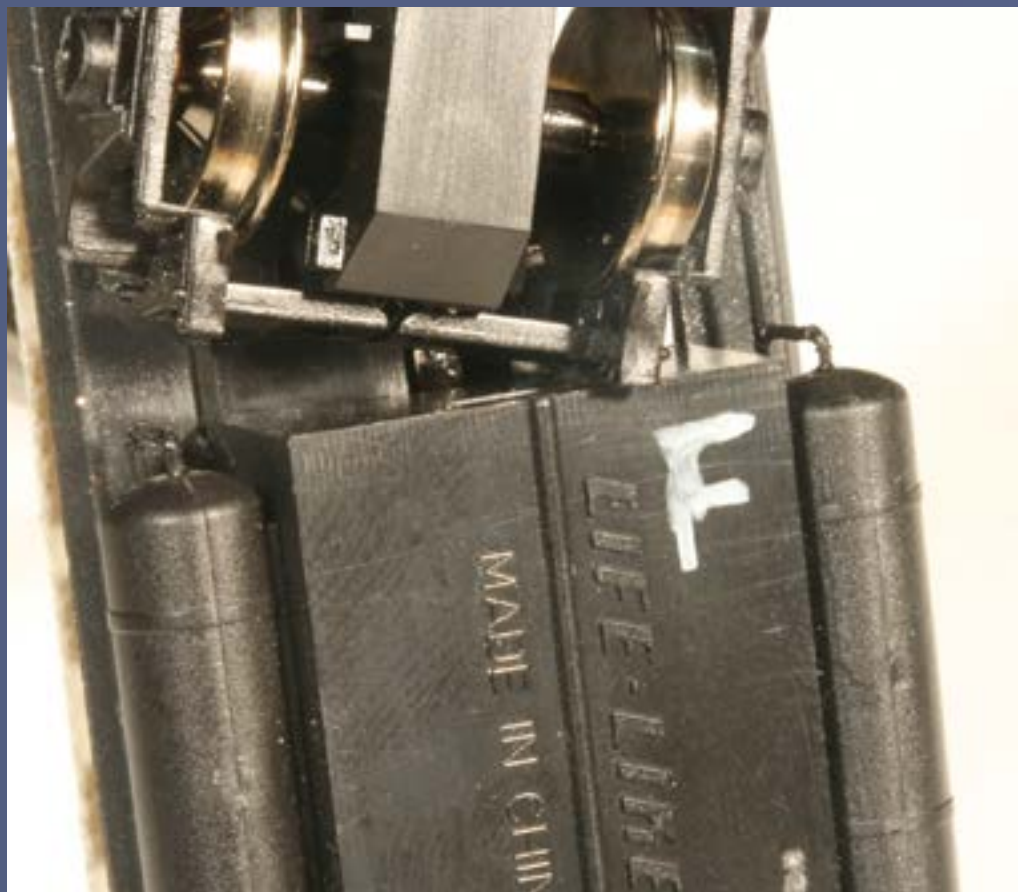
Figure 13: Whenever a model is disassembled, mark each part with the proper orientation (FRONT, REAR, LEFT, RIGHT, etc.) to insure that everything goes back together correctly.
