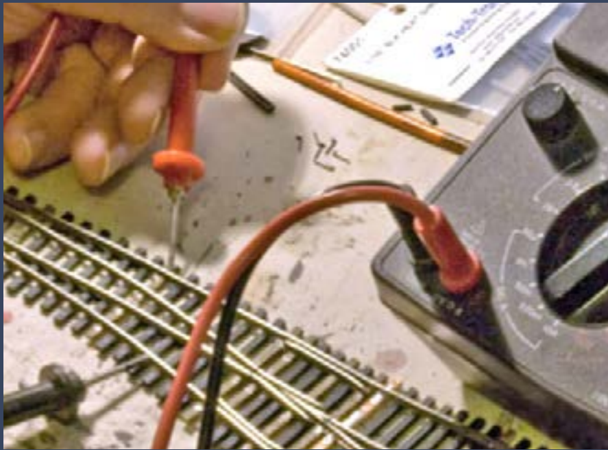
Figure 57: Using a multi-meter, I set it on continuity testing (sounds a tone when there's a connection) and check the turnout for shorts.
