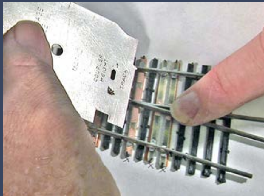
Figure 31: I slide the inner stock rails in/out a bit, using an NMRA track gauge to ensure the track's at minimum gauge through this area, then tack the rails in place with a few spikes.
