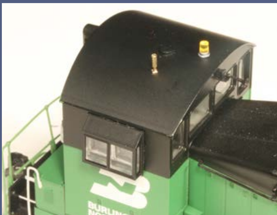
Figure 18: Even adding a few details can make a mass production model look more like a specific prototype. In this case the firecracker antenna and the strobe beacon at the front of the roof are signature details of the Burlington Northern.
