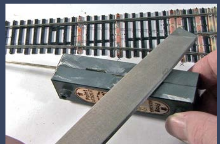
Figure 37: I use the 10" mill file with a #6 Fast Tracks point filing jig to file the point end of the closure rail to a fine taper. Follow the Fast Track guidelines for using this jig to file the point, as shown in the video on their web site ( www.handlaidtrack.com ).
