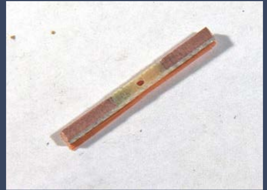
Figure 48: I use the mill file to remove the copper foil from the hole area for about 1/4" in each direction. I also apply a couple layers of masking tape to shim the throwbar.
