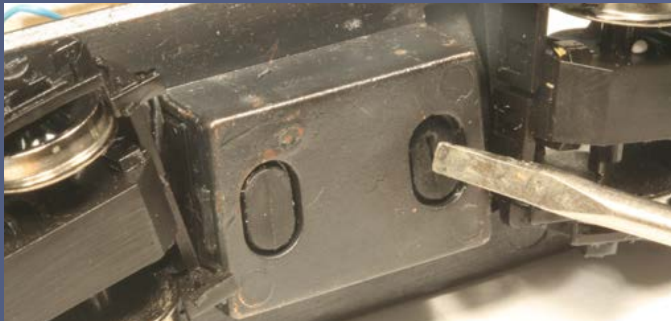
Figure 16: Removing the motor from a model locomotive requires removing any screws holding it in place, then pressing the motor mounts from the frame with a screwdriver.
