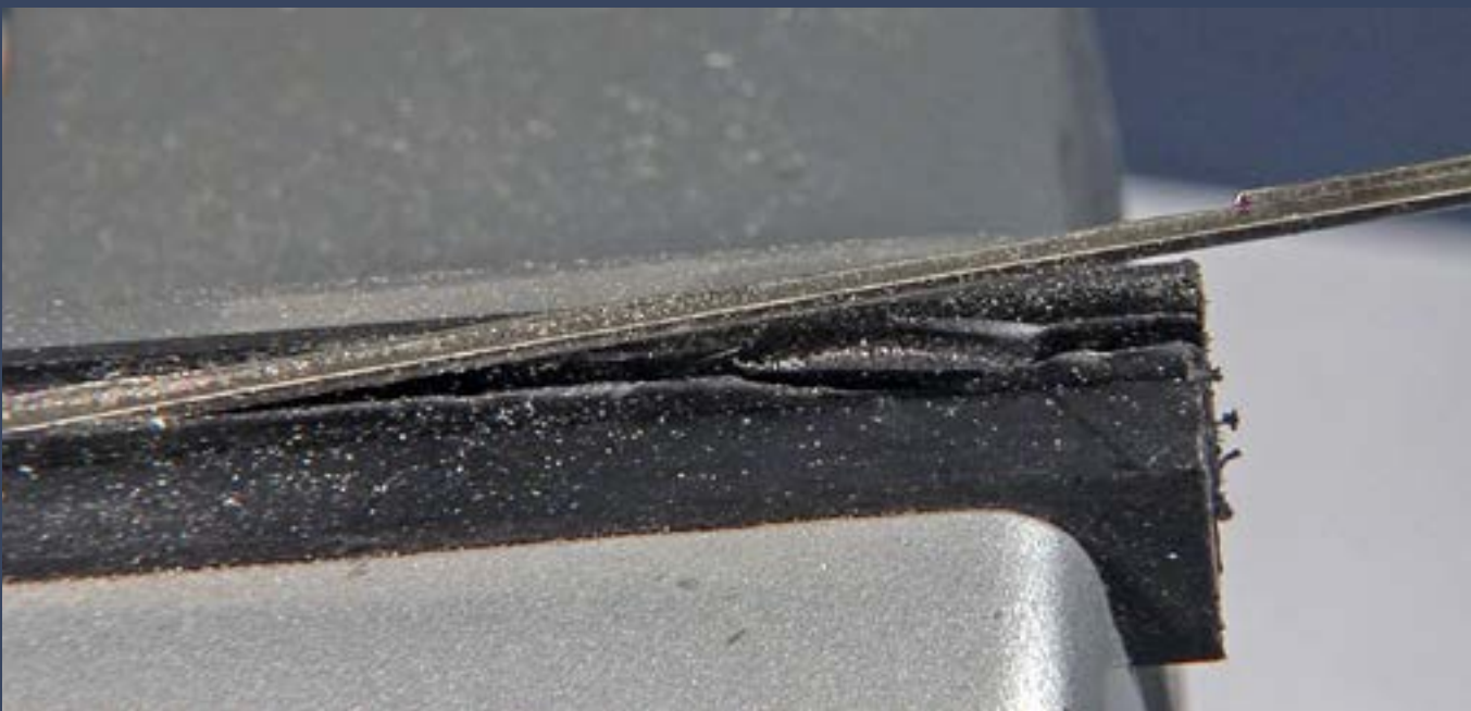
Figure 19: Here's the completed stock rail with a taper filed in the base. Notice I touched only the base of the rail – I did not touch the railhead with the file.
