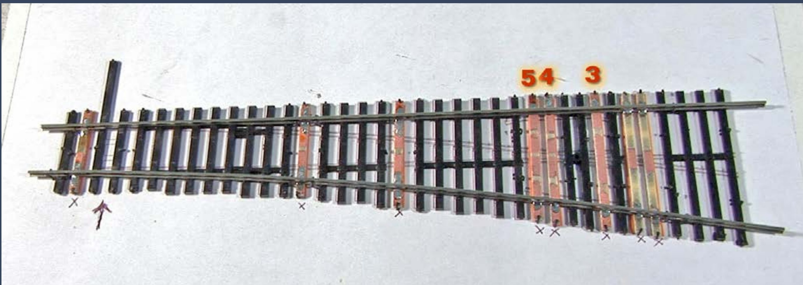
Figure 26: Here's the turnout with the stock rails soldered to all the PC ties. Note that on PC ties 3, 4, and 5, I only soldered the outside of the rails because the inside of the rails will be where I solder the guard rails. I don't want any solder interfering with the proper placement of the guard rails.
