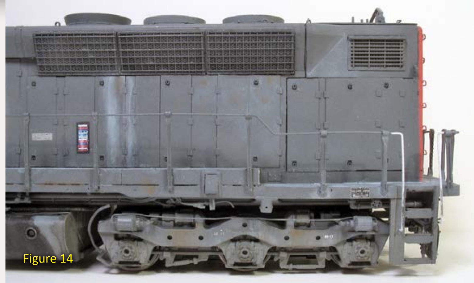
Figure 13 and 14: Elizabeth scratchbuilt the hood of her SDP45 using Evergreen styrene and Cannon doors. Other details include radiator grilles salvaged from a Proto 2000 SD45, and Precision Investment Associates (PIA) handrail stanchions (Figures 2, 8, 13, and 15).
