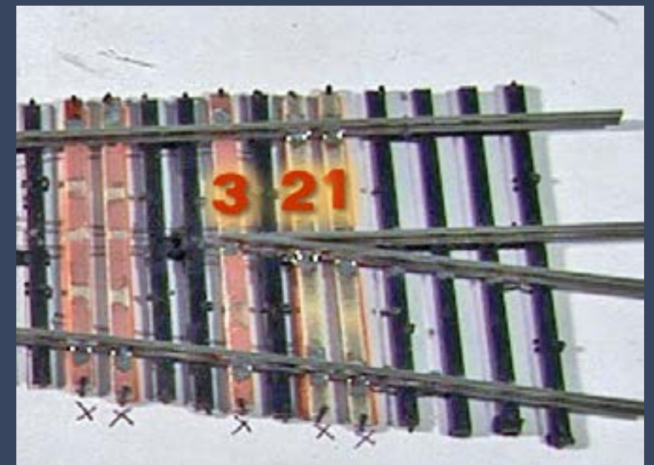
Figure 32: I solder the inner stock rails to PC ties 1 and 2 on the sides of the rails I can reach. I apply minimal solder to PC tie 3 to avoid issues later with the frog wing rails.
