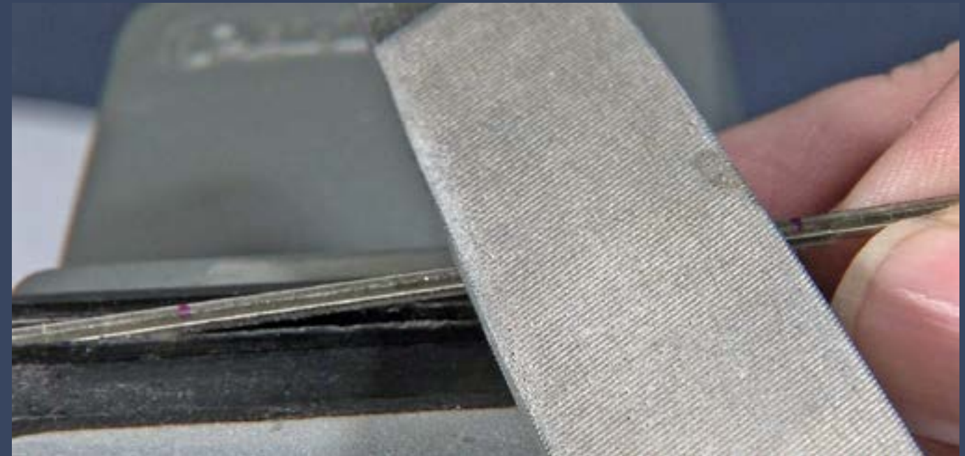
Figure 18: I put the rail in a vise and use a 10" mill file to carefully file away just the base of the rail over the distance between the two marks. I slant the file slightly to avoid touching the railhead with the file.
