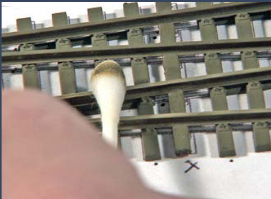
Figure 63: Once the glue is set, I remove all the spikes and take the turnout outside and spray paint it with a spray can of Floquil Rail Brown. I use Q-tips dipped in lacquer thinner to clean the rail heads.
