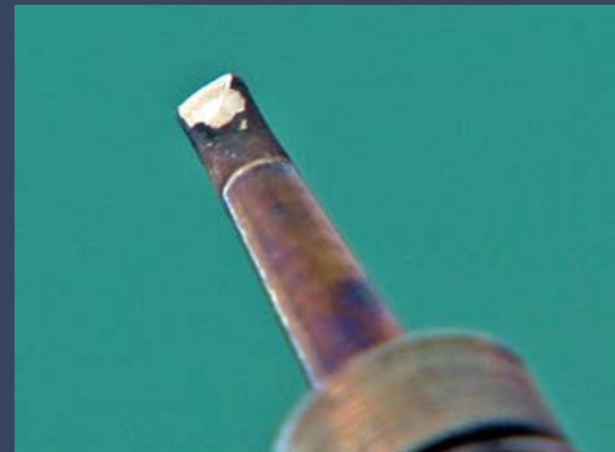
Figure 23: Once properly cleaned and tinned, the tip is shiny like this.
