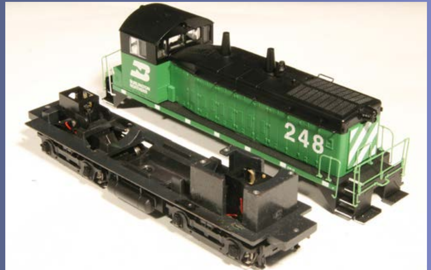
Figure 17: With the locomotive's drivetrain fully removed, we now have an unpowered chassis that the shell can be mounted onto.
