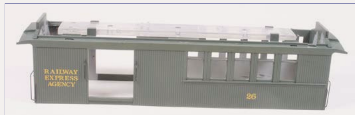
Figure 9: The light bar attaches across the top of the body shell and is held in place with plastic ears. Filing the tabs lower on the ears makes disassembly of the parts easier for repair. Grabirons and handrails have been applied to the body shell.
