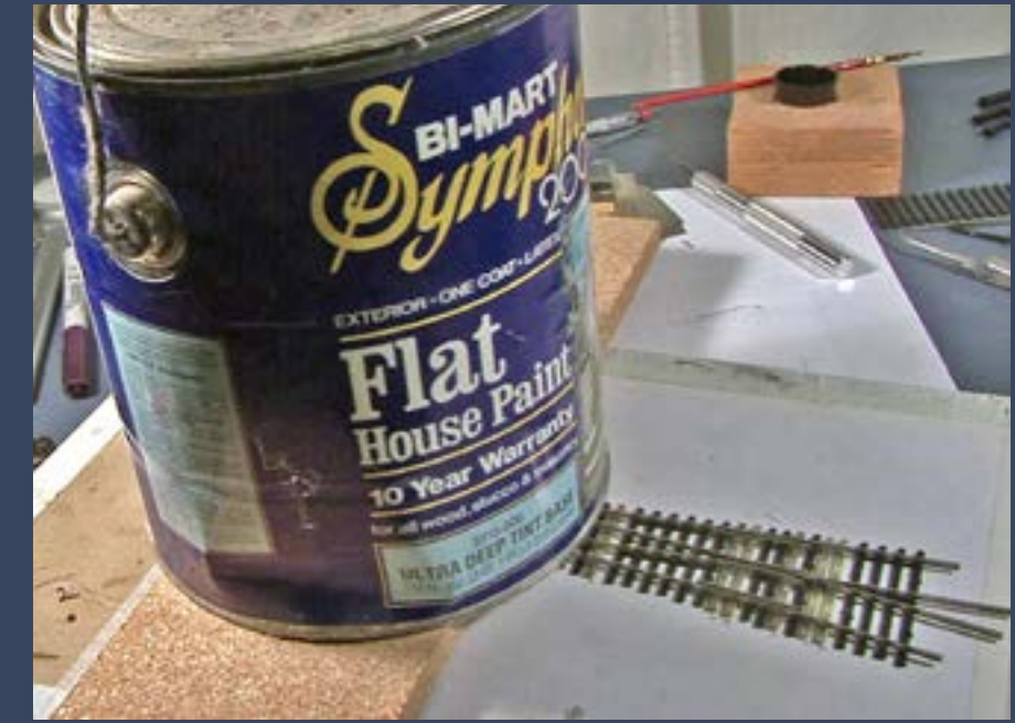
Figure 62: The point end of the turnout didn't stay perfectly seated in the tie slots, so I used a scrap of particle board and a full paint can as a weight and let it sit for an hour.
