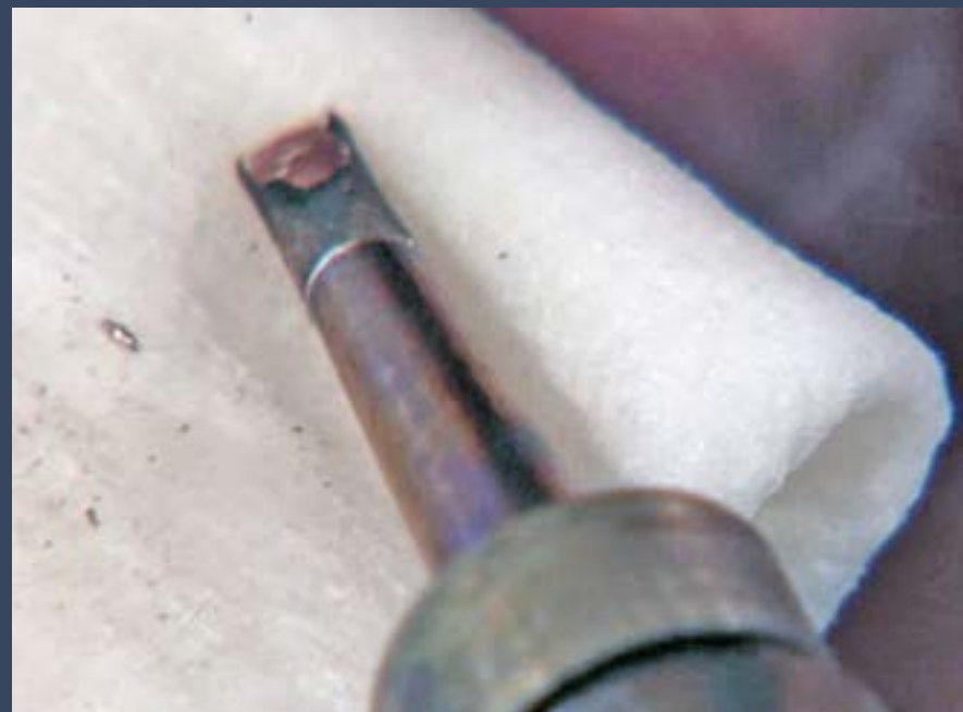
Figure 22: I heat the iron, apply a bit of rosin-core solder to "tin" the tip, and then wipe the tip on a damp paper towel.
