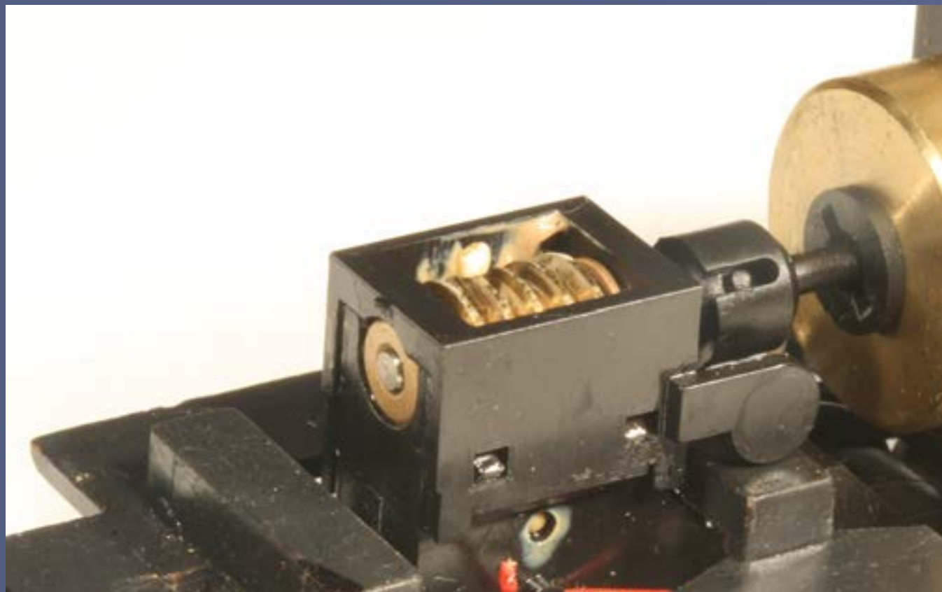
Figure 9: A driveshaft turns a worm gear at the top of the gear tower of the truck. The worm gear then turns gears inside the truck causing the wheels to turn.
