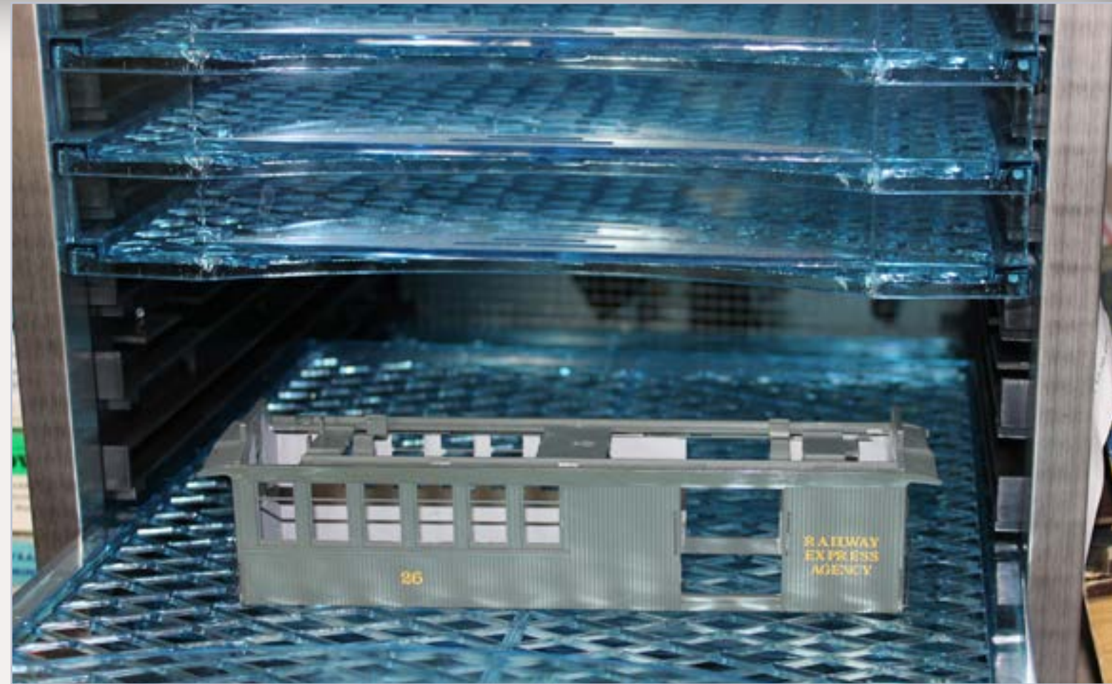
Figure 7: Food dryers with adjustable heat and circulating fans make excellent paint dryers. One hour in the machine is equivalent to about 12 hours of open air drying.
