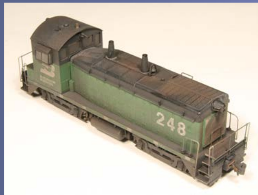
Figure 18: Even adding a few details can make a mass production model look more like a specific prototype. In this case the firecracker antenna and the strobe beacon at the front of the roof are signature details of the Burlington Northern.
