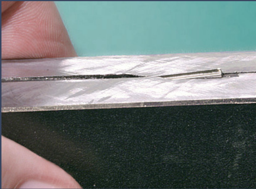
Figure 27: Using a 10" mill file on #6 frog point filing jig from Fast Tracks, I file the frog point on each of the two inner stock rails.
