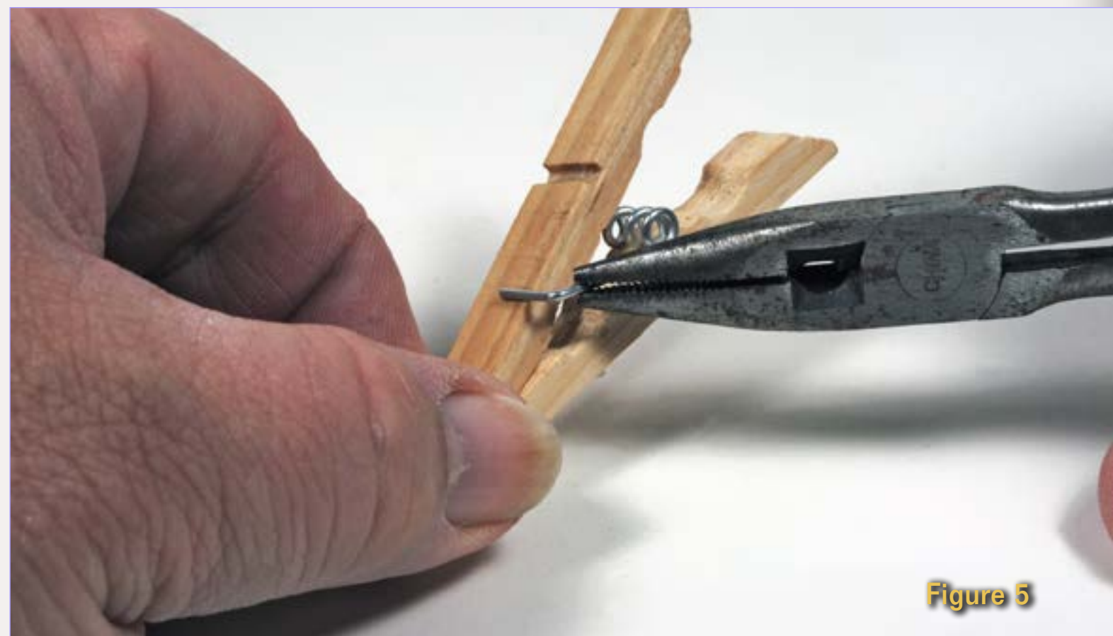
Figure 4: Grasp the spring firmly and reverse it end for end so that the coil now faces the heavy end and the wire pins face the thin, former handles that will be the jaws of the clamp.
