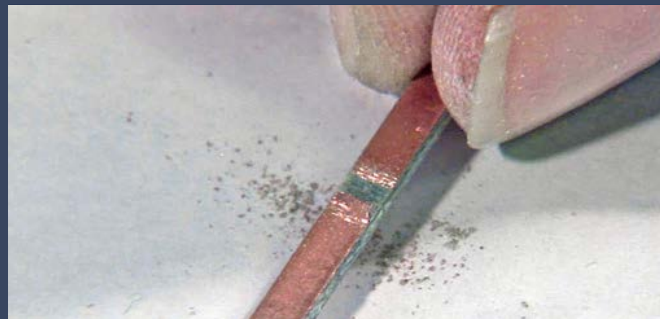
Figure 14: In order to prevent shorts, I file a gap in the copper foil on the PC ties. For the first two ties past the points, I only filed one gap, to allow the turnout closure rails and stock rails to be the same polarity. Around the frog I file two gaps - one in each route.
