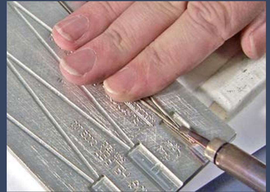
Figure 29: A quick touch to the fluxed area with a hot soldering iron tip pre-loaded with a little solder and the solder flows onto the rails and makes them a solid unit.
