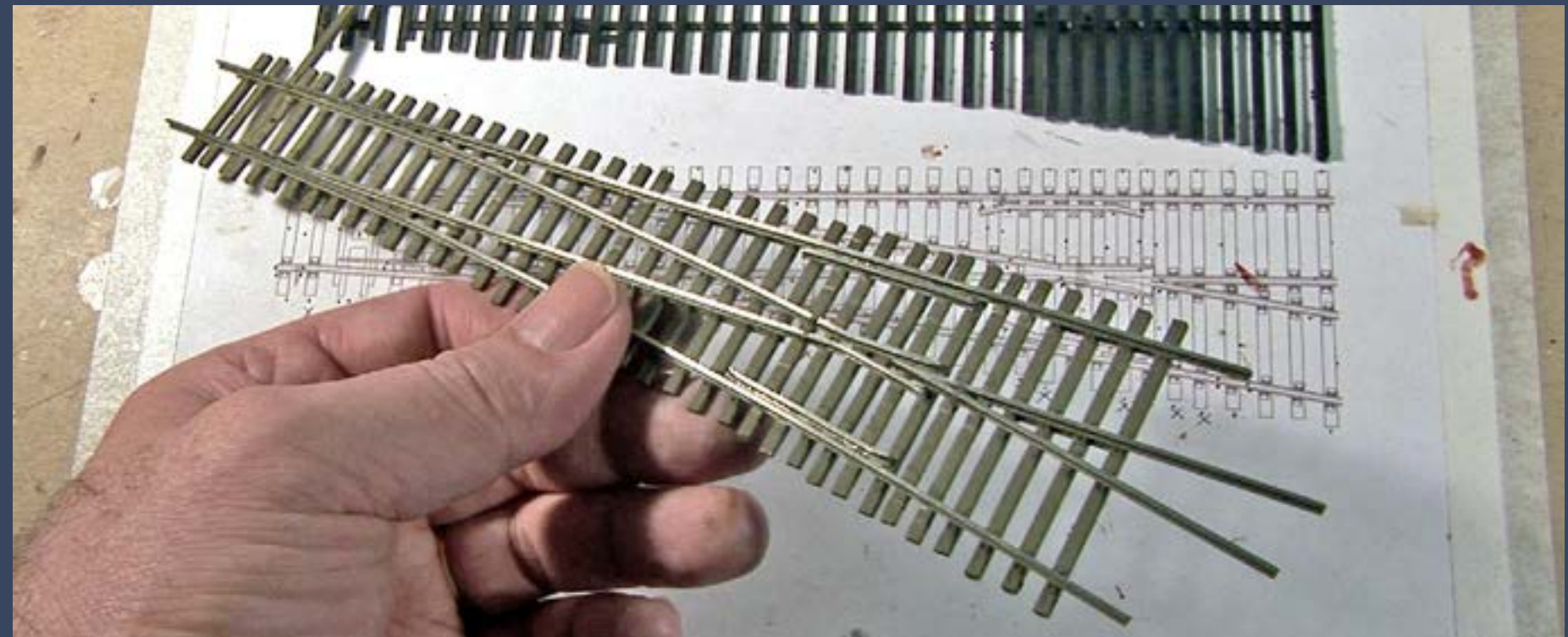
Figure 64: So here's my finished, completely in-spec turnout, ready to install. You can do more to superdetail a turnout, but we'll leave that for a future article.
