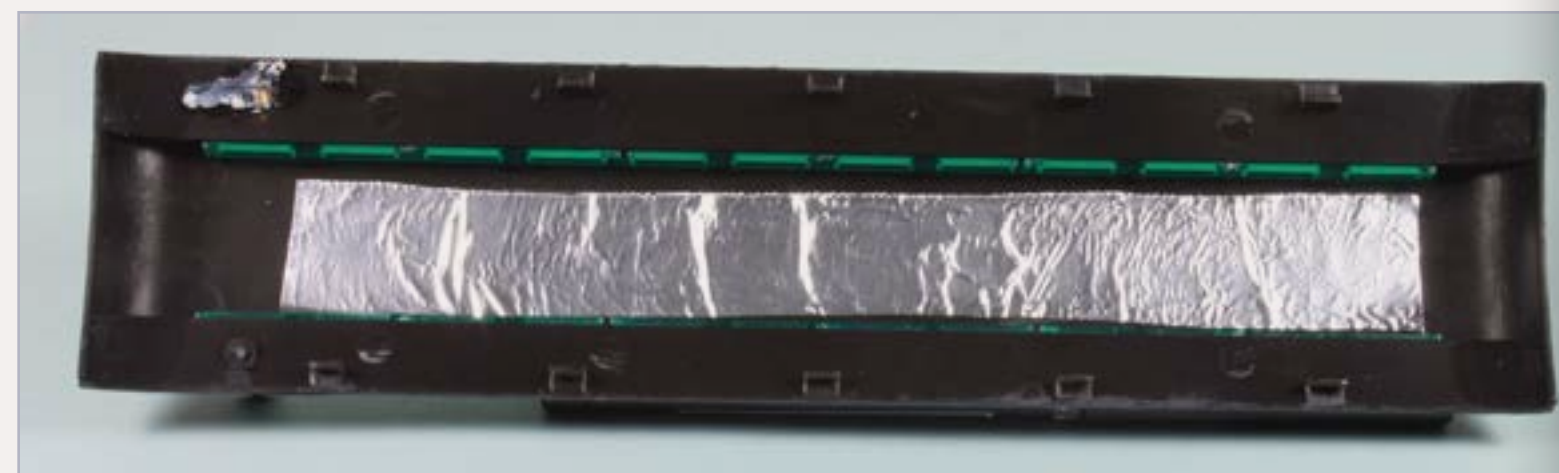
Figure 13: A roof reflector helps even-out the illumination. Apply a piece of double sticky tape to aluminum foil, trim with a scissors and attach the foil inside the roof.
