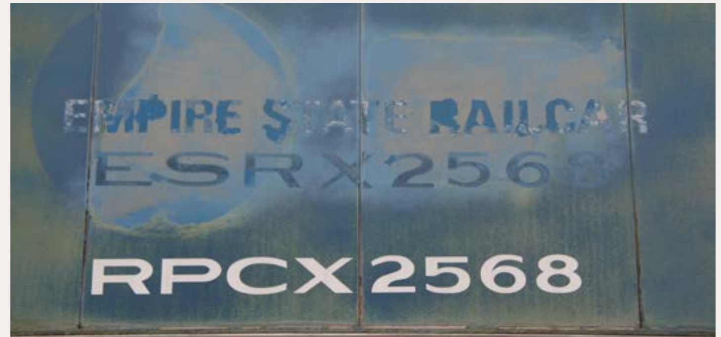
Figure 2: The reporting marks of this railcar are an example of equipment that remains in an older livery with new reporting marks making it AAR compliant.
