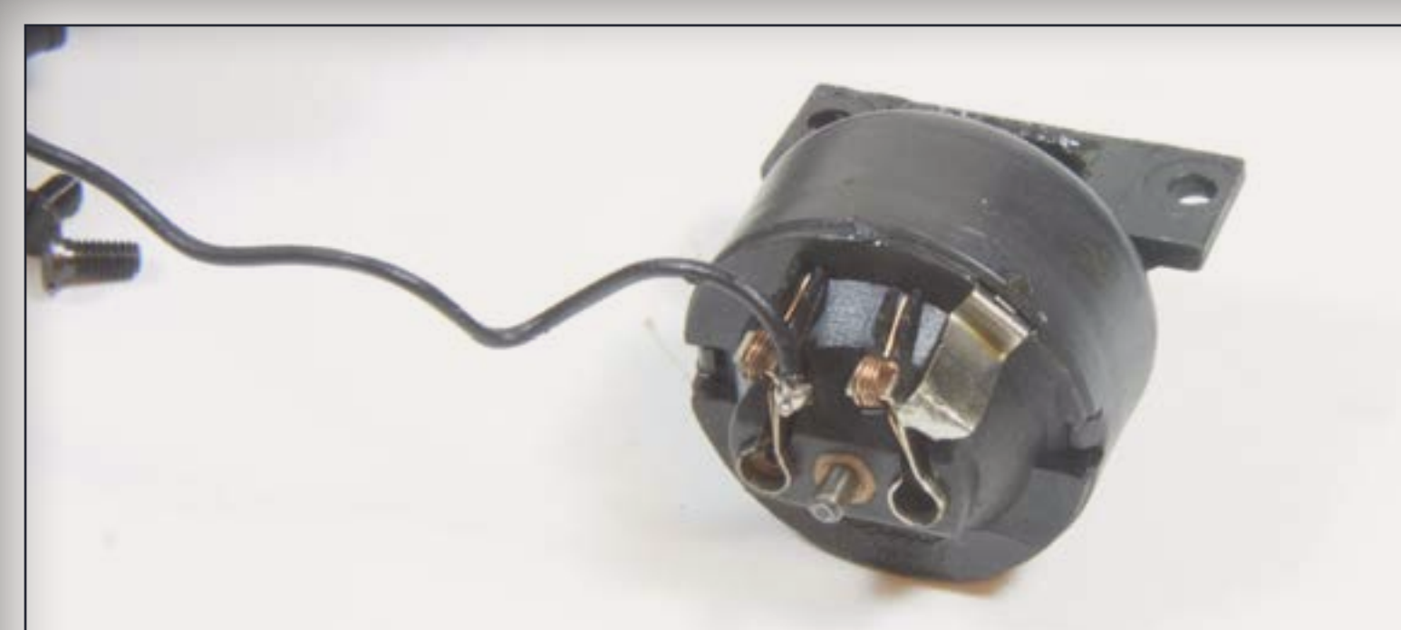
Figure 4: This is what the Heisler motor looks like out of the HO model. The wire on the left is the connection to the right rail and the silver tab is the jumper from the left rail, grounded from the chassis to the motor. When the tab is cut, the motor will be isolated from the chassis. Always use a meter to confirm that the motor is electrically isolated from the body and chassis.
