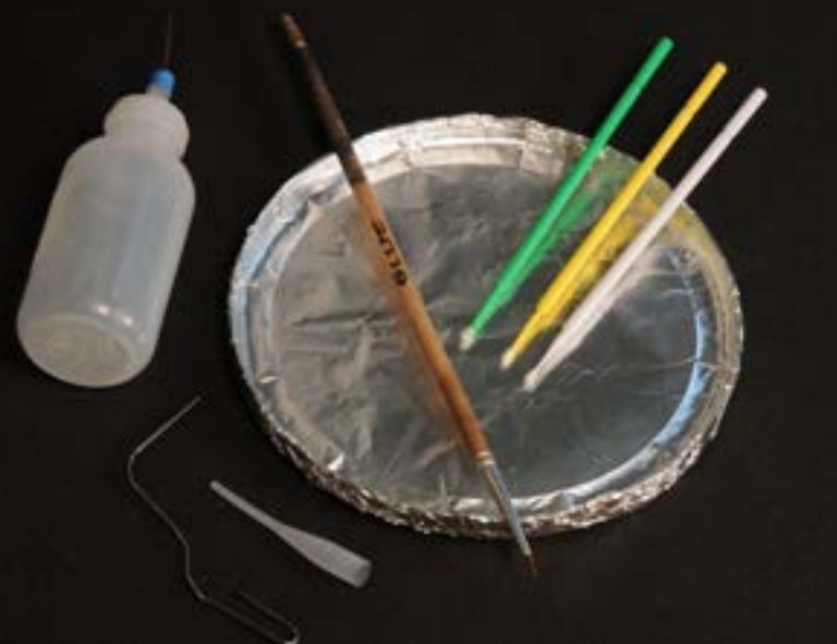
Figure 3: Solvent applicators – using the right tool is critical with solvents. Aluminum foil on a plastic container lid makes a good palette. Fine paint brushes or Microbrushes can apply small amounts of cement. So can bits of wire, straightened paperclips and plastic bottles with needle-fine applicators. Thin Delrin tips can control the liquids' flow.
