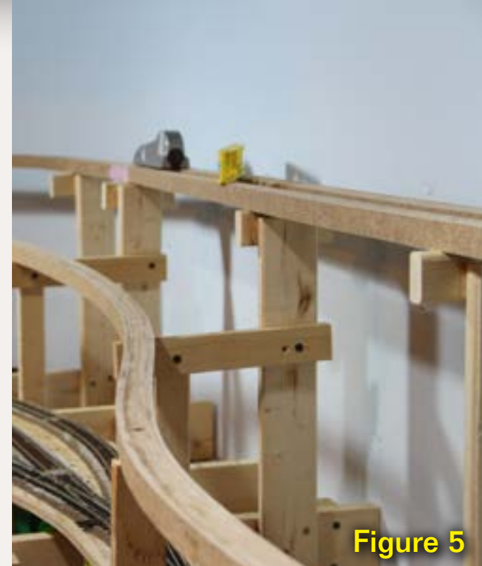
Figure 5: Spline roadbed is made by laminating individual vertical splines, in this case 1" strips of 1/4" Masonite. It lends itself to making graceful curves and is nearly indestructible once the glue cures.
