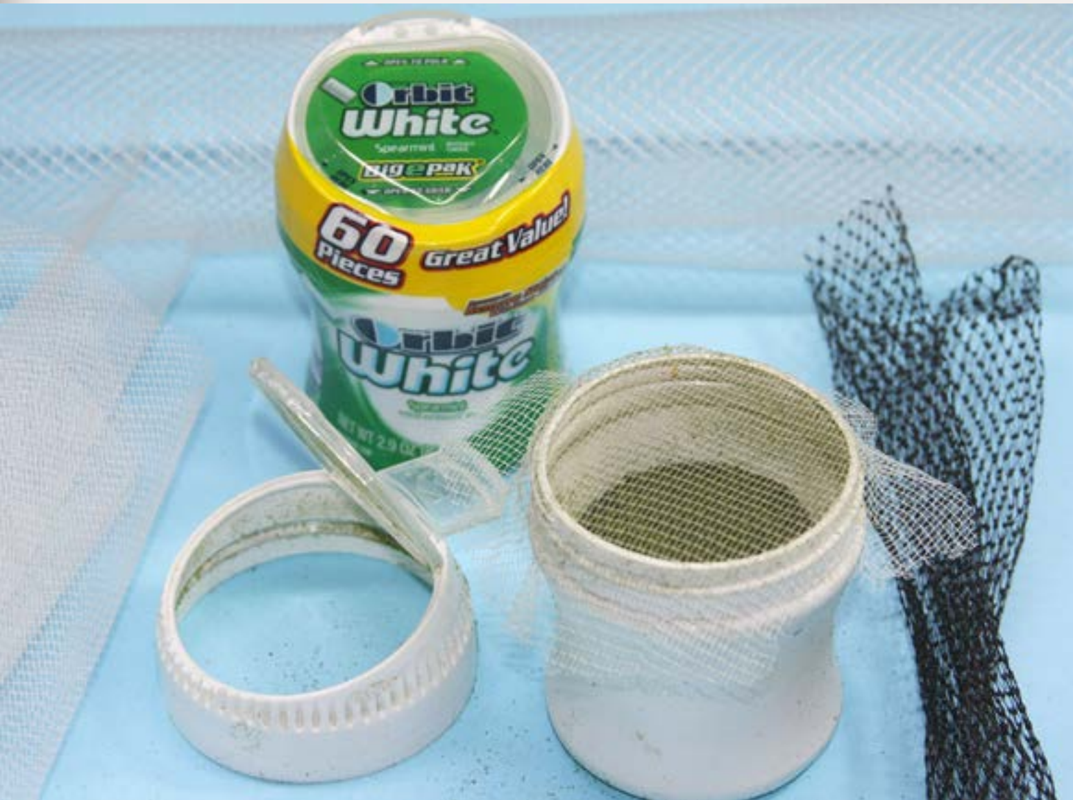
Figures 4 and 5: Inexpensive shakers for applying scenic materials made from plastic screening and containers that originally held gum.
