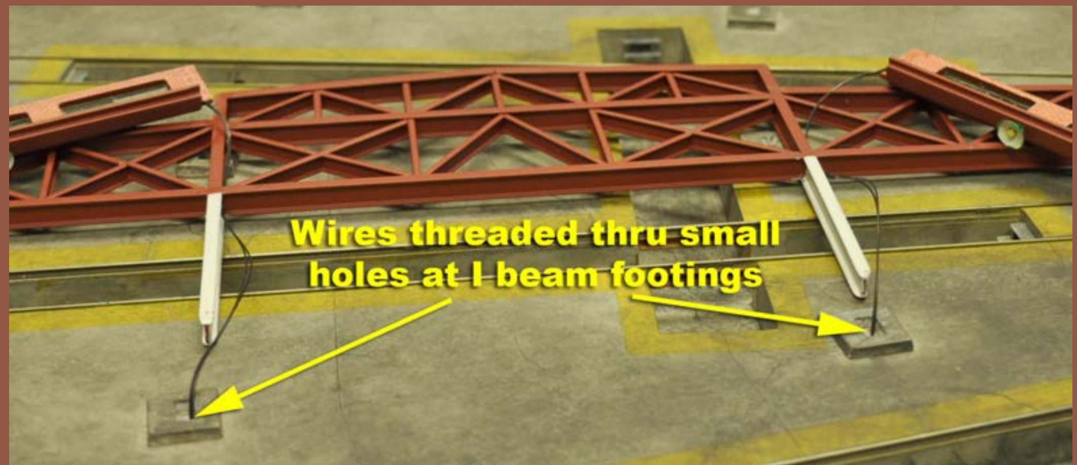
Figure 5: I drilled holes in the footings in the roundhouse floor where the I beams will be inserted.
