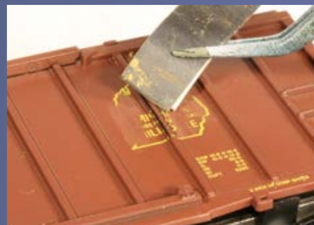
Figure 31: Thin sandpaper can become very rigid and allow excellent control when it is cut into thin strips and folded over upon itself.
