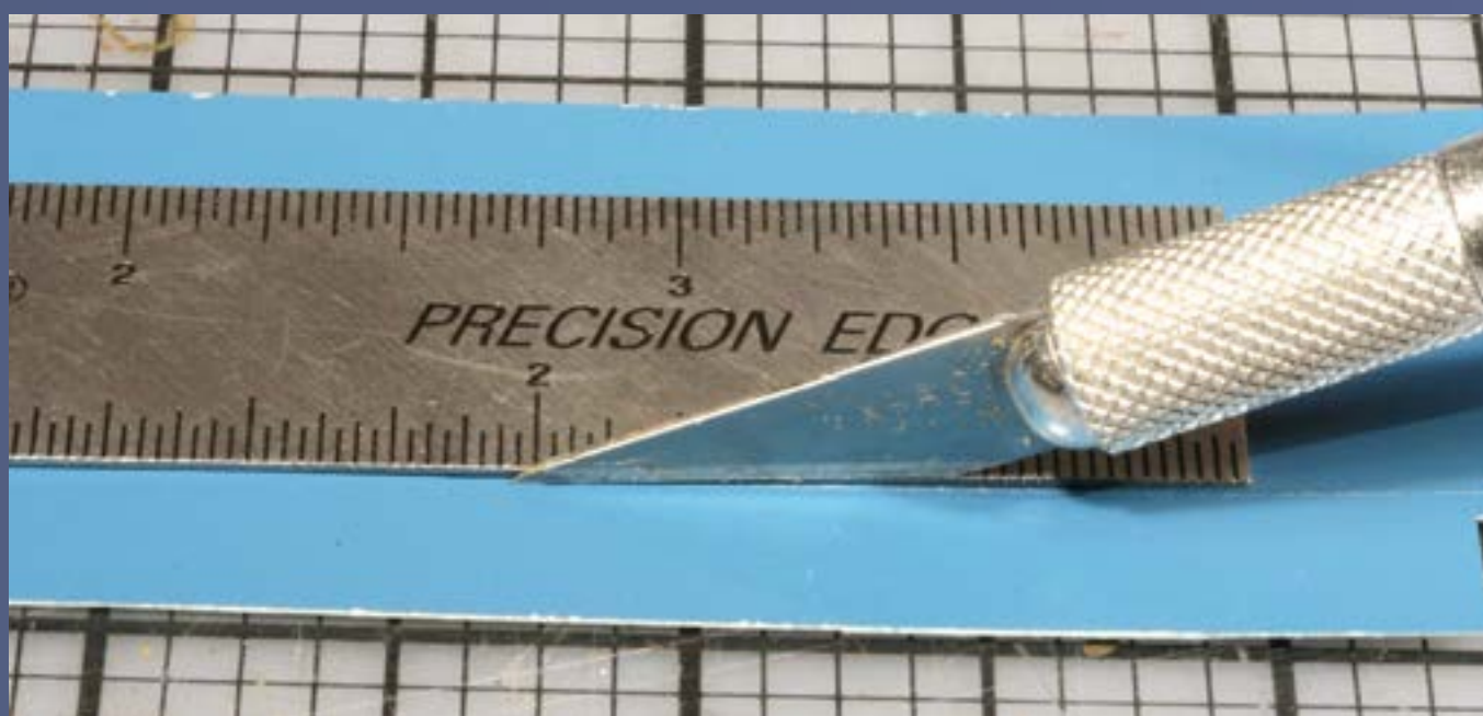
Figure 38: Placing the knife blade flat along the surface of the film will help to prevent chipping along the cut edge.
