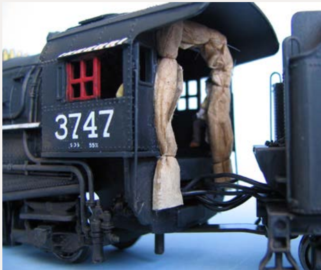
Figure 6: The rolled and tied off cab curtain is ready to install in your locomotive. The ends will be trimmed in place after installation.
