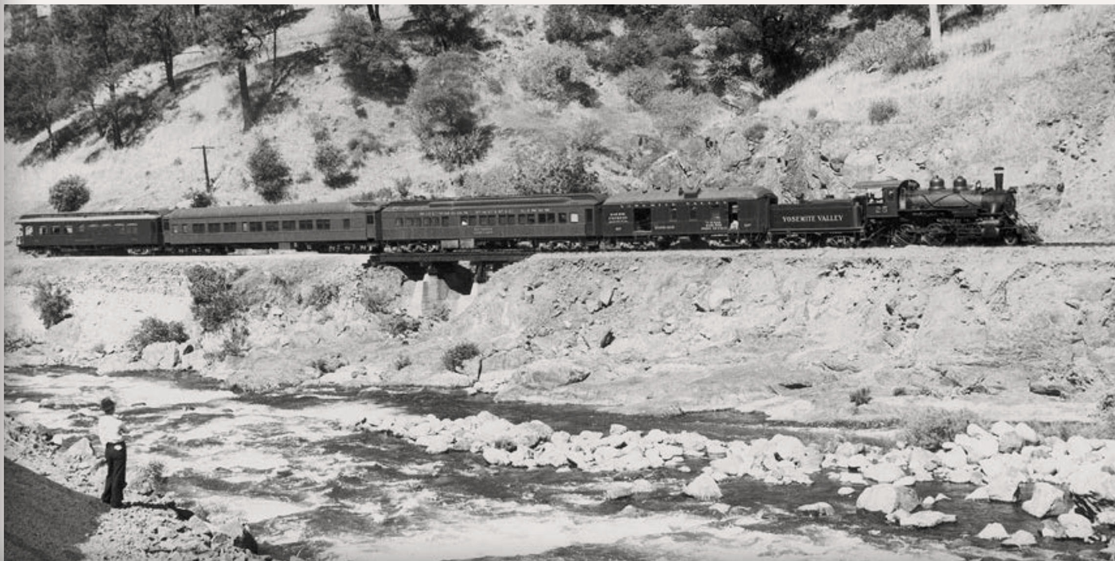
Figure 2: Will Whittaker took this photo of a YV passenger train in July 1941. The train includes a YV steel 40-ft. RPO car, a heavyweight Pullman, a rented SP diner, and the YV's classic observation car on the end. Vegetation along the Merced River has not yet returned after the disastrous 1937 flood. Pullmans were operated only between Memorial Day and Labor Day, which was another factor in my decision to model August.
