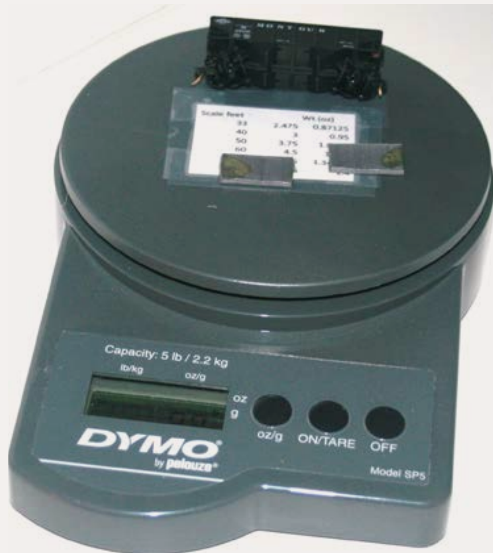
Figure 2: An inexpensive postal scale is excellent for measuring car weight. This one has the NMRA standards taped to the top for easy reference. Added weight in the form of sheet lead is weighed along with the car prior to installation.
