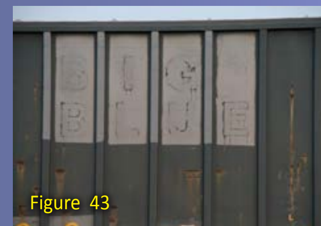
Figures 42-43: An interesting effect can be created by placing trim film directly over factory printing that has not been made smooth with the paint surface. The relief of the raised printing will show through the trim film, leaving a ghost effect such as the 'BIG BLUE' showing through on this ex-CSX boxcar.
