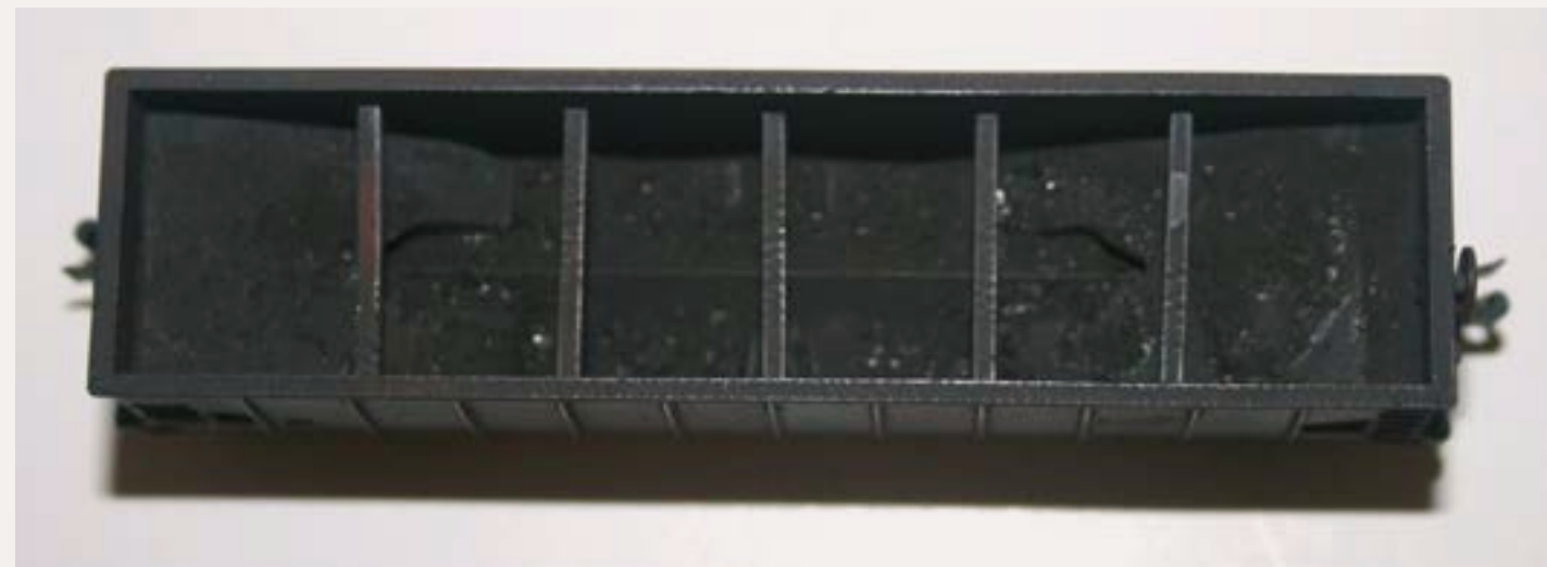
Figure 5: Here is a top view of the cross-bracing on PRR's 4-bay hoppers. The figure also shows how weathering and a bit of coal can disguise the sheet lead weights below the bracing.
