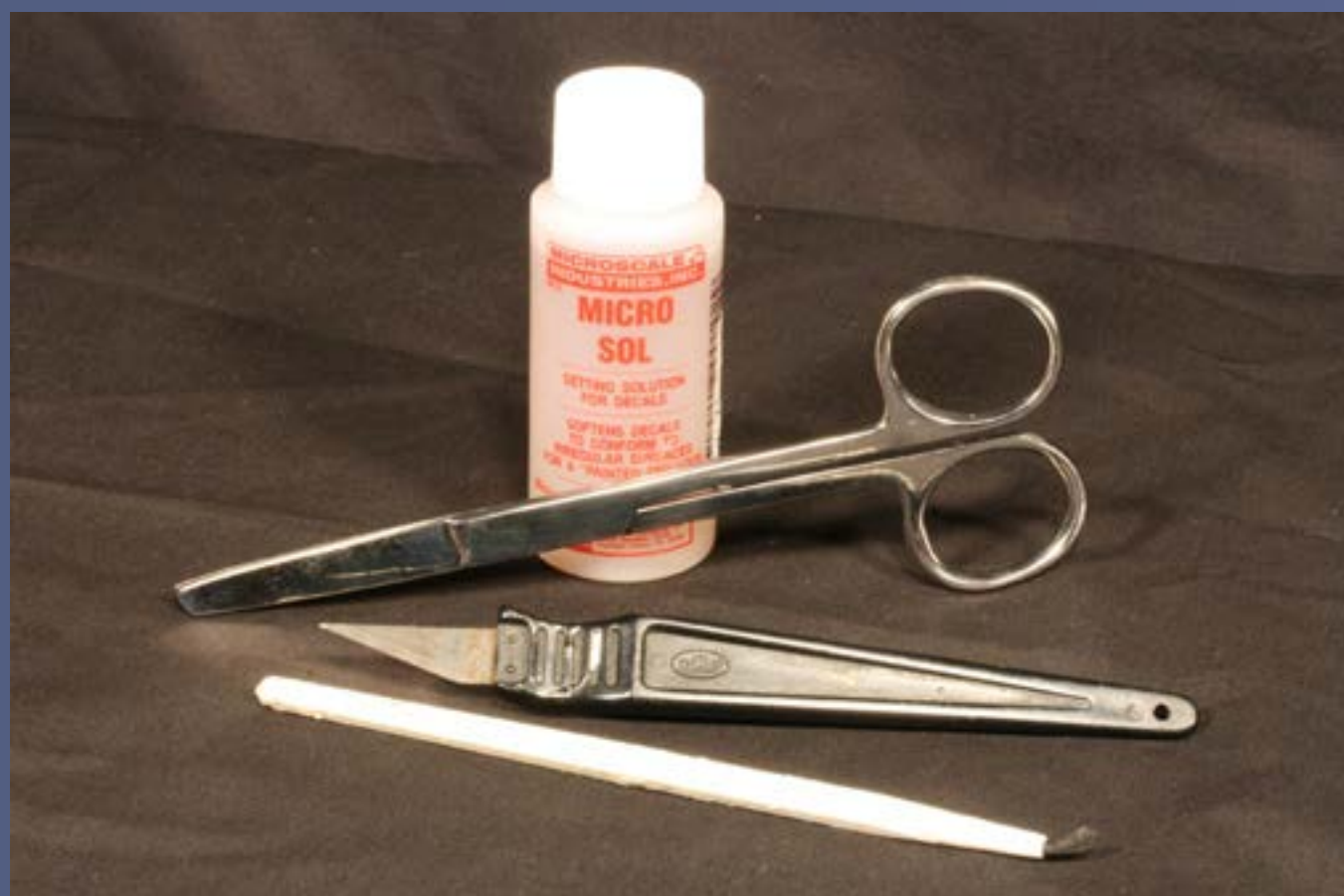
Figure 41: Four tools required for any successful decal application are sharp scissors, a dull hobby knife to position the decal, a decal setting solution to allow the decal to conform to imperfections in the surface, and a small brush to apply the setting solution.
