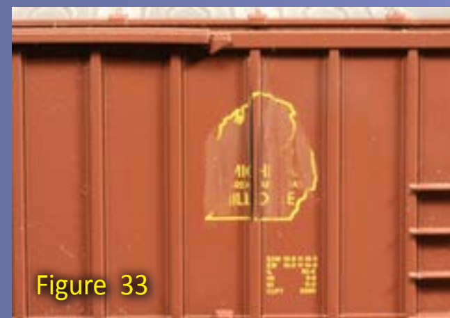
Figures 32-33: Varying the amount of distress of the car's graphics can create the look of aged, faded, or flaking paint.
