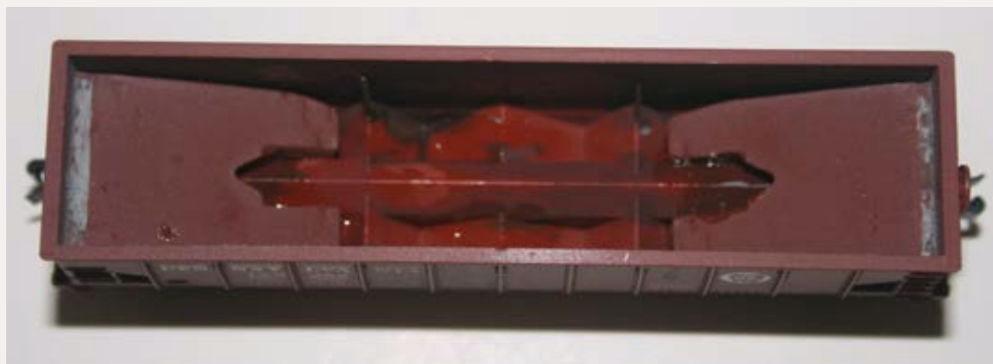
Figure 4: Sheet lead fitted to the bottom of a hopper. This 4-bay hopper 'borrows' the weight from a Bowser 2-bay, but sheet lead can be cut to fit any car.
