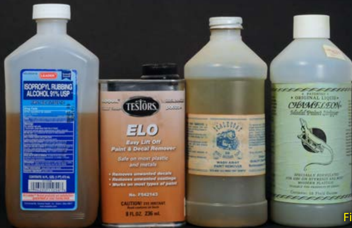
Figure 3: A variety of paint strippers. From left to right: 91% isopropyl alcohol, Testors Easy Lift Off, ScaleCoat Wash Away, and Chameleon Model Paint Stripper.
