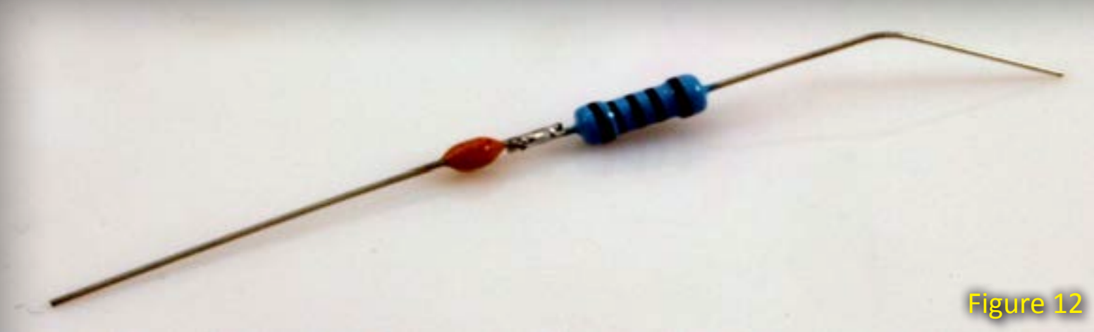
Figure 12: A snubber made from a 100 ohm 1/2 watt resistor and a 0.1 µF 50 volt or higher capacitor.
