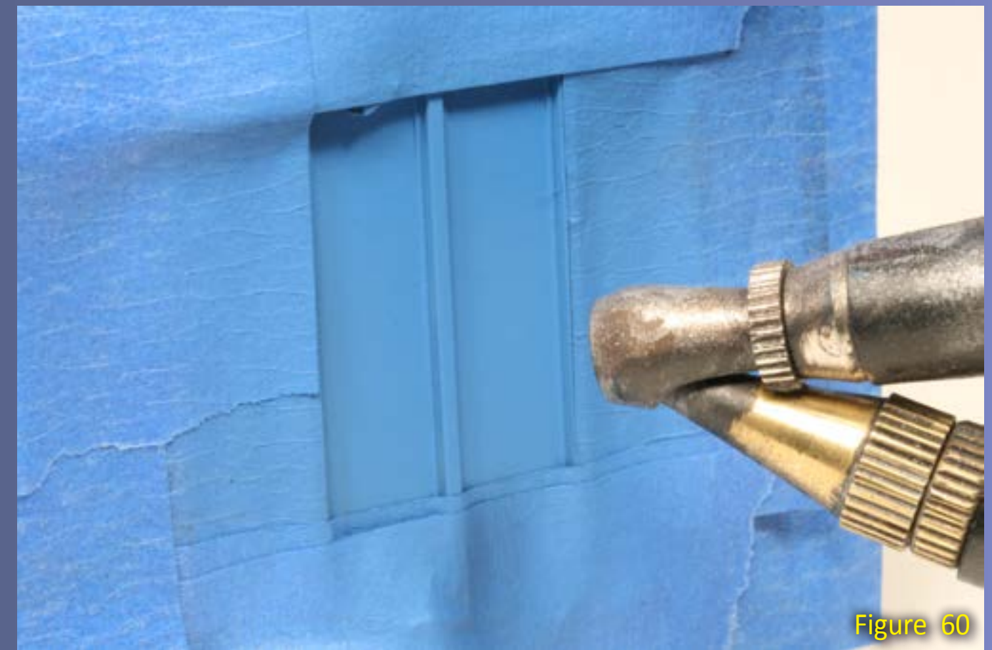
Figures 60: Applying patch paint in thin coats with an airbrush will insure that the patch paint is applied evenly and does not bleed under the masking.
