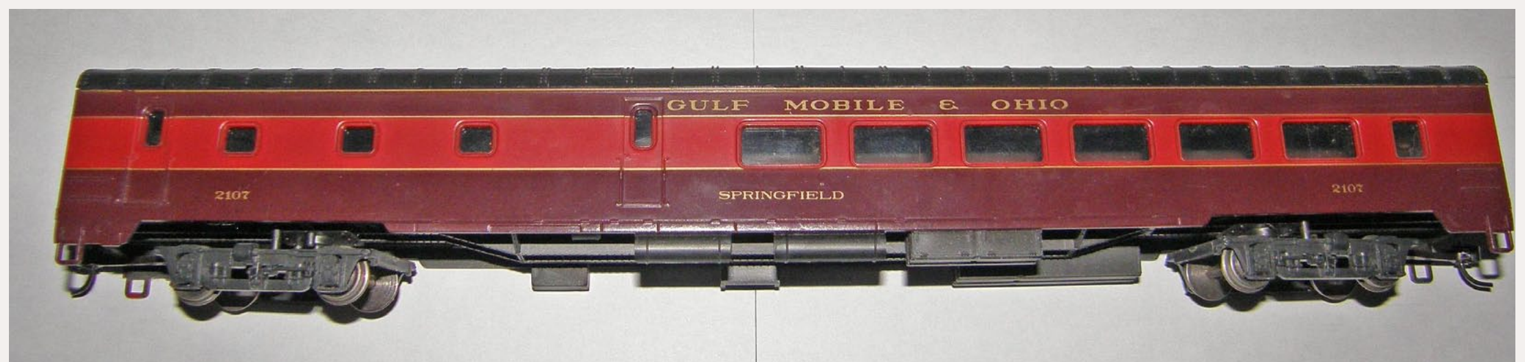
Figure 1: Here is a "before" view of the Rivarossi diner which we are converting to become an ACF parlor car with six-wheel trucks.
