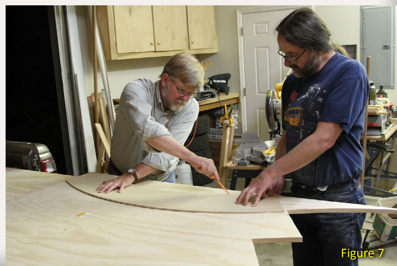
Figure 7: Marking helix segments using the template is a lot less work than swinging a trammel for each piece.
