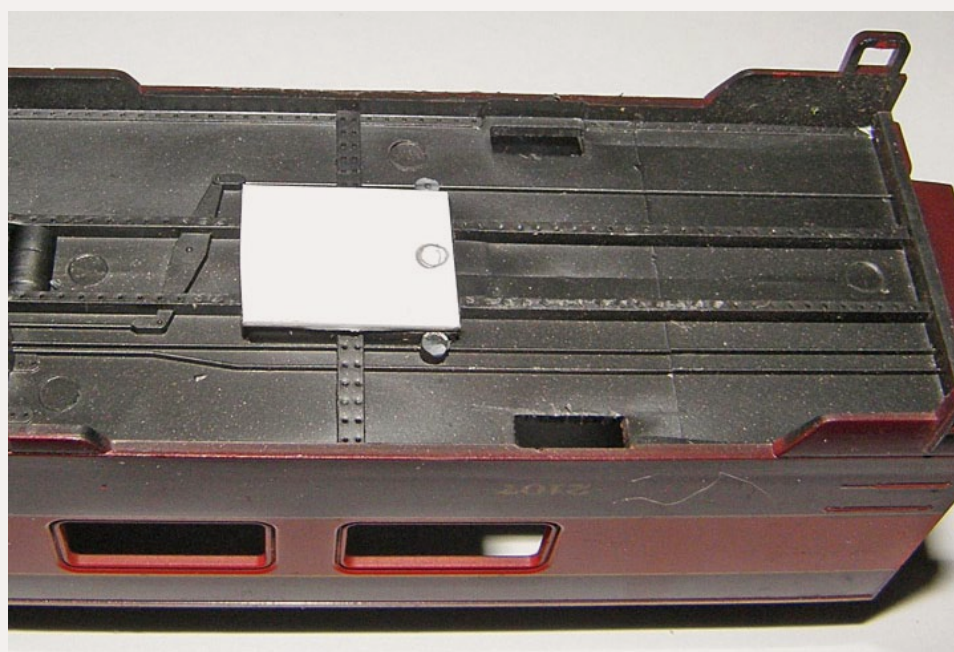
Figure 9: The bolster pad with the pencil-marked location of the new bolster pin hole.
