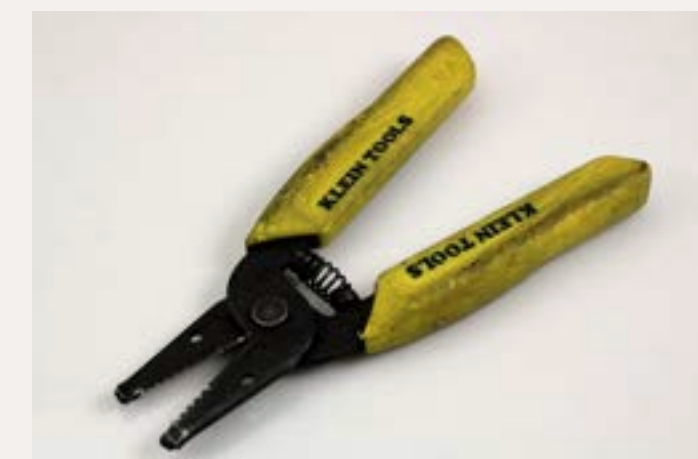
Figure 1: My dirty, old wire strippers are Klein Tools #11047 – specifically designed for 22 AWG to 30 AWG wire.
