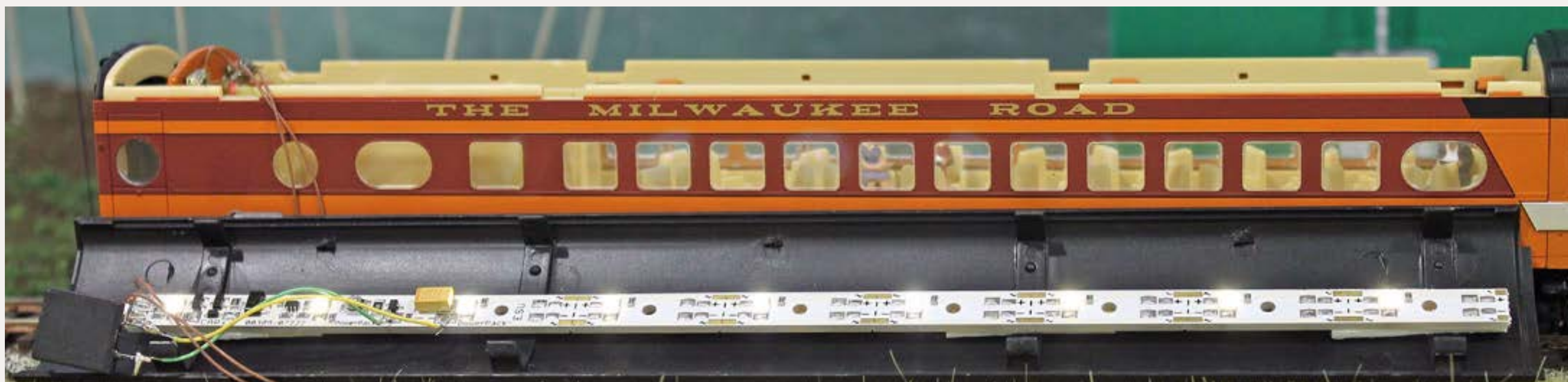
Figure 4: Lighting strip installed and illuminated.
