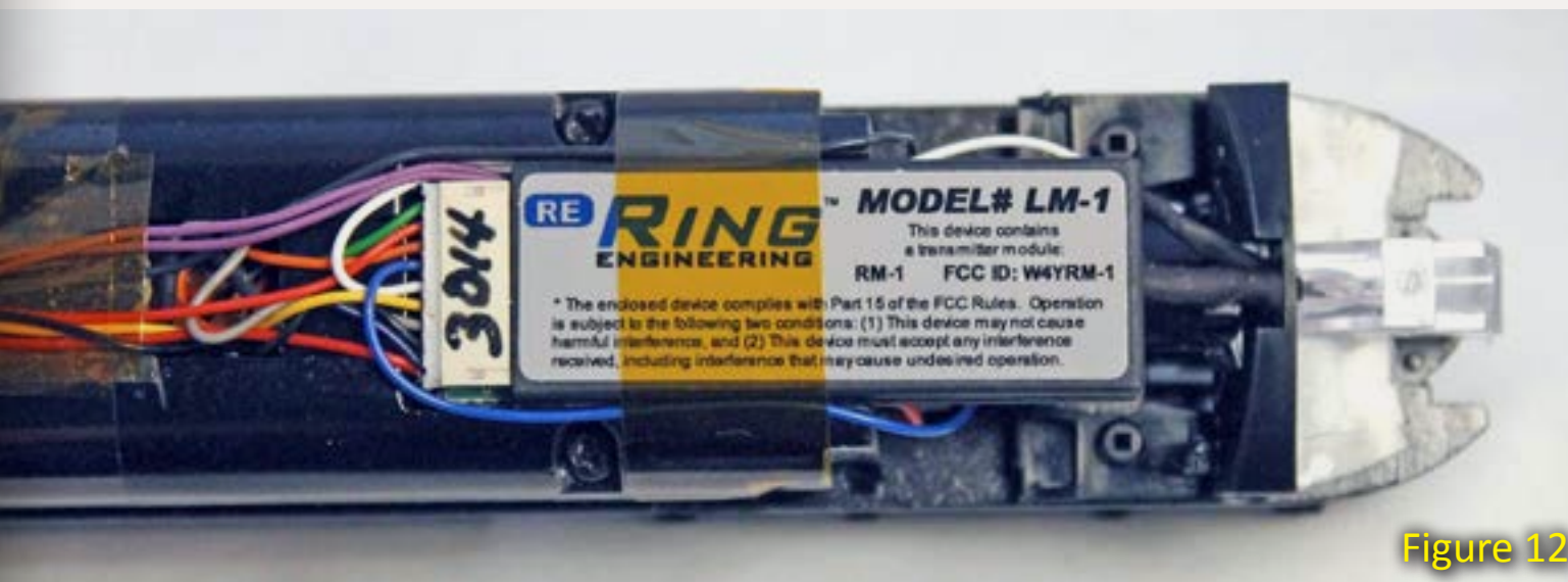
Figure 13: Close-up of installed LM-1 from the side.
