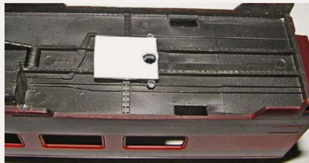
Figure 10: Using the #2 X-acto knife I bored the new pin hole starting from the bolster side first. As soon as the point of the blade comes through the inner side of the new styrene pad I bored from the interior side. I finished
