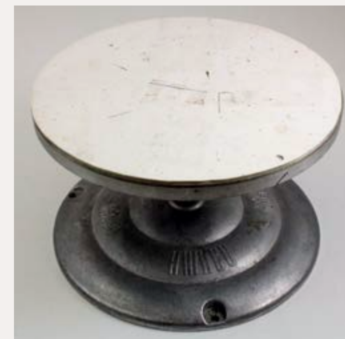
Figure 12: Amaco No. 5 Decorating Wheel modified by adding foam placemat material to the top surface.
