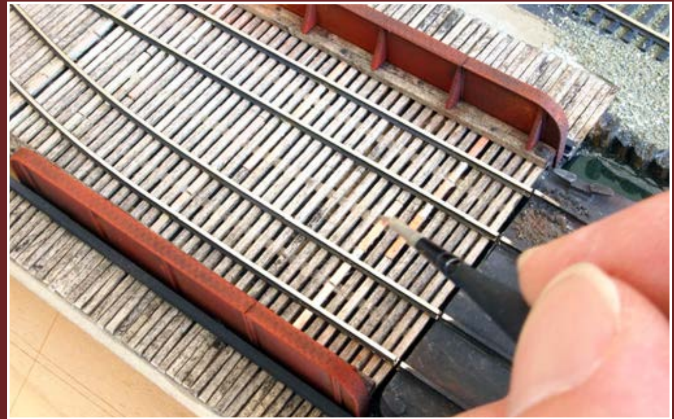
Figure 12: After soldering the rail to the apron deck, we cut the rail at the car float edge to relieve any tension on the Gorilla Glue bond along the rails. A few coats of Floquil mixed paint turn the PC boards into wood ties.
