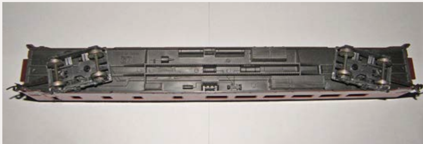
Figure 2: Looking at the underside of the car, we see the snap-fit bolster pins and the original 4-wheel trucks.
