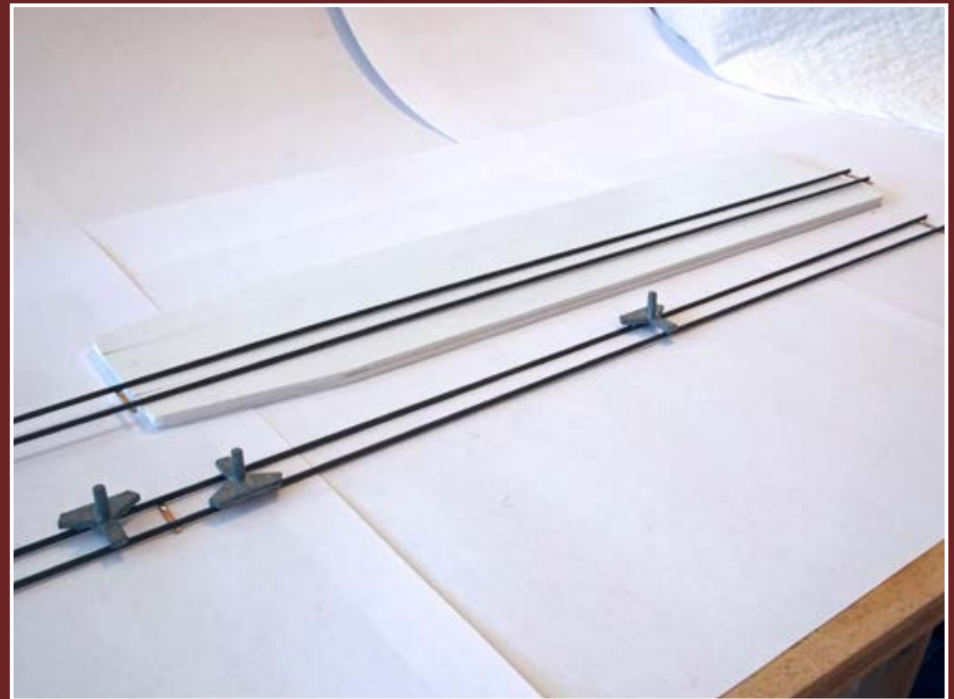
Figure 4: Two PC board ties and three-legged gauges will ensure rail spacing. After applying a thin layer of Gorilla Glue under the rails, trust your eyeball to align the rails along the 1" track center pencil lines.
