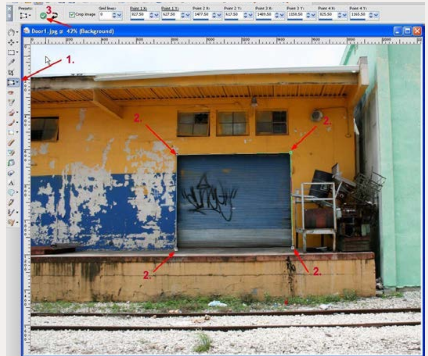
Figures 3: Because of natural perspective issues, the photo of the door is slightly trapezoidal in shape and noticeably tilted to one side. In many cases you'll find that your photos have an even more pronounced perspective distortion. Paint Shop Pro has a very simple and effective tool called 'Perspective Correction' that quickly cleans up the distortion. 1. Click the perspective correction icon. 2. A box will appear on the screen. Drag each dart on the screen box to a corner of the door in your image. 3. Hit the green check mark. That's it! Almost like magic the distortion has been fixed.
