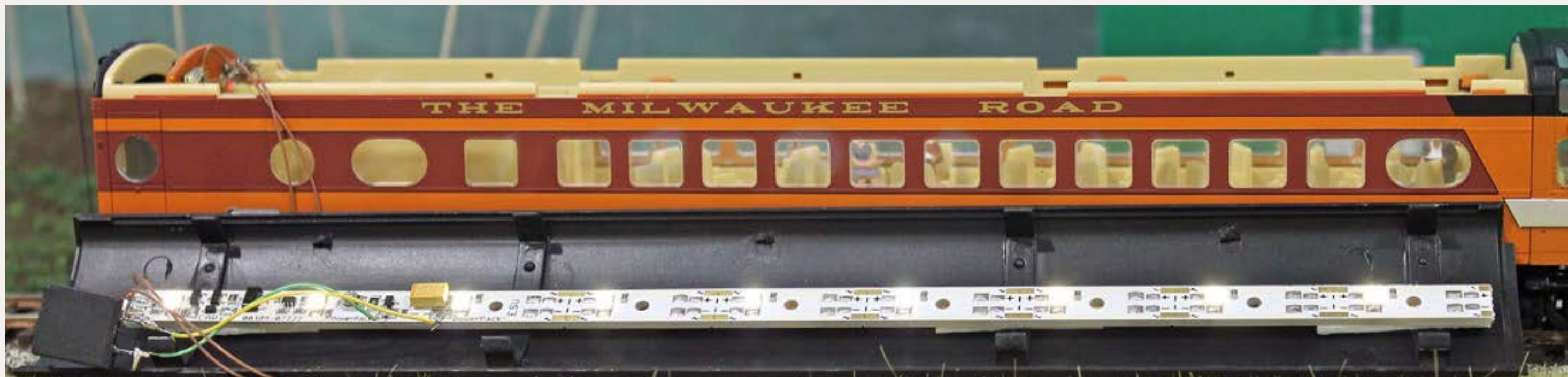
Figure 4: Lighting strip installed and illuminated.
