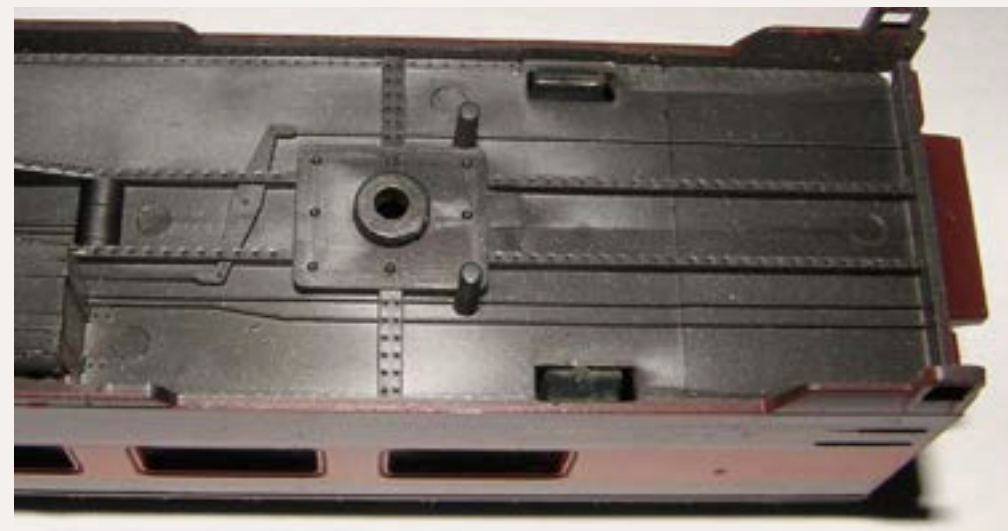
Figure 4: Removing the truck reveals the molded-on bolster. Take note of the location of the three rivets closest to the end of the car on the bolster pad (between the two short pins). The new bolster hole will be in the location of
