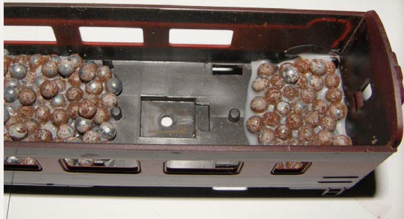
Figure 7: I like my cars super-weighted! This car is a long-time veteran on my railroad and the b.b.'s are showing their age but they do the job and do it inexpensively! The depression in the car floor needs to be filled to make up for the difference we removed from the original bolster so the bolster pins will click-in and stay. I cut two pieces of .030 styrene (not shown) and filled the depression with them.
