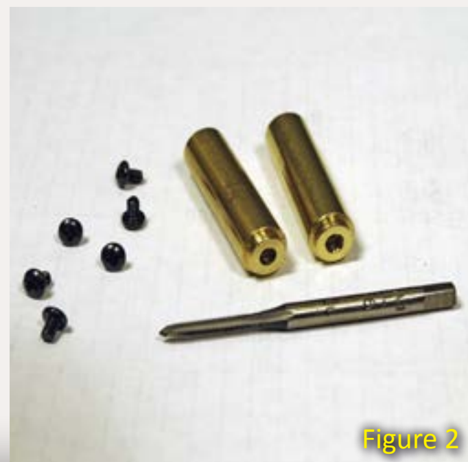
Figure 4: The resulting hole is clean and centered, with no spreading of the mounting post. Notice the hand-located (and off-center) hole for the truck mounting.
