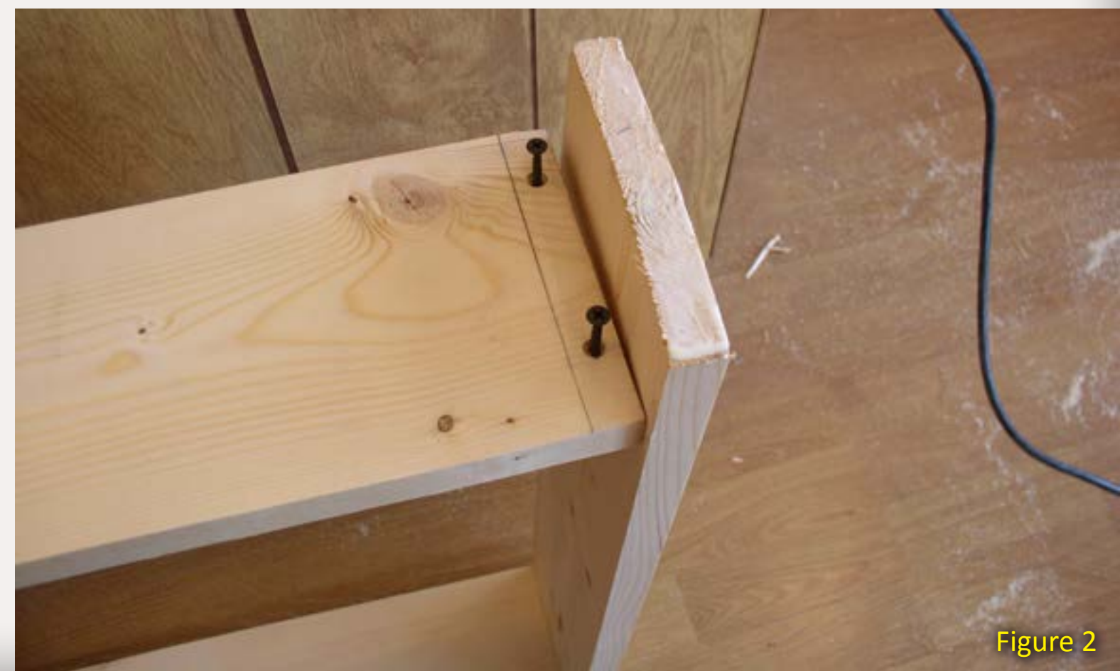
Figure 2: All the wood joints are glued and screwed for strength.
