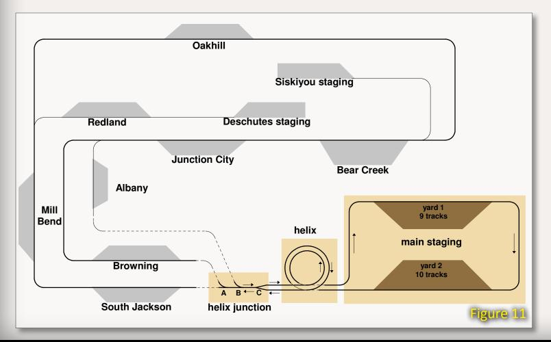
traversing "helix junction" and taking the inner (steeper) track down the helix. Trains leaving staging take the outer (less steep) helix track. Turnouts A and B (figure 11) route emerging trains to South Jackson (east end of the layout), Browning (west end of the layout), or the Toledo branch (passing through Albany).
