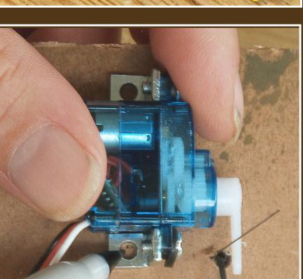
Figure 8: To mount the servo I used prethreaded L-brackets available from Tam Valley Depot. You could also use small blocks of wood. The hard rubber black washer came with the servo. Some brands of servo don't use them.
