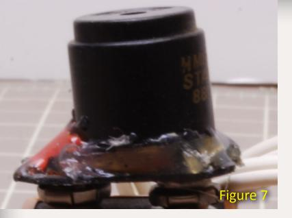
Figure 7: Hot melt glue works well, to fill the gap and hold the parts firmly together. I take my time with the glue, allowing cooling before filling more of the gap.
