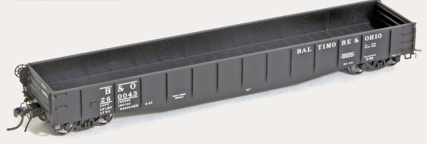
Tangent Scale Models' 70-ton, riveted, drop-end Baltimore & Ohio gondola is a meticulously scaled **HO model** of the 52' 6" prototype the Bethlehem Steel Corporation built for B&O in 1937.
