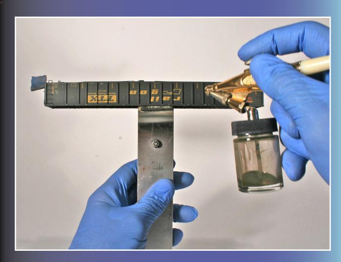
Figure 4: Several light passes with an airbrush add overall weathering on the exterior.
