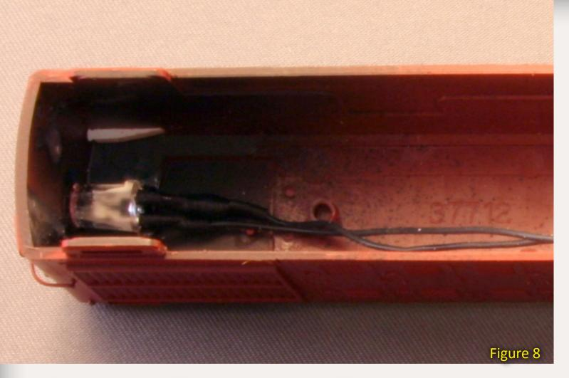
Figure 8: 5 mm LED as part of an Atlas RS-1 sound installation. Figure 9: Kato RS-2 light pipe replacement.
