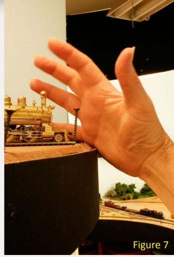
Figure 7: It seemed prudent to add stop blocks anywhere a train might drive off the layout. Management used drywall screws to temporarily eliminate this possibility. Better looking Lexan shields will replace these when I have more time.
