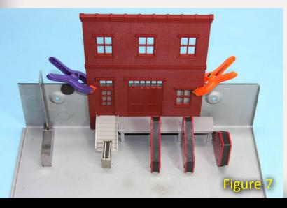
It help avoid mistakes and lets me test kitbashing ideas with different combinations of parts. The red magnetic welding holders are luxury items, they are strong, square, and can be used in various ways to form different angles. A clever person would probably magnetize the machinist's squares.
