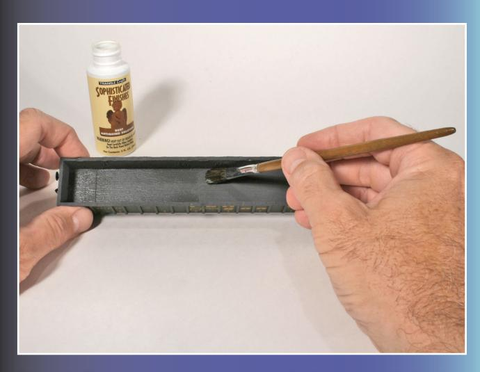
Figure 8: The rusting solution is a clear fluid that is applied to the dry iron metallic paint to start the rusting process.
