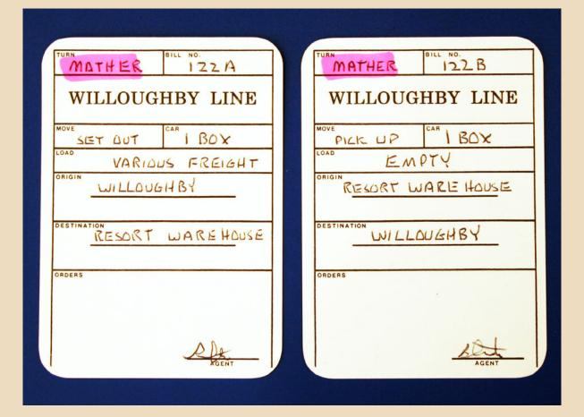
Figure 21: Note these cards have the same number but different letters (upper right). Each card specifies the number of cars to be moved, the type of car, and the origin and destination location. Specific car numbers are not used with these cards.
