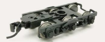
Wheels of Time (wheelsotime.com) is selling an N scale six-wheel heavyweight drop-equalizer passenger truck with an 11' wheel base at \$12.89 a pair. The model truck features 36" metal wheelsets, adjustable draft gear,
