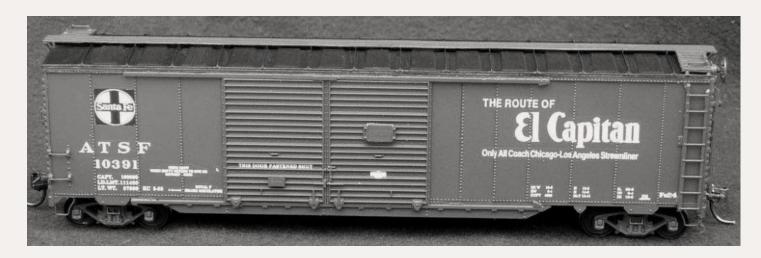
compensate for the extra-wide 14' door opening, a reinforcing sill was added under the door and adjacent section. For additional strength, the number of internal posts to the right of the door was increased, which accounts for the unusual design of seven panels on the right and four wider panels on the left. In late 1948, ATSF raised the roof 12" on 79 cars (below) to handle Plymouth and Dodge auto bodies that were transported stacked on their ends.
