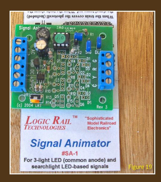
Figure 19: I am going to use this Signal Animator board from Logic Rail Technology to control the board. The board has three outputs, Y, R, G that go low when they are active, which is ideal for the Dual 3-Way I am using to control the servo.
