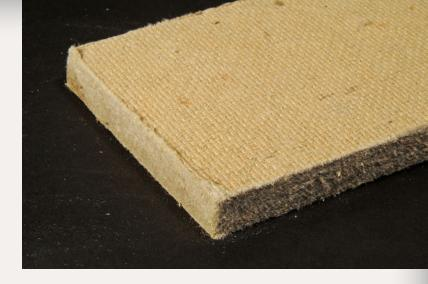
Figure 2: Recycled newspapers and cardboard are ground up, saturated, and pressed to form Homasote, a building board product popular for quiet roadbeds on model railroad.
