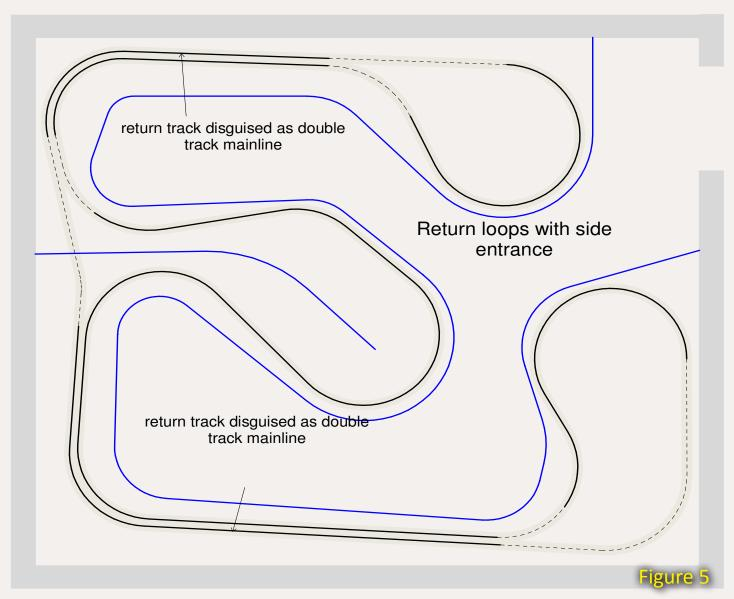
Figure 5: The hidden "return" track has been "daylighted" in two places and disguised as the opposite direction track of a section of double track mainline. A crossover in these locations will create a reversing loop.
