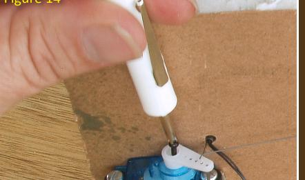
Figure 12: At this point I needed to power up the servo to center it. If the servo arm is put on randomly it may pull the semaphore out of its hole or bend the wire. All the next steps were done with the servo connected to the driver board (Dual 3-way in my case) and with the servo powered up.
