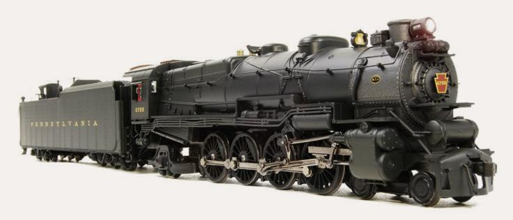
came equipped with large class 210F75 tenders. At the end of WWII, some of the original locomotives were modified for increased boiler pressure and the addition of circulators to the firebox. These became the M1b versions.
