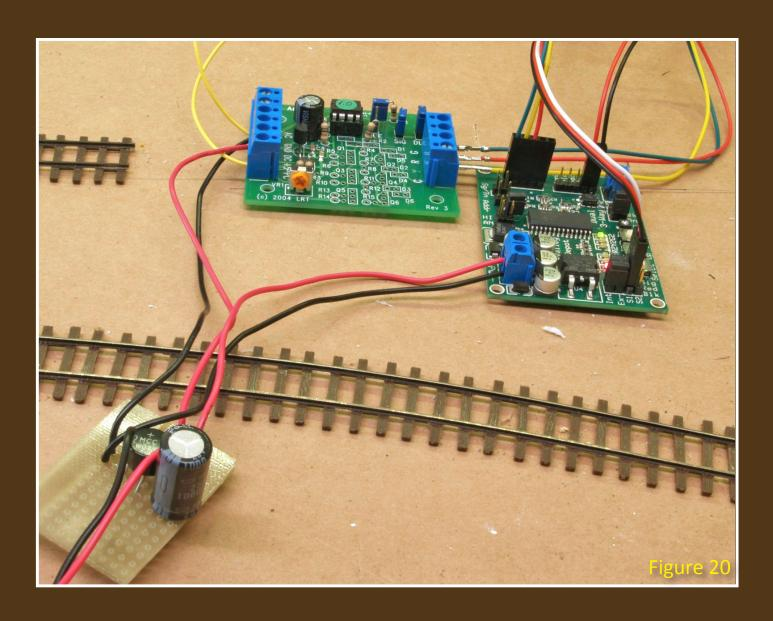
Figure 20: I've installed the boards temporarily above the layout so I could troubleshoot more easily. When everything was working I moved the electronics below the layout. I built a small DC power supply to connect both boards to my AC accessory bus. It's just a bridge rectifier and a capacitor. However, any DC power supply that puts outs at least 500 mA would have worked.
