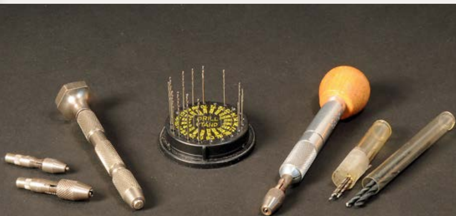
Figure 3: For drilling, have a selection of drill bits and holders available, including duplicates of the most-frequently used drill sizes.
