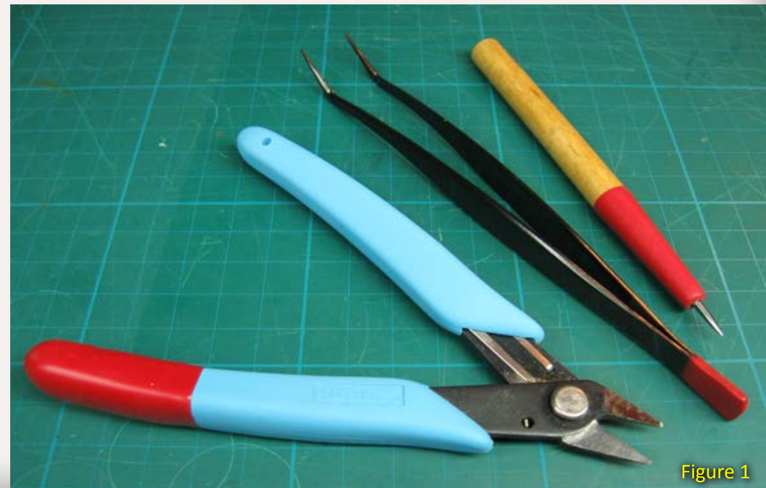
Figure 1: A red “plastidip” coating on my tools makes them easily identifiable in a tangle of tools next to a layout.
