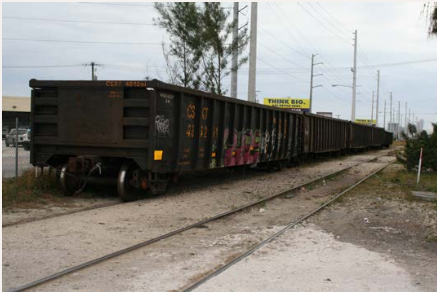
Figure 1: Several gondolas await loading on a siding in Miami outside of a scrap metal processing facility. These gondolas have seen many years of service and their rusted and battered condition can be modeled easily.
