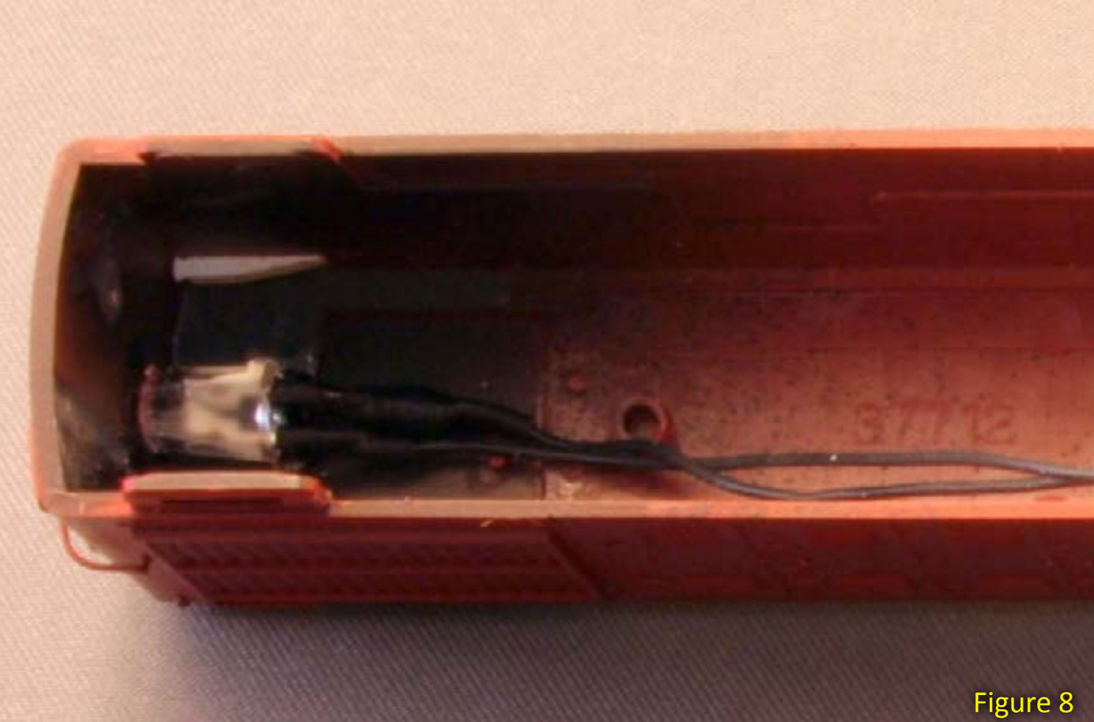
Figure 8: 5 mm LED as part of an Atlas RS-1 sound installation.
