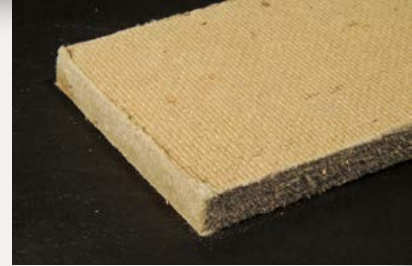
Figure 2: Recycled newspapers and cardboard are ground up, saturated, and pressed to form Homasote, a building board product popular for quiet roadbeds on model railroad.
