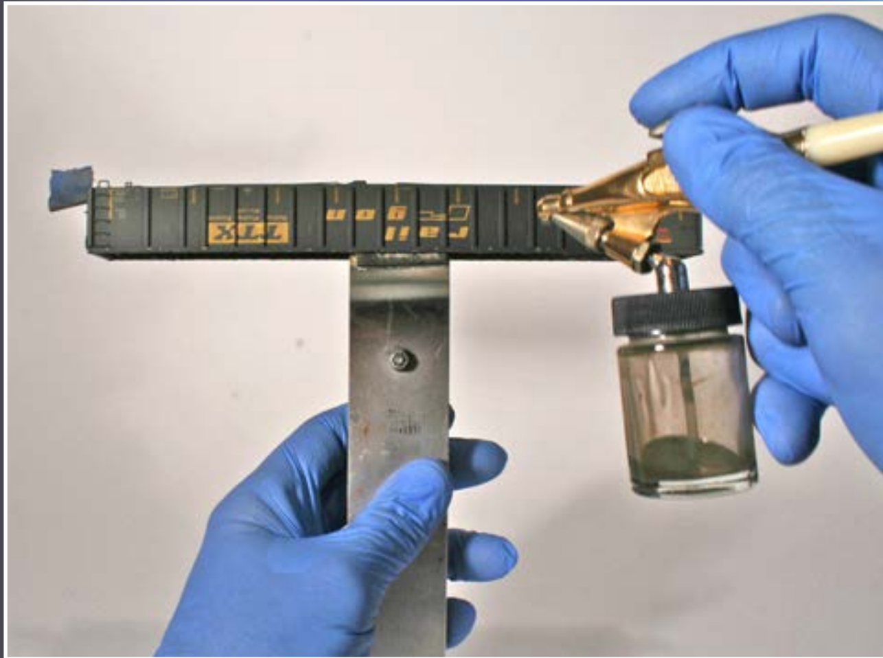
Figure 4: Several light passes with an airbrush add overall weathering on the exterior.
