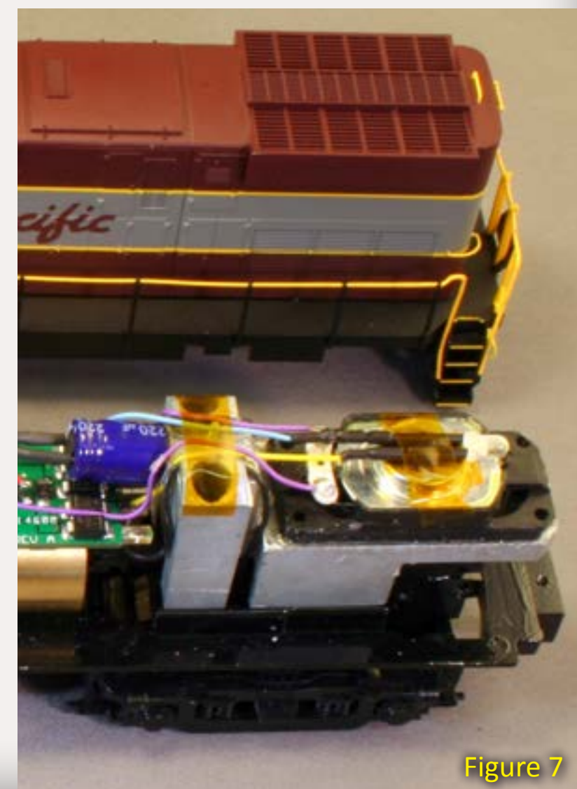
Figure 6: Golden-white LED in an Athearn blue-box locomotive.
