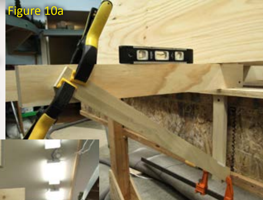
Figure 10a: Once the plywood roadbed was cut to size, I installed permanent joists to support it. I used clamps and a level to ensure the roadbed would also be level.
