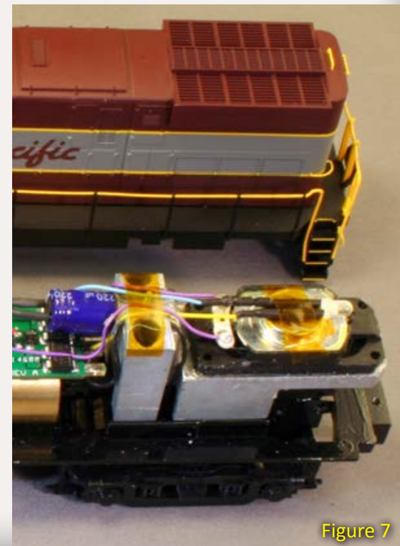
Figure 6: Golden-white LED in an Athearn blue-box locomotive.
