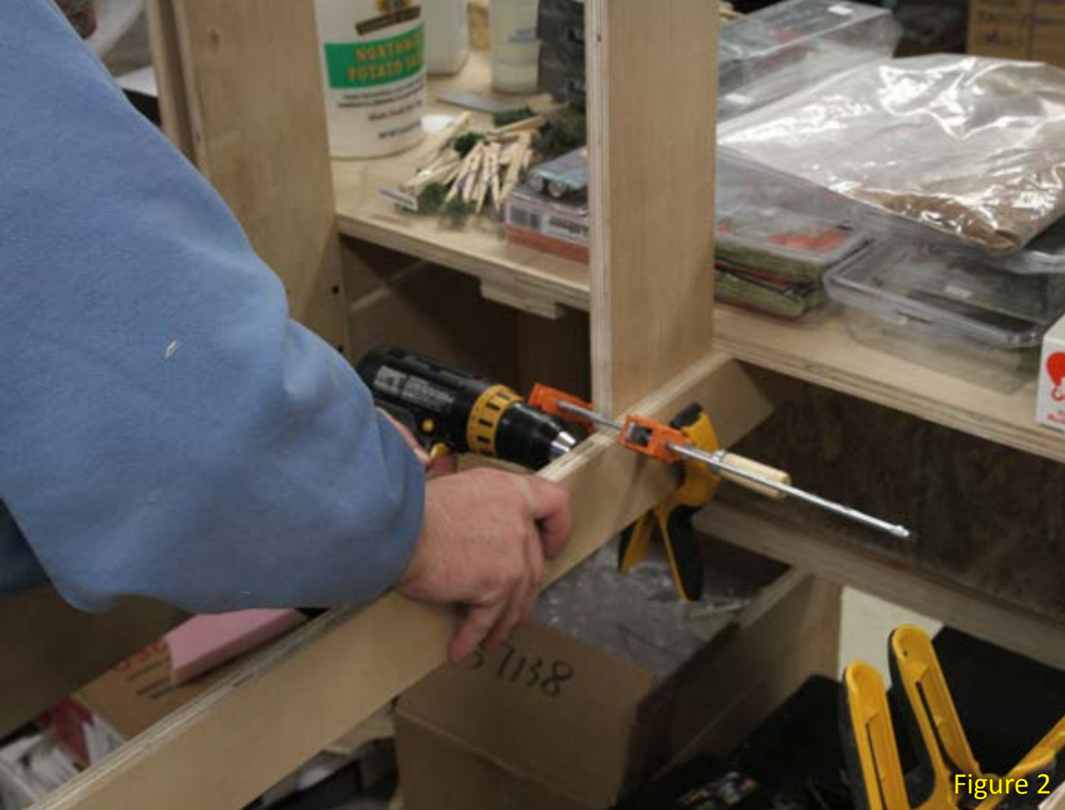
Figure 2: With the riser double-clamped in place, Mike drills pilot holes for the screws that will hold it in place.
