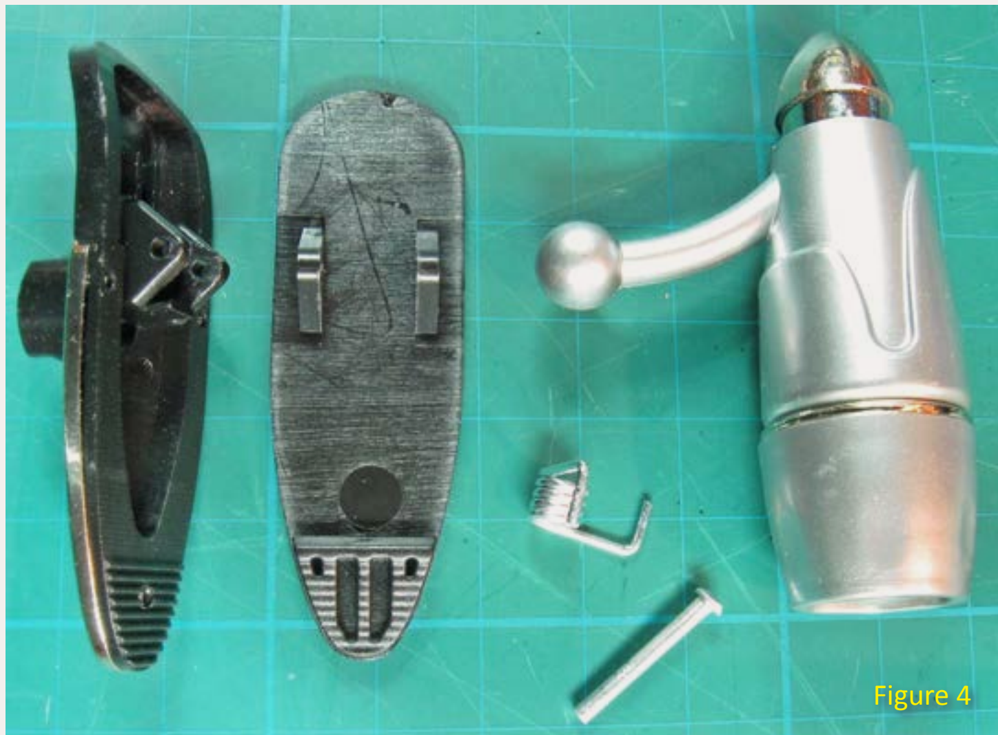
Figure 4: The clip light disassembled. We will use the upper clip (shown at the extreme left) and the light unit (in silver gray on the right).
