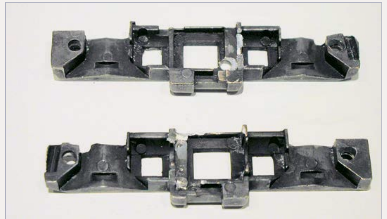
Figure 9: N Scale Bachmann F7A frame machining for DCC installation.
