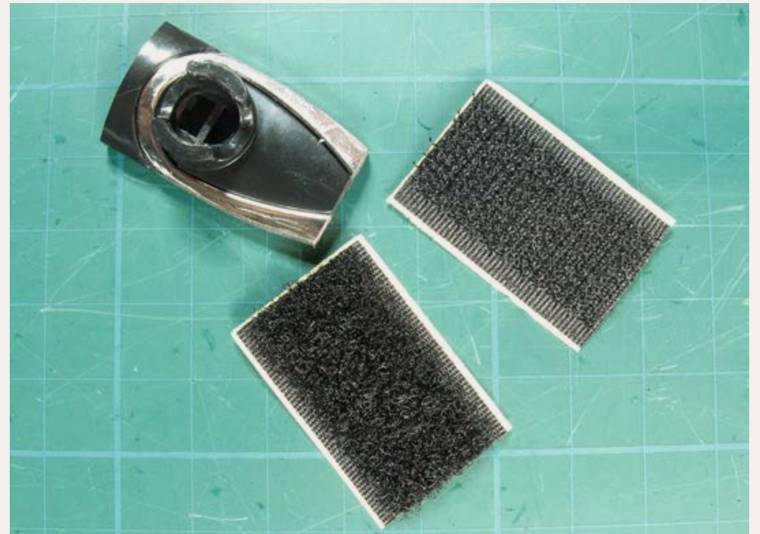
Figure 9: Cut two pieces of Velcro and add to the Optivisor and the other to the bottom of the modified clip.
