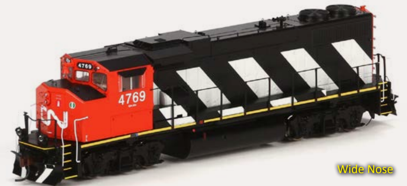
Figure 1: The difference between a standard and a wide nose GP38-2s is clearly illustrated in Athearn's HO scale model. The standard-nose SP version replicates a locomotive built by EMD in 1980, while the CN model is of a wide-nose locomotive built by MLW in the early 1970s.
