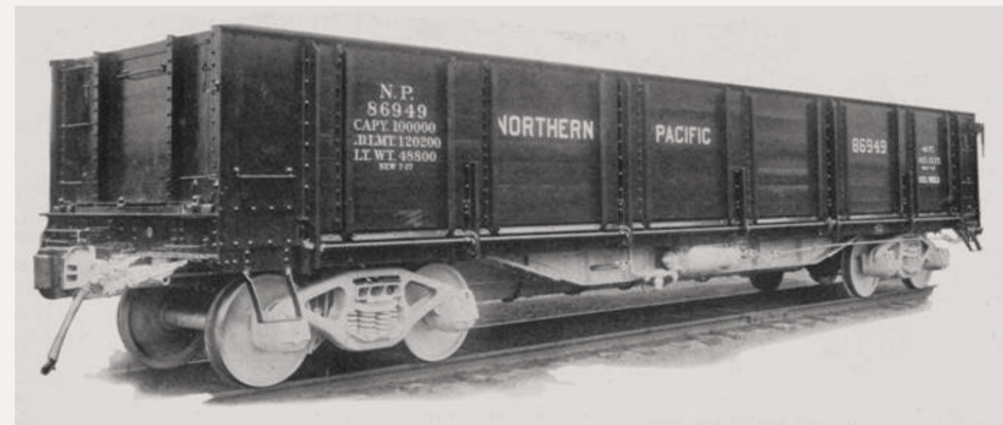
Figure 2: Builders photo of a Hart convertible car built for the Northern Pacific by the Roger Ballast Car Company in 1927. – Richard Bale collection.
