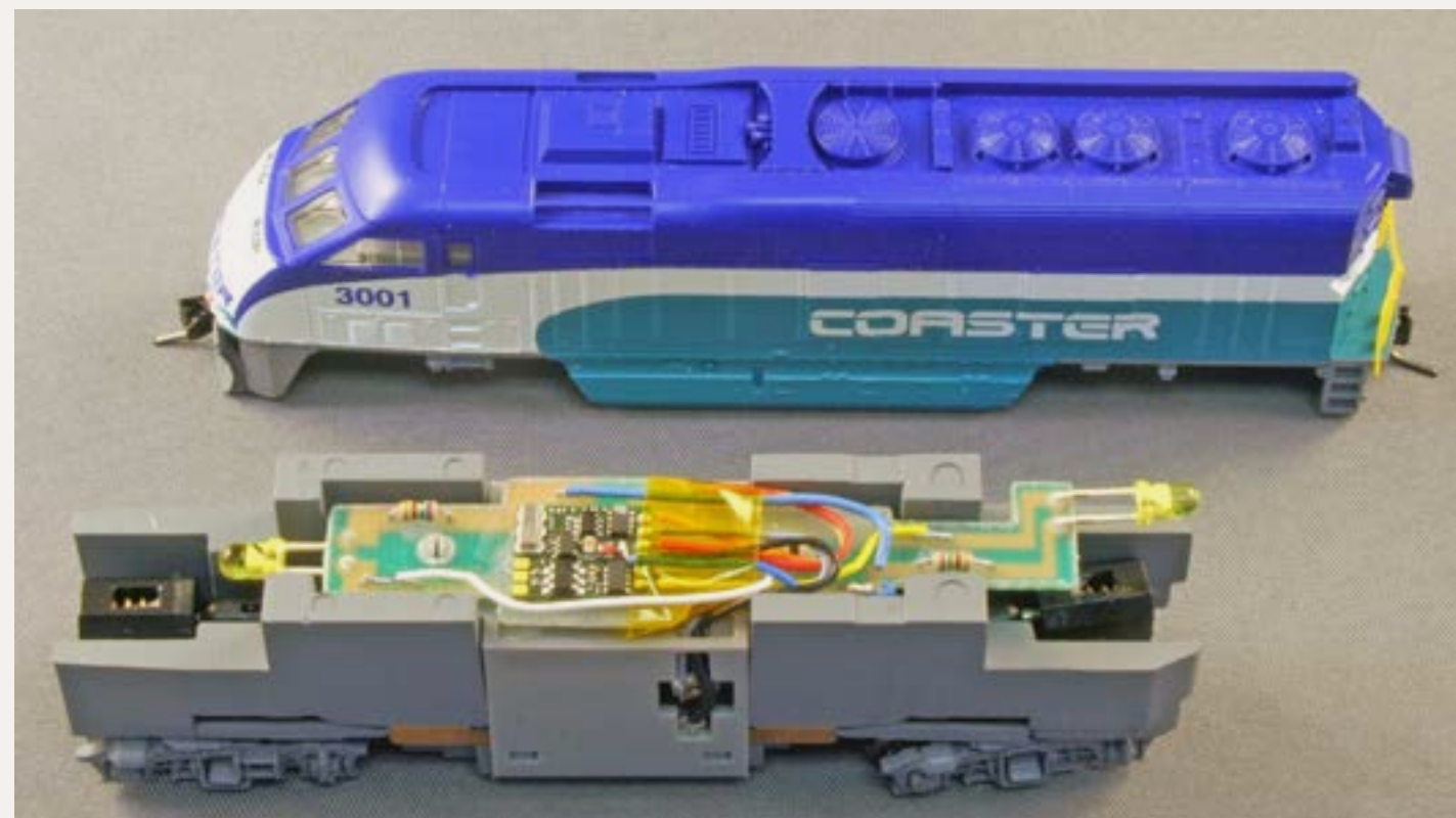
Figure 1: N scale Athearn F59PH with Lenz Silver Mini decoder.
