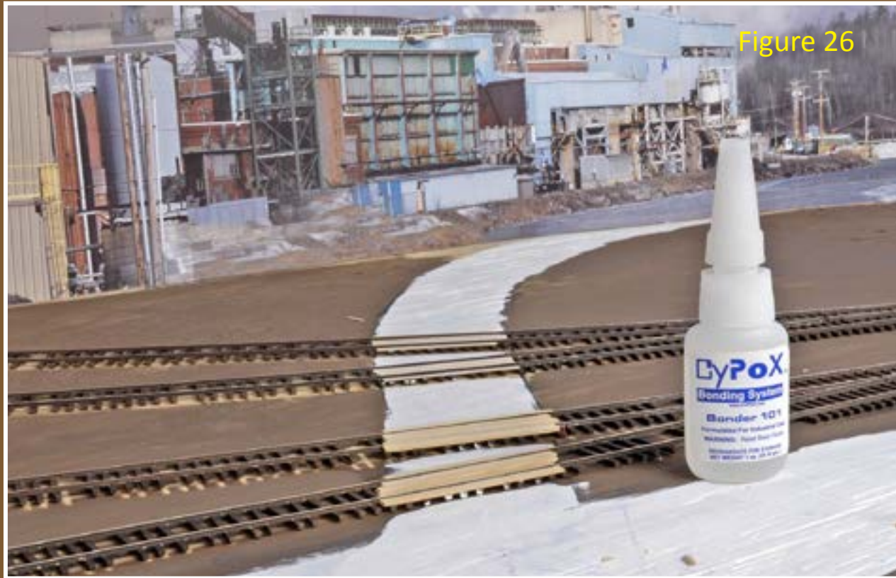
Figure 26: I secured the wood planks to the tops of the Micro Engineering plastic ties using CyPOX Bonder.
