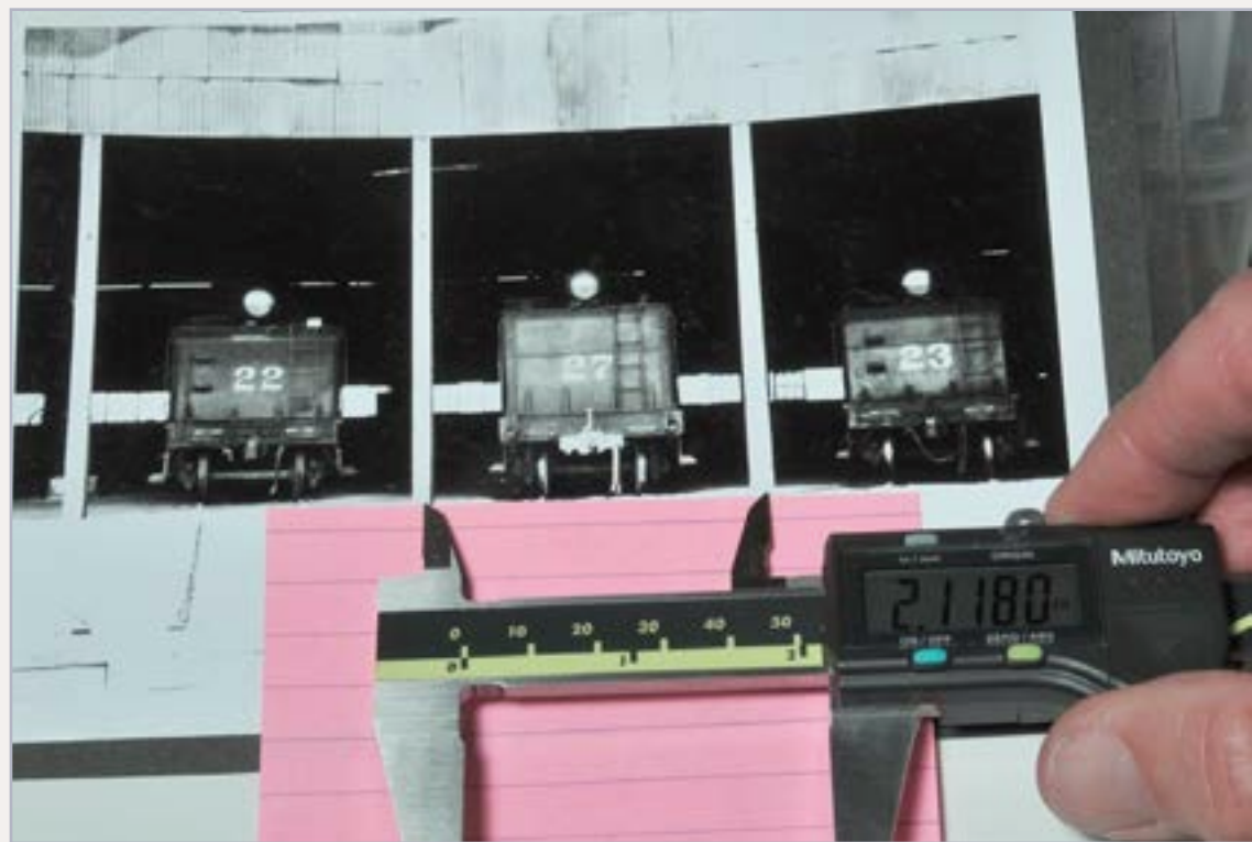
Figure 17: Measure the width of the inside edges of the rails (the track gauge) right where they cross the edge of the paper, using a dial caliper. Also measure the distance
