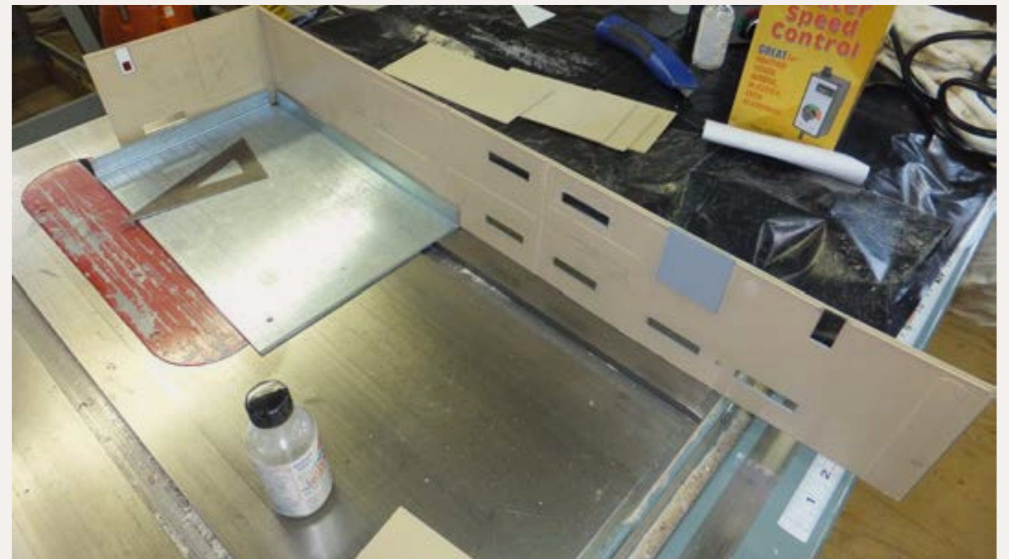
Figure 1D: Using the table saw table again, I’m beginning to assemble the wall sections, cut from the Walthers Paper Mill kit. Here I’m using a jig to make a nice 90° corner. Plastrac Pro Weld liquid cement was used extensively.
