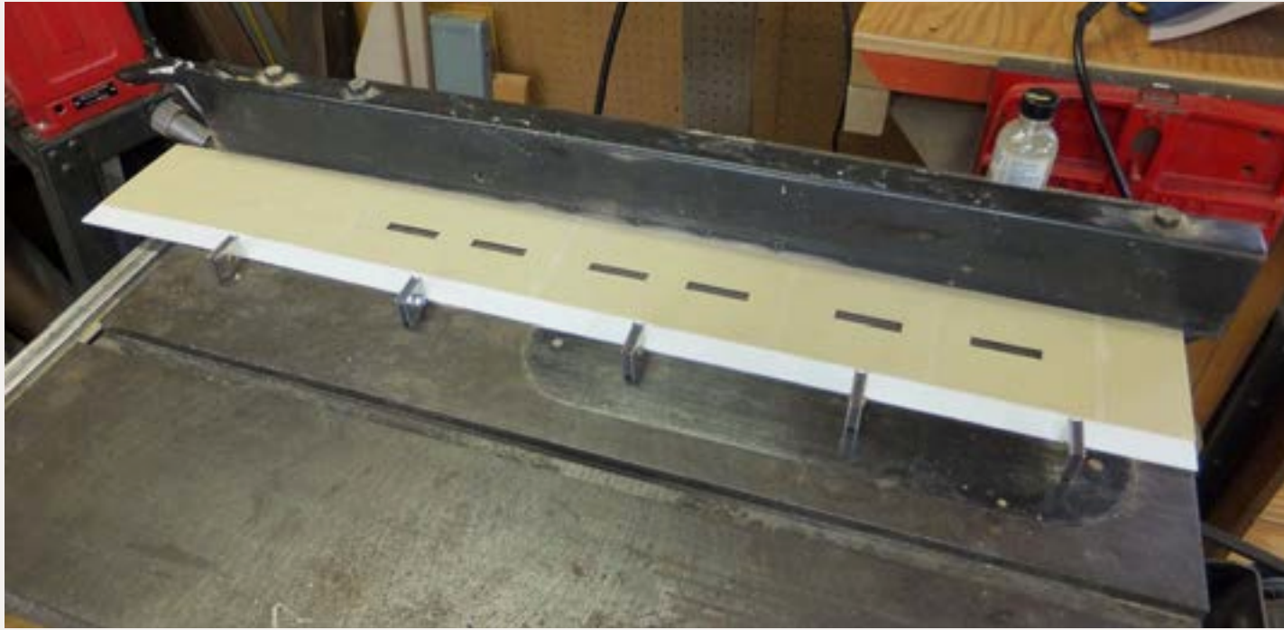
Figure 1M: Magnets hold the styrene “concrete foundation” in place for bonding with Pro Weld. Note that it’s already trimmed for length.
