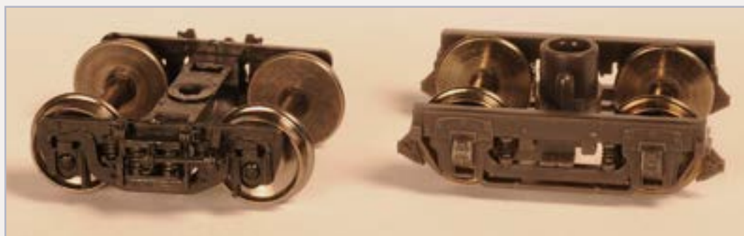
Figure 4: The Centralia model has outside swing-hanger trucks (left) applied in the 1950s to 175
