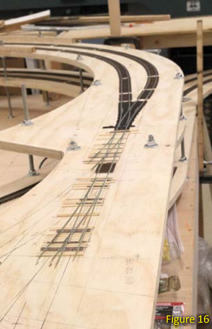
Figure 16: The helix junction with the turnouts set in place. It all looks good – time to start spiking them.
