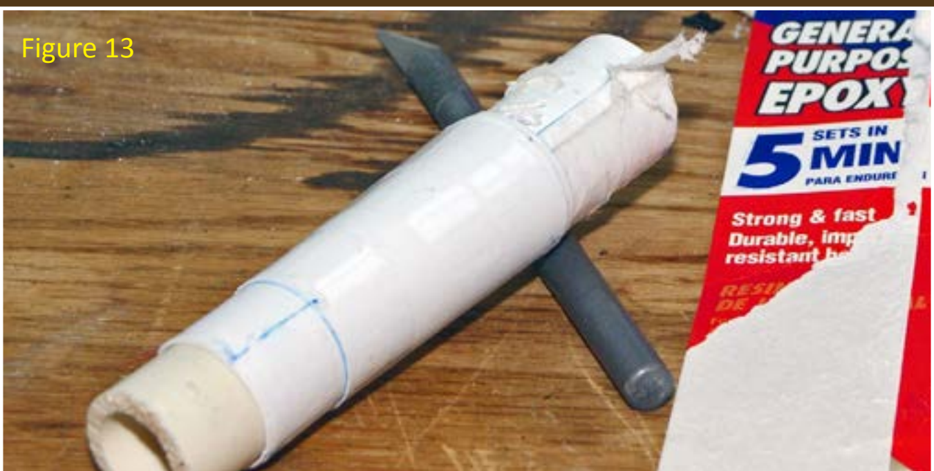
Figure 12: The tapered section is ready to be glued in place, as well as the material added to the core to build up the wider portions of the boiler and firebox. The conical wrapper does not need to be heat formed, since the core will force it to hold its shape.
