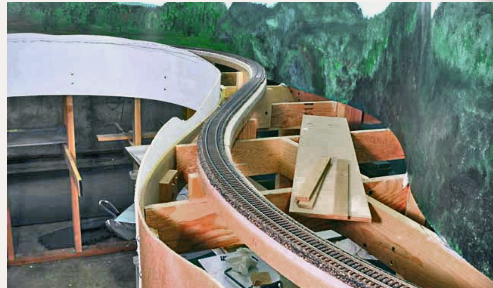
Figure 1: Spline allows long swoopy curves using a minimum of materials, but careful attention has to be paid to grades, curvature and easements.
