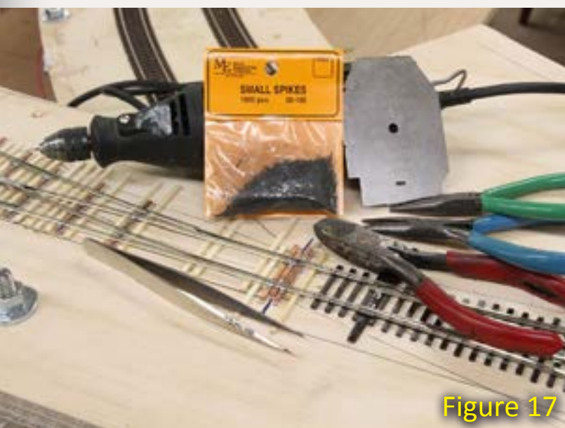
Figure 17: The tools and supplies I use when installing turnouts.
