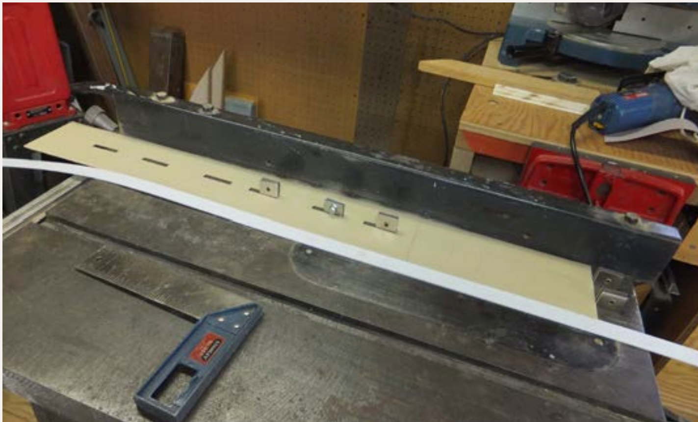
Figure 1F: More magnets are added to hold the siding in place. I'm getting ready to measure the white styrene strip to length before cementing in place. It's important to glue it with the siding good side up so excess cement does not melt the siding into the table top.
