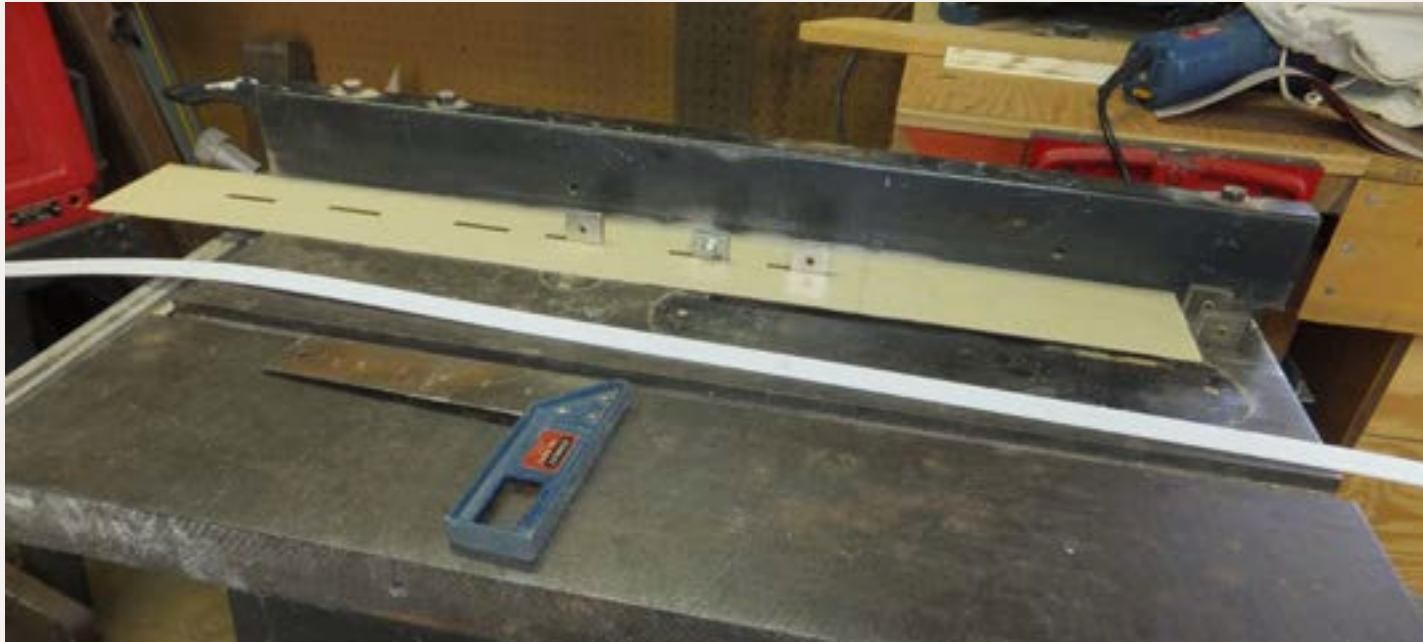
Figure 1E: I have two table saws and used both for assembly! I'm getting ready to add styrene strip to the bottom of the corrugated metal walls, to represent the concrete foundation. Note the magnets inside the window openings to hold the siding in place.
