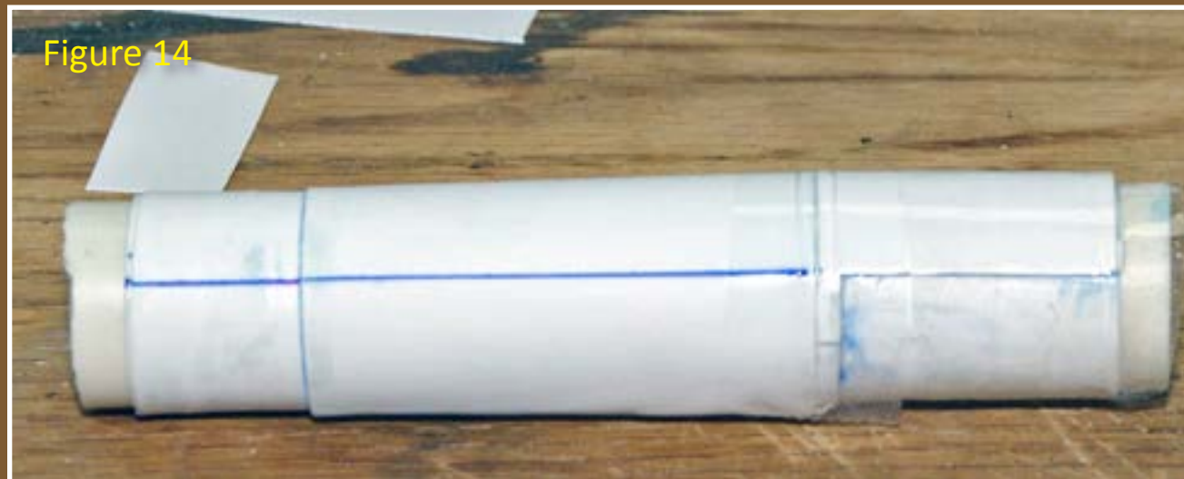
Figure 14: The boiler and firebox are taking shape. The bottom of the boiler (along the seam) shows a little irregularity, but that can be sanded out and it's not very visible underneath the model anyway.
