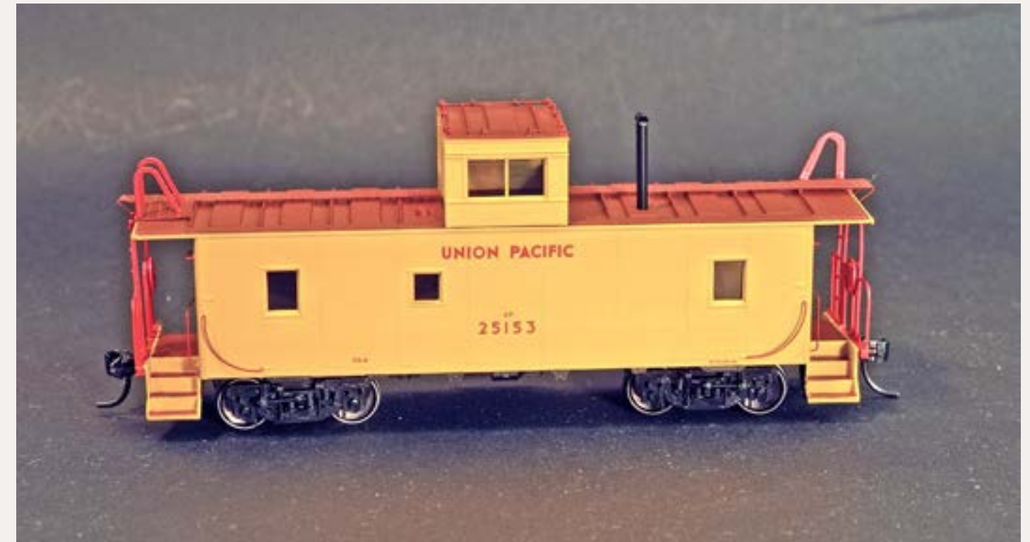
Figure 1: Centralia's CA-4 has the correct wooden end platforms and steps, and a rectangular panel Murphy roof.
