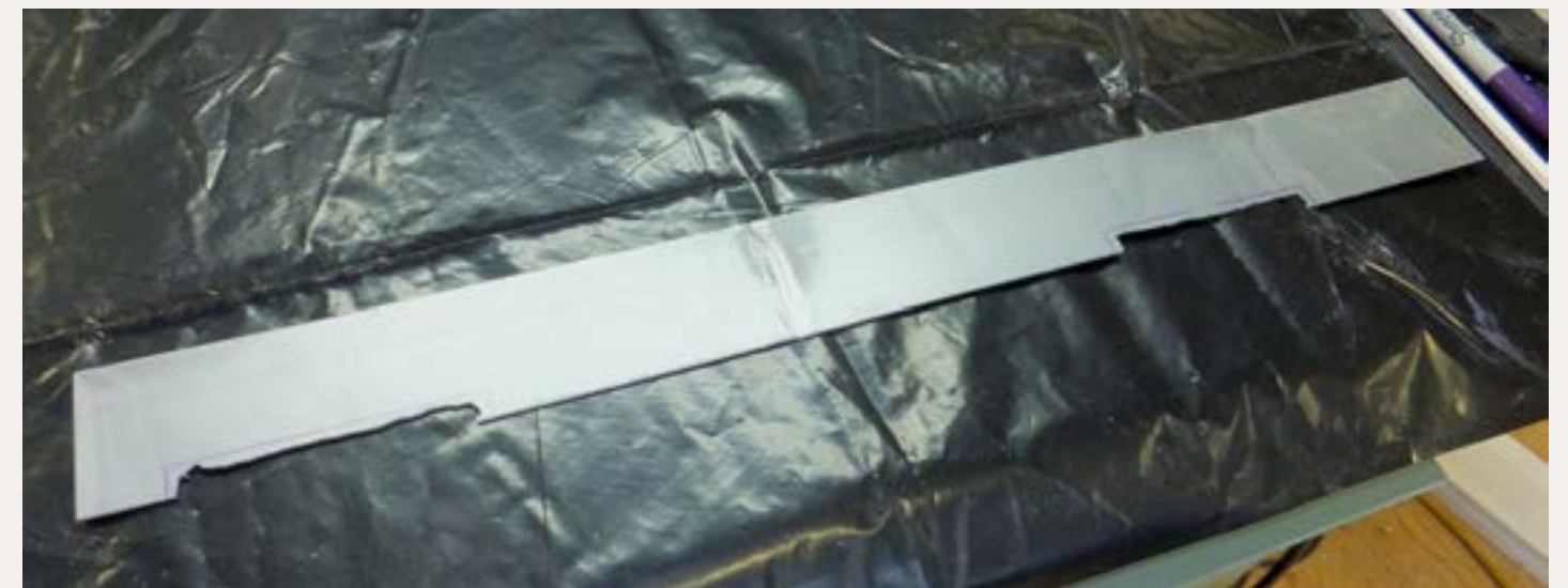
Figure 1P: Corrugated siding material has been bonded edge to edge. I'm cutting out the areas over the track dock entries to permit full height to the opening.
