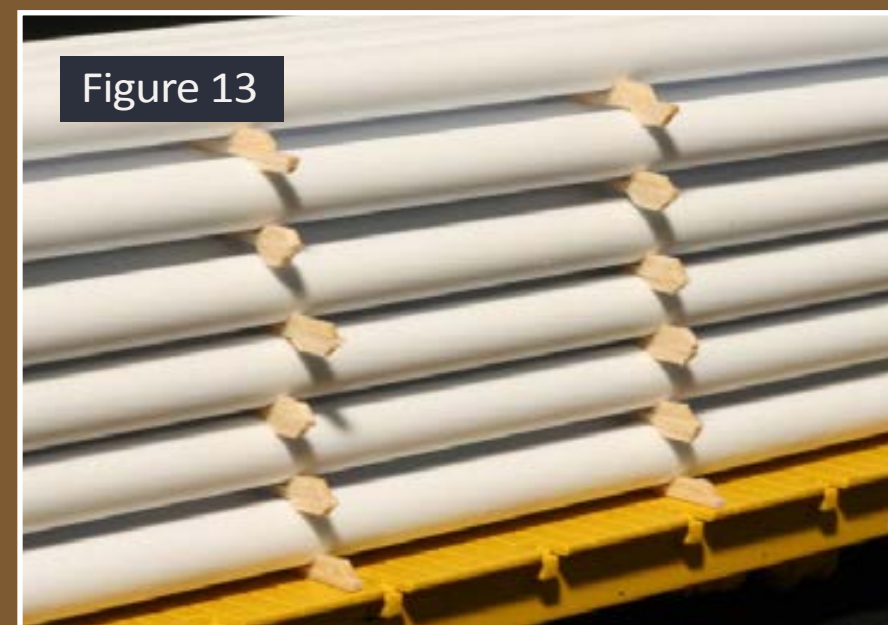
Figure 13: Once all the runners are complete, the individual tiers can be 'test-stacked' to determine if any additional trimming is necessary.
