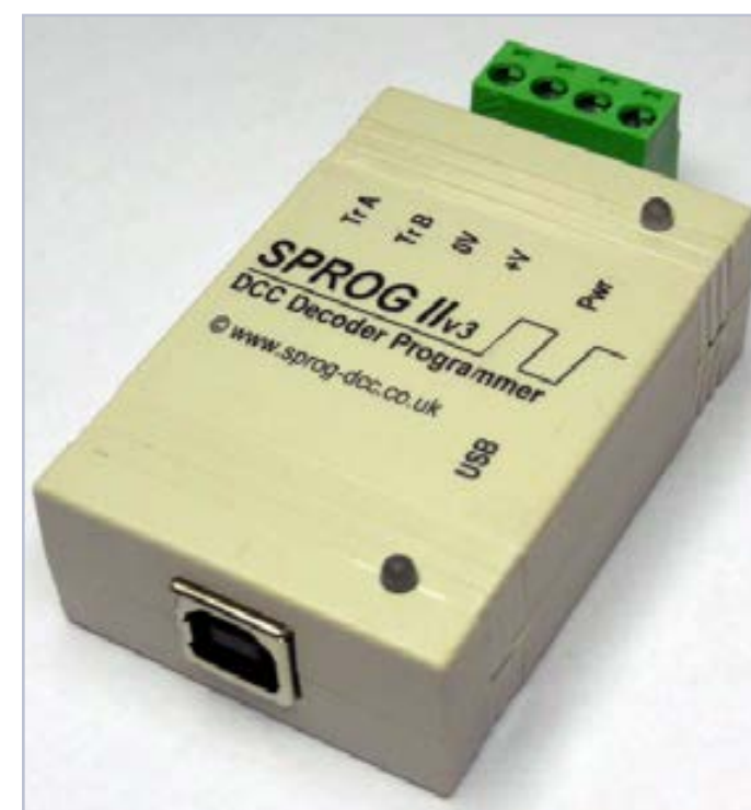
Figure 6: SPROG stand-alone programmer – photo courtesy Andrew Crosland.
