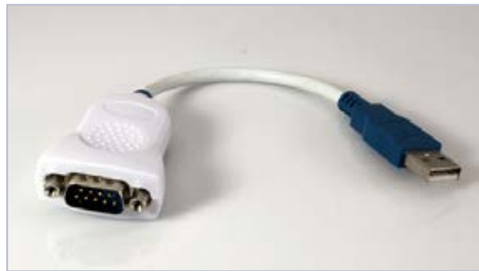
Figure 7: RS232 to USB adapter – ES-U-1001-B10 from EasySYNC.
