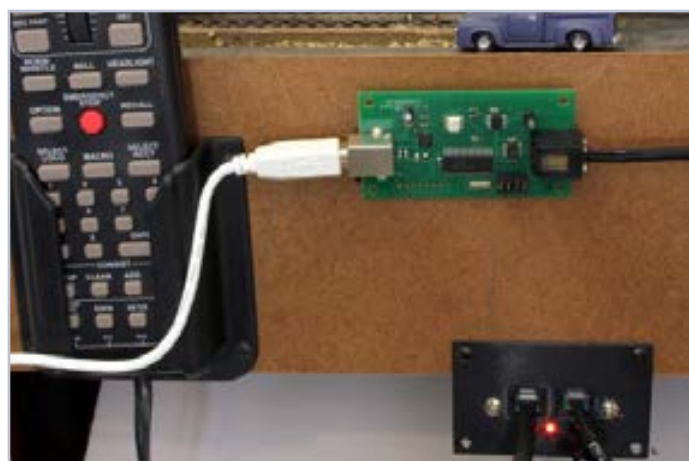
Figure 4: The NCE USB adapter in use with the PowerCab on my layout.
