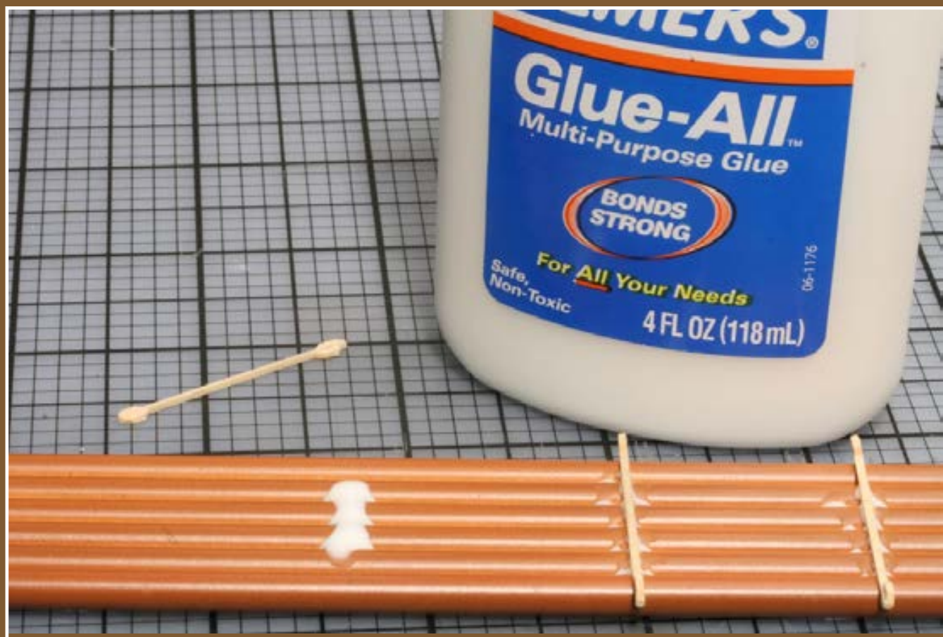
Figure 14: Gluing the runners to the tier of pipe will make handling easier while the load is still under construction, and will also make the load sturdier once it is complete.
