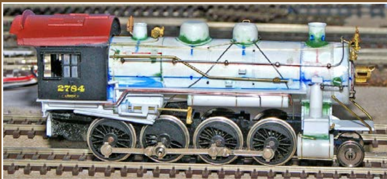
Figure 16: Here you can see the brake pipe, cooling line for the main reservoirs, air lines for the bell ringer and sanders, and the ash pan fitted to the bottom of the firebox. There are also lines running to the generator and power reverse. The engineer's side detailing is done at this point.
