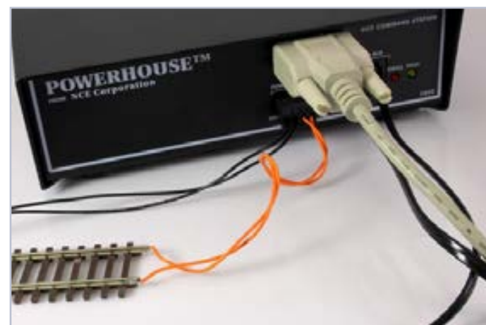
Figure 5: NCE command station with RS232 cable interface.
