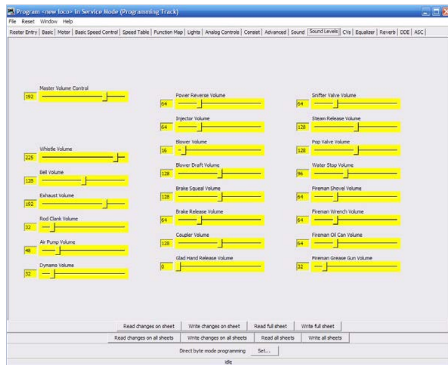
Figure 12: Tsunami Sound level page in DecoderPro.
