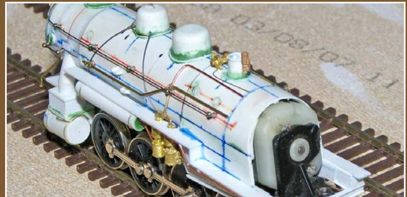
Figure 18: Rather than continue the plumbing inside the cab, with the associated challenge of fitting it through the cab wall or fitting the cab around it, I chose to simply end the plumbing at the cab wall. It's nearly invisible unless you look very closely, and it made construction a lot easier.
