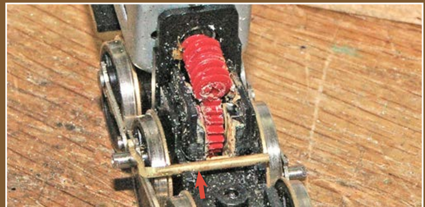
Figure 10: The power-reverse lever is glued to the chassis (red arrow). This interfered with the electrical contacts on the frame, so I removed them and made my own.
