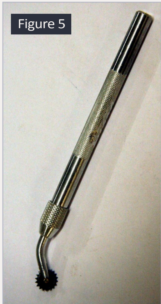
Figures 5-6: A pounce wheel was used to transfer lines from the plans to the plywood base.
