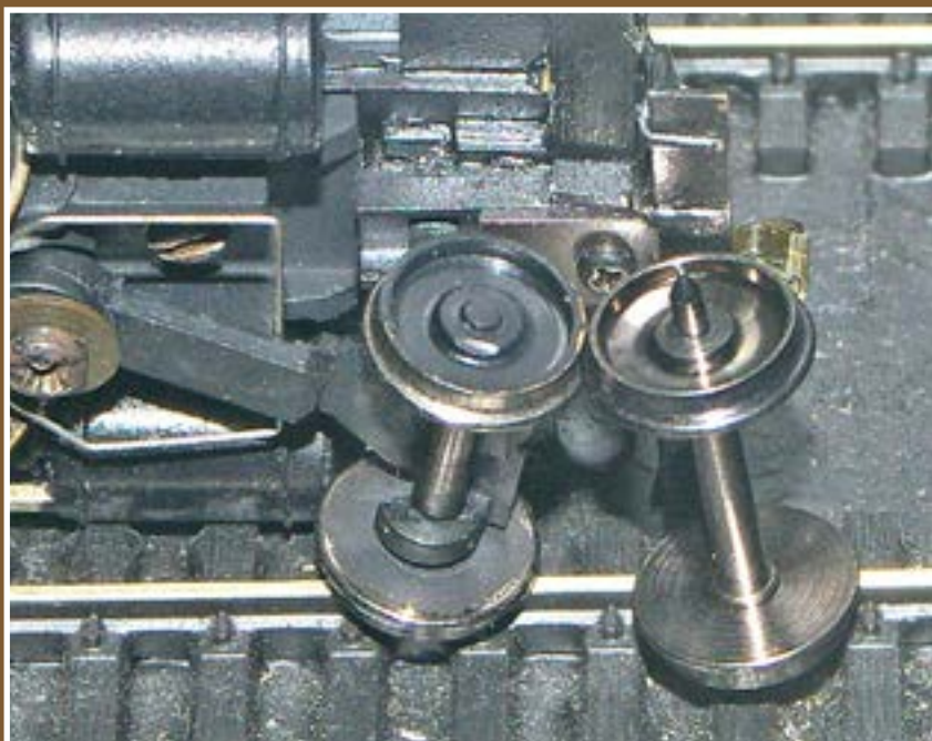
Figure 25b: Finished pilot wheels after modifying the axles.
