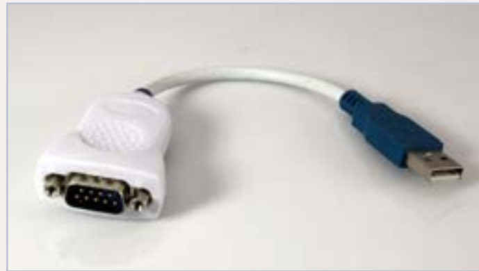
Figure 7: RS232 to USB adapter – ES-U-1001-B10 from EasySYNC.
