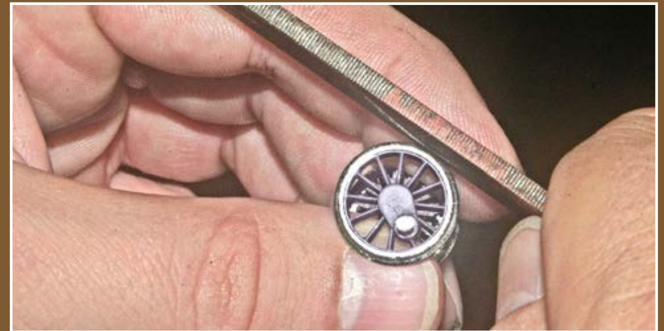
Figure 25b: Filing down too-deep flanges on a driver.
