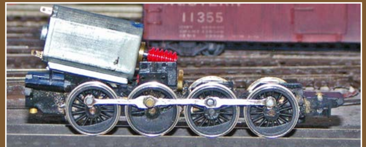
Figure 30: The new rods have a much finer profile than the originals did.
