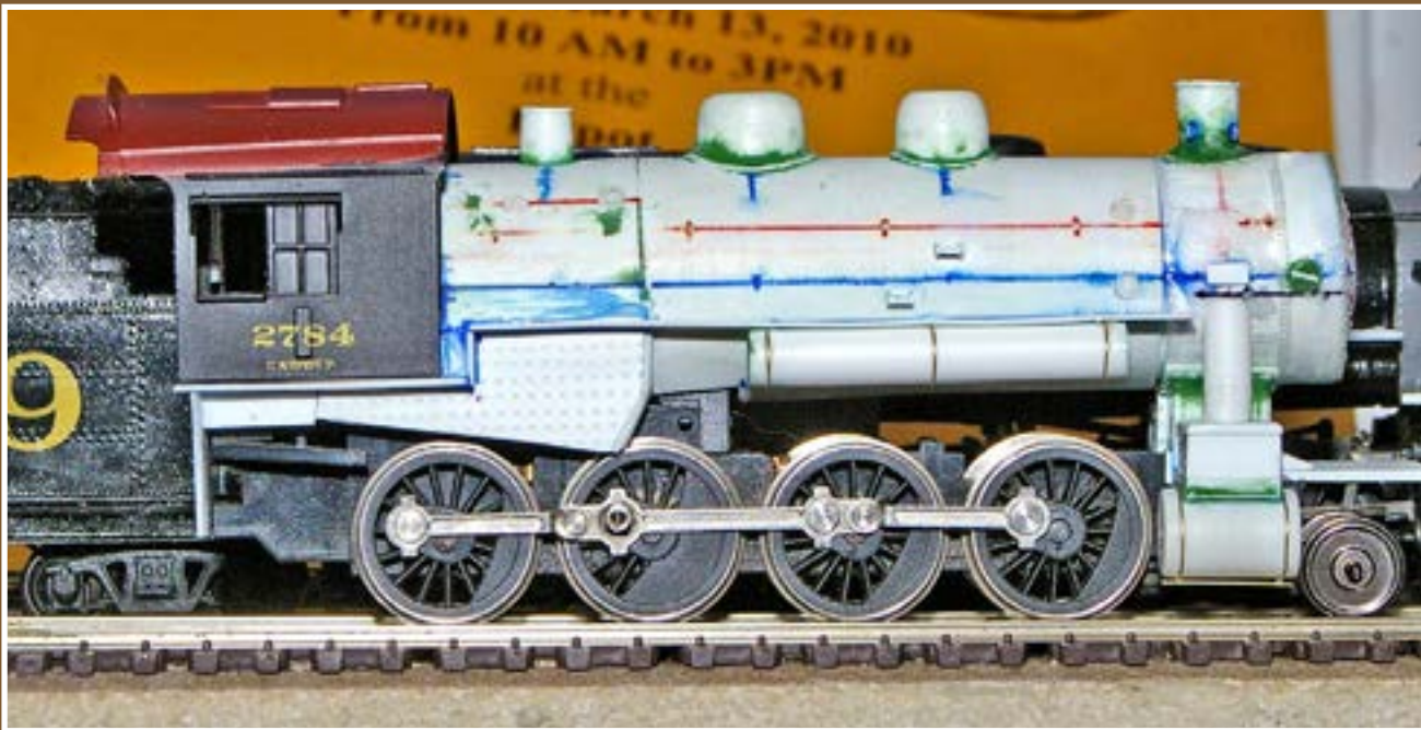
Figure 7: The firebox overlay is in place here, along with the smokebox cleanout and builder's plate. Also clear in this angle is how the #3 driver is recessed into the firebox, a compromise required because the drivers are too large and too widely-spaced, compared to the prototype. Many commercial models are lengthened to disguise this, but I chose to make the boiler the correct prototypical length.
