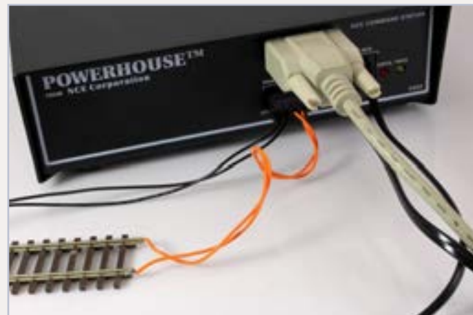
Figure 5: NCE command station with RS232 cable interface.
