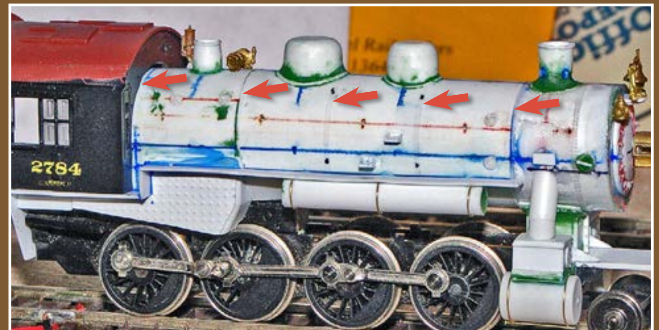
Figure 8: While they are difficult to see (marked with red arrows), the lagging bands have been added. The black marks on the boiler were used to get the correct spacing.
