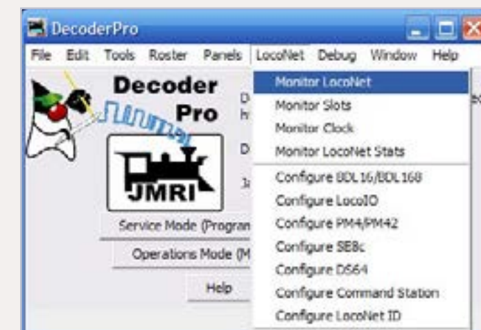
Figure 8: DecoderPro Screen shot with Monitor LocoNet selected.
