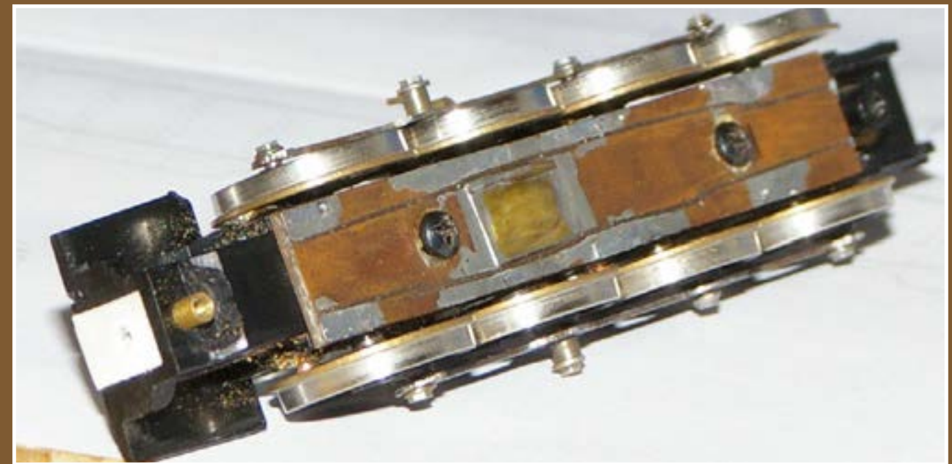
Figure 23: I ended up removing the first wipers, leaving the bottom cover a lot uglier than it needed to be.
