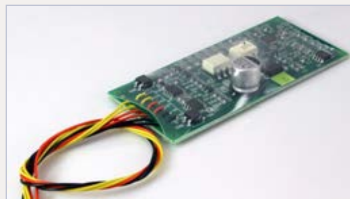
Figure 9: SoundTraxx' PTB100 Programming Track Booster.
