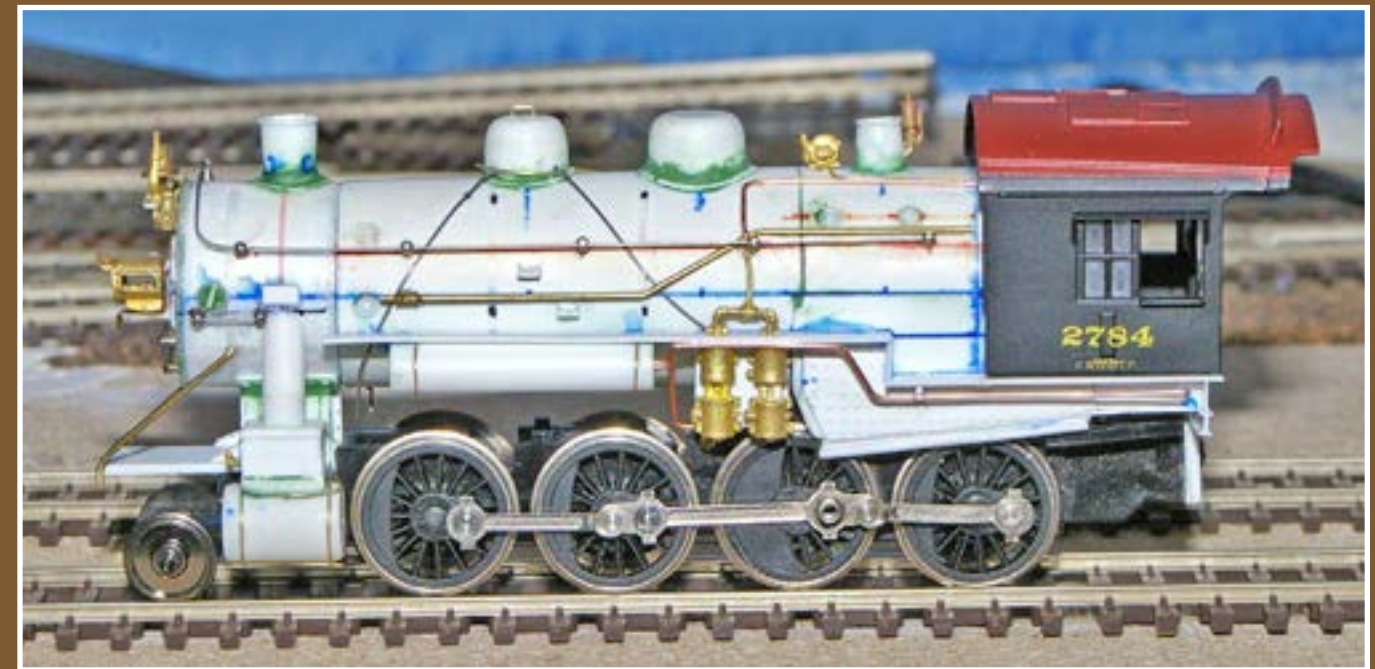
Figure 17: This is the finished fireman's side. You can see the steam and air lines for the compressors.
