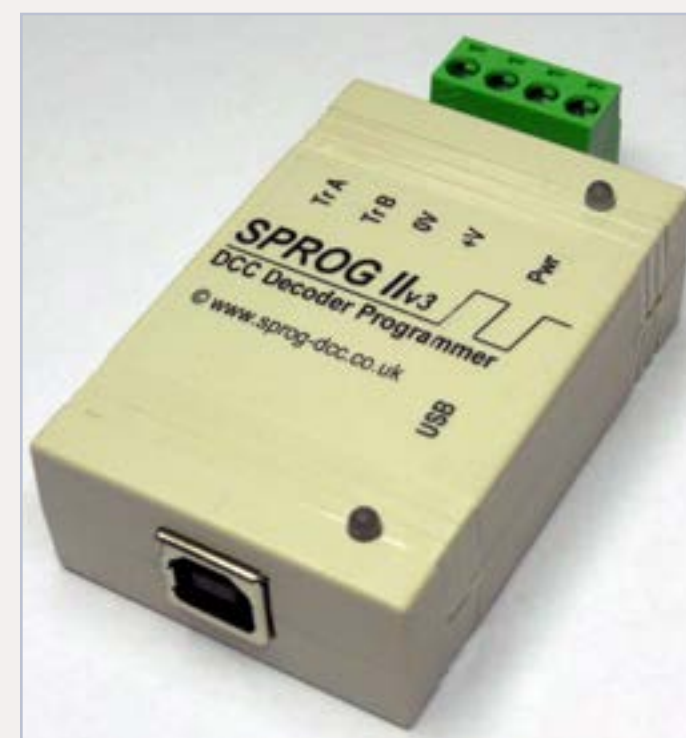
Figure 6: SPROG stand-alone programmer – photo courtesy Andrew Crosland.
