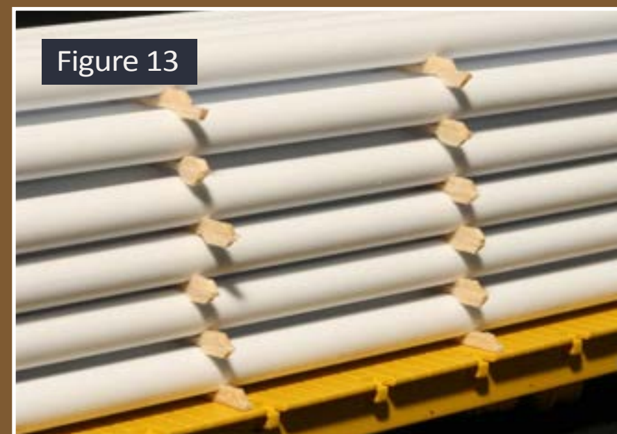
Figure 13: Once all the runners are complete, the individual tiers can be 'test-stacked' to determine if any additional trimming is necessary.
