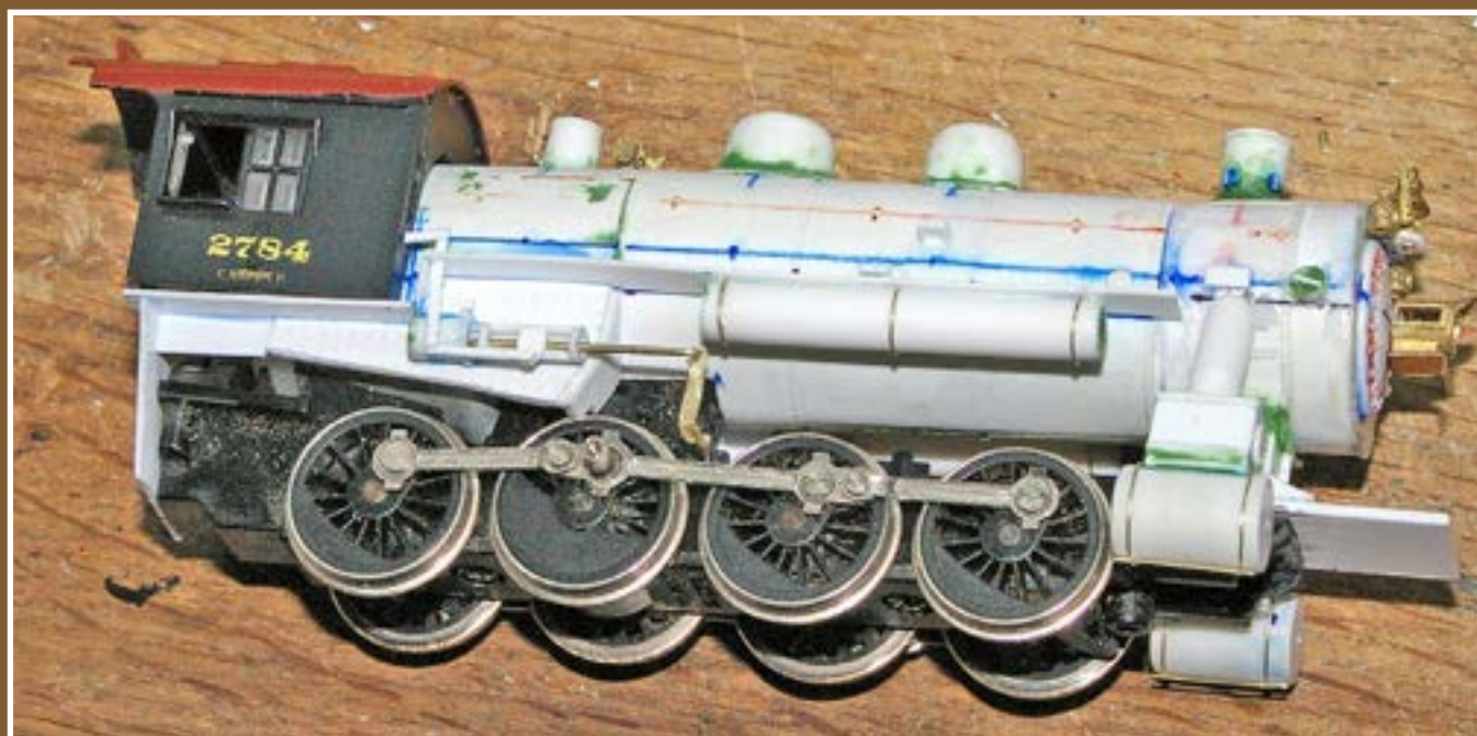
Figure 9: This is the scratchbuilt power reverse, in all its glory. By imagining it as a collection of basic shapes, it's simple enough to build.
