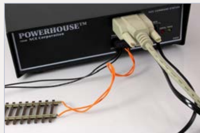
Figure 5: NCE command station with RS232 cable interface.
