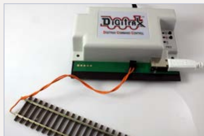
Figure 2: Digitrax PR-3 connected to USB and programming track.
