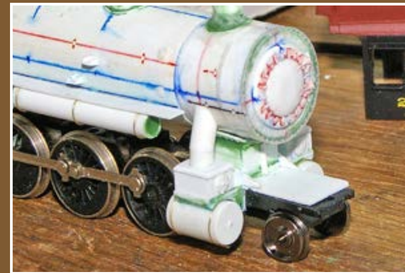
Figure 5: The steps are glued in place. Rather than mark their locations, I simply measured as I glued them in place, making sure to keep them level.
