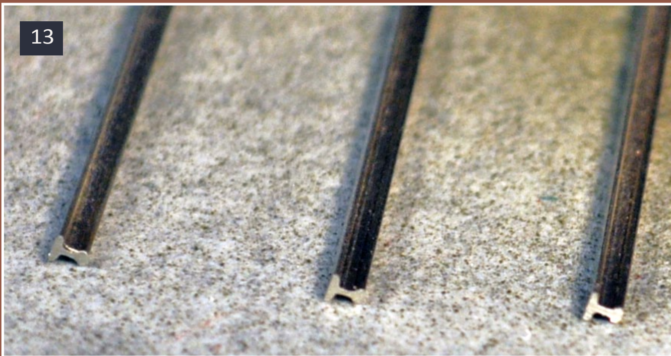
13: I painted the rails on three sides with Floquil Rail Brown. The unpainted ends will butt up to the roundhouse base, and won't be visible. Neither will the unpainted bottom sides, which will be facing down.
