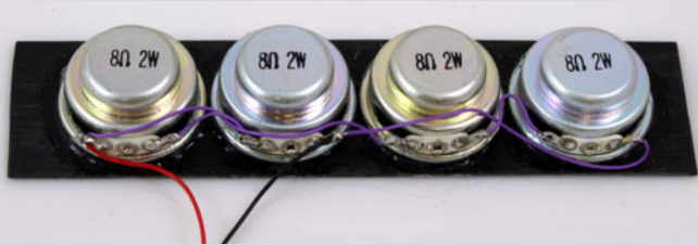
12: A series-parallel wiring of four speakers.
