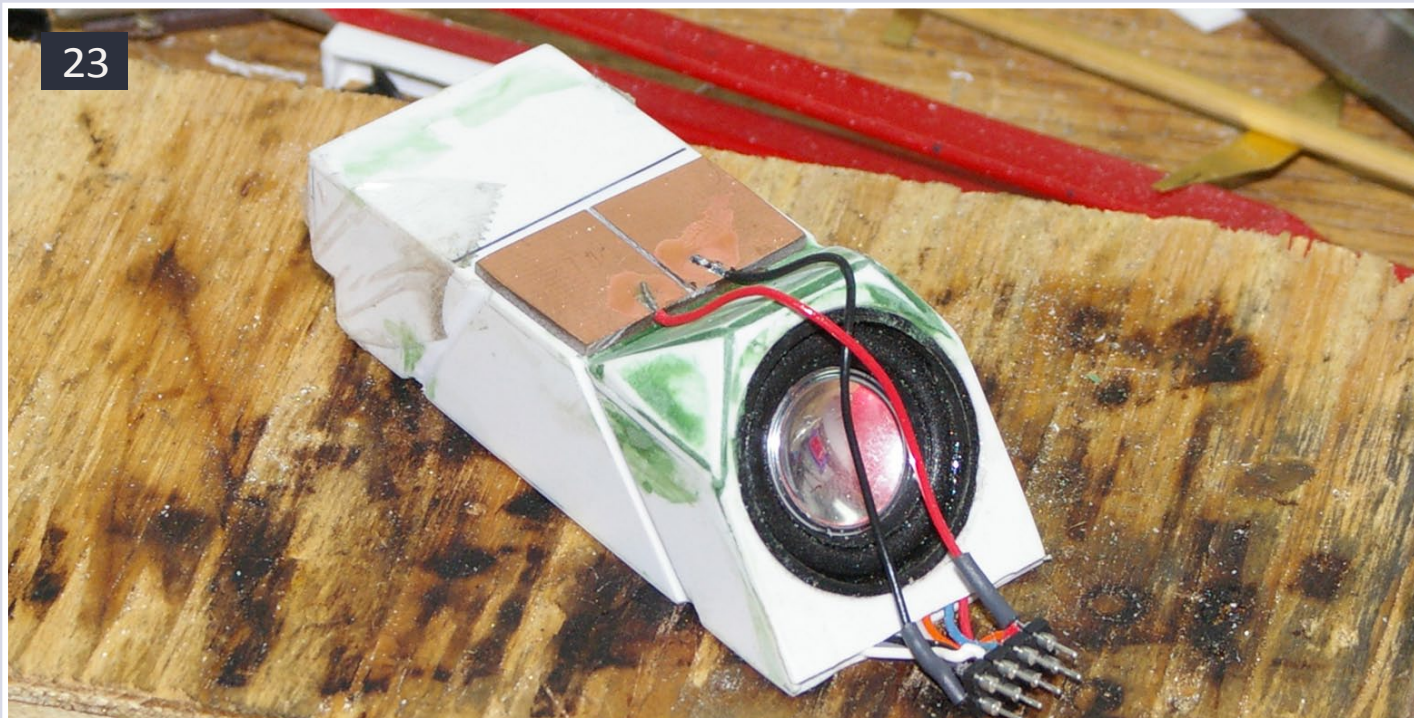
Figure 23: I made the enclosure just as large as I could. In order to fit around the rear tank mount, I notched the bottom and used tape to cover the hole.
