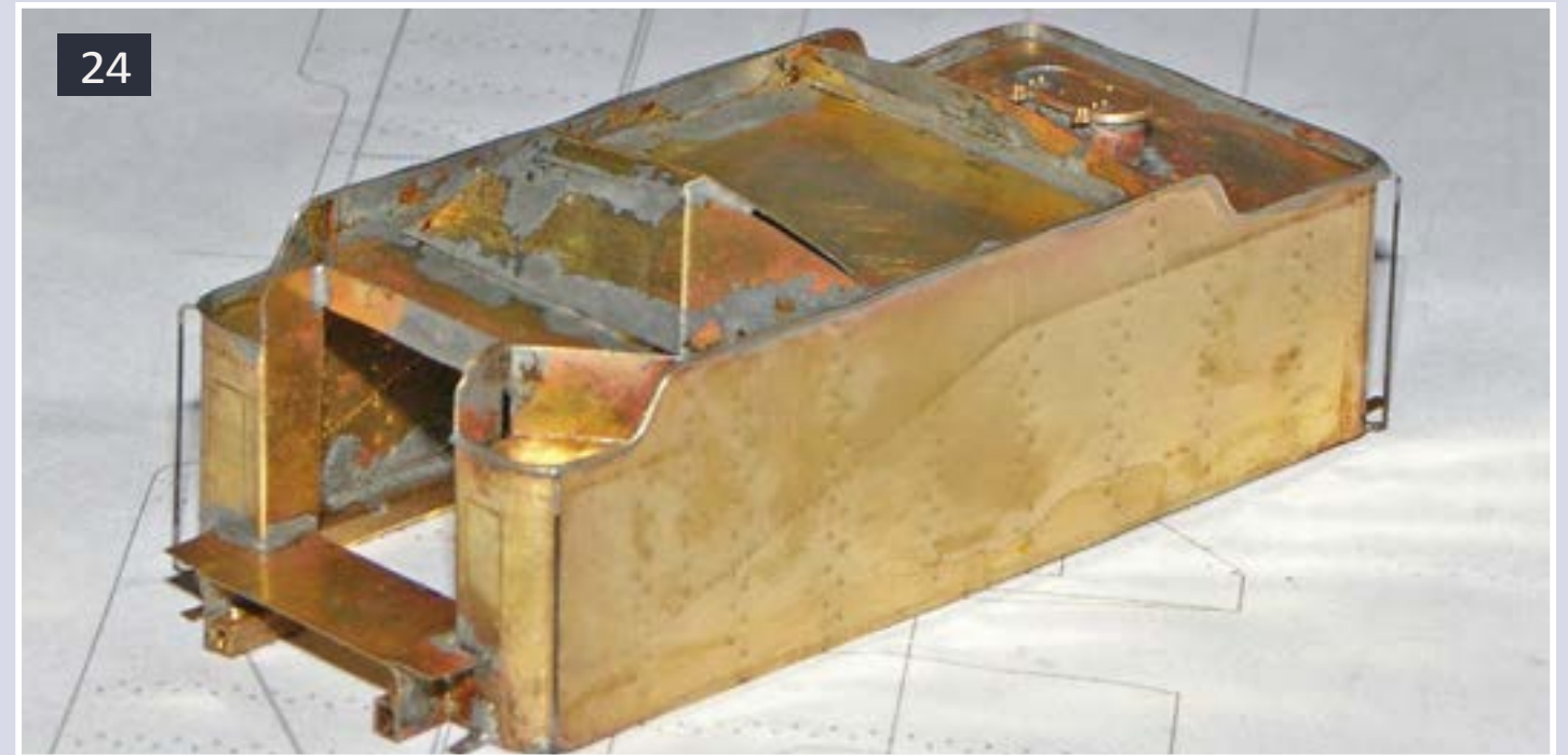
Figure 24: I was having fun with brass at this point, so I made a cover for the enclosure. It's far from perfect, but it won't show, and it was a quick and easy thing to make and solder into place.
