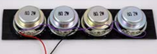
12: A series-parallel wiring of four speakers.
