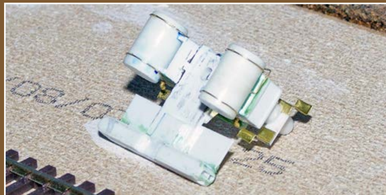
11: The underside of the pilot deck has a pad for mounting the coupler, since I chose to use a regular coupler modified to resemble those on a steam locomotive pilot.
