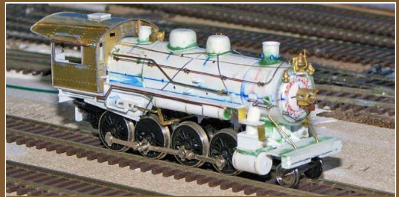
12: Aside from being a way to test the fit of various parts, putting everything together can be a way to keep yourself inspired. It's starting to look like a locomotive!
