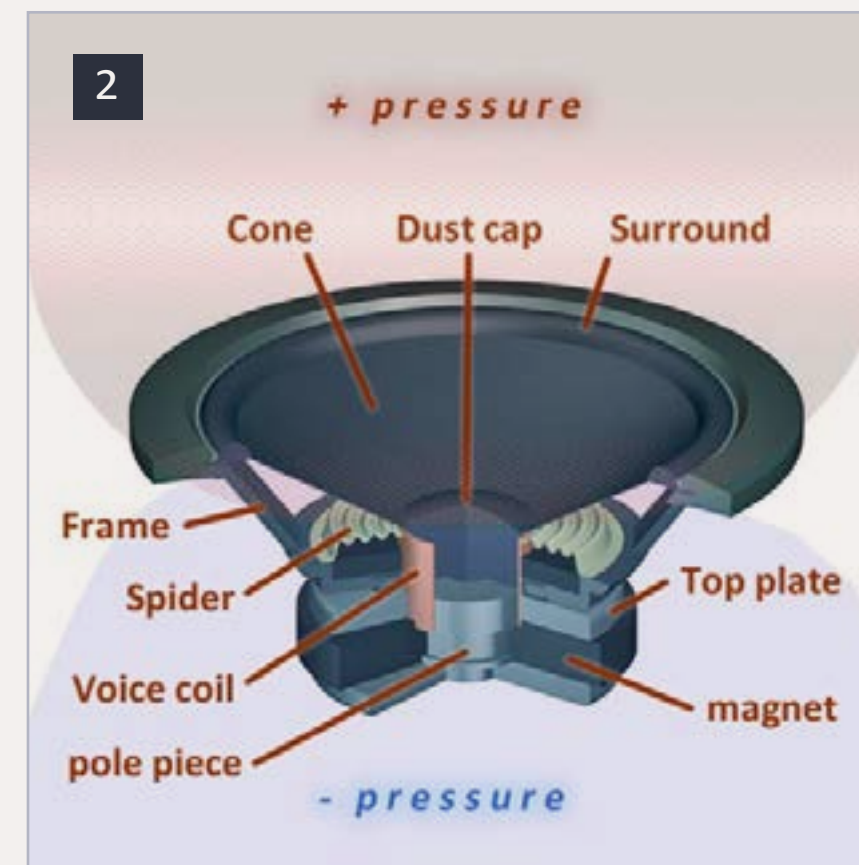
2: Speaker Cross-section with parts labeled – adapted from Wikipedia.
