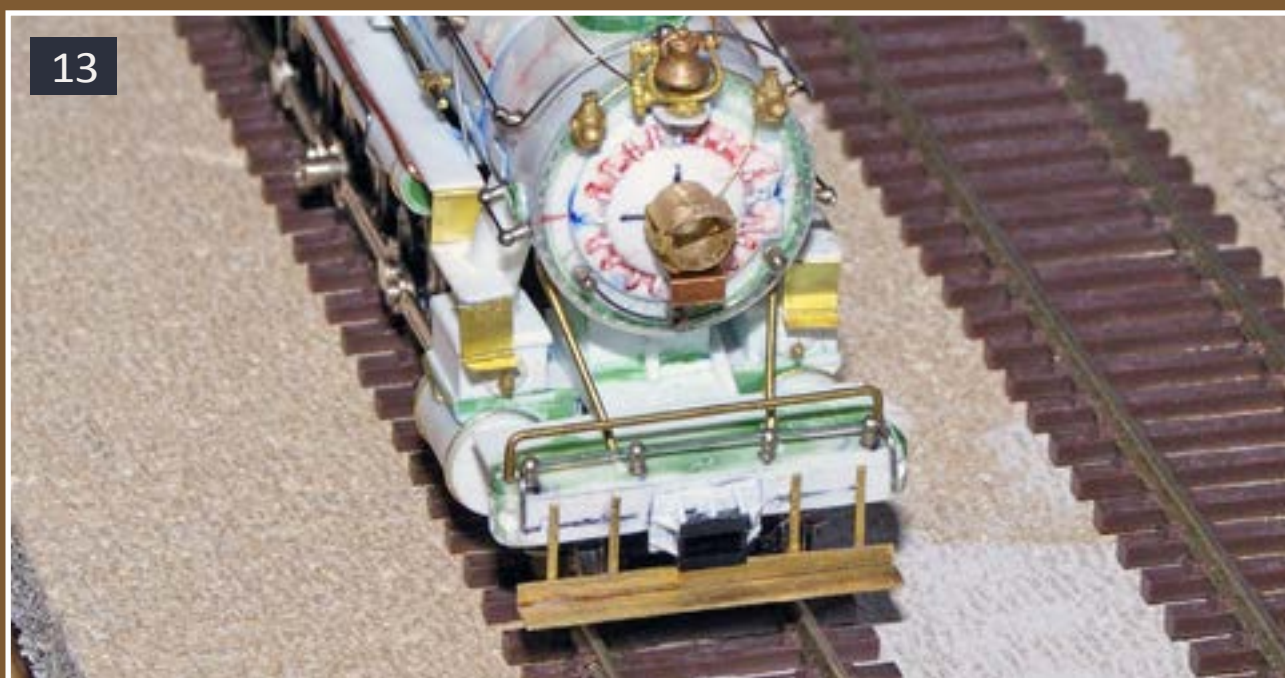
13: With the coupler "casting" built up and the foot boards, cut lever and hand rails in place, the pilot is pretty well finished.
