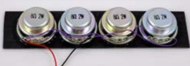
12: A series-parallel wiring of four speakers.
