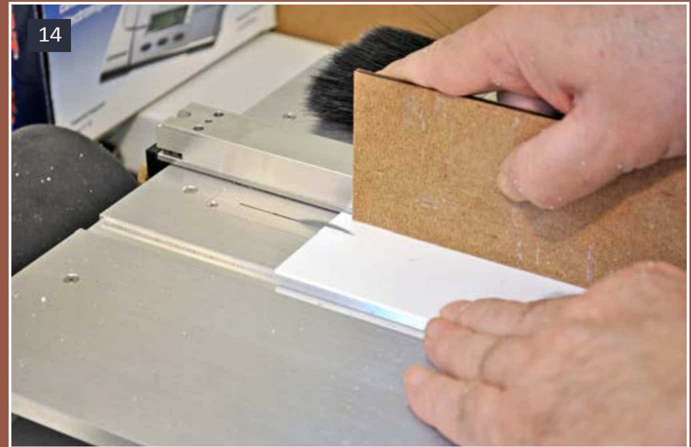
14: Once I figured out the dimensions between the rails, I cut the .040" styrene pieces.
