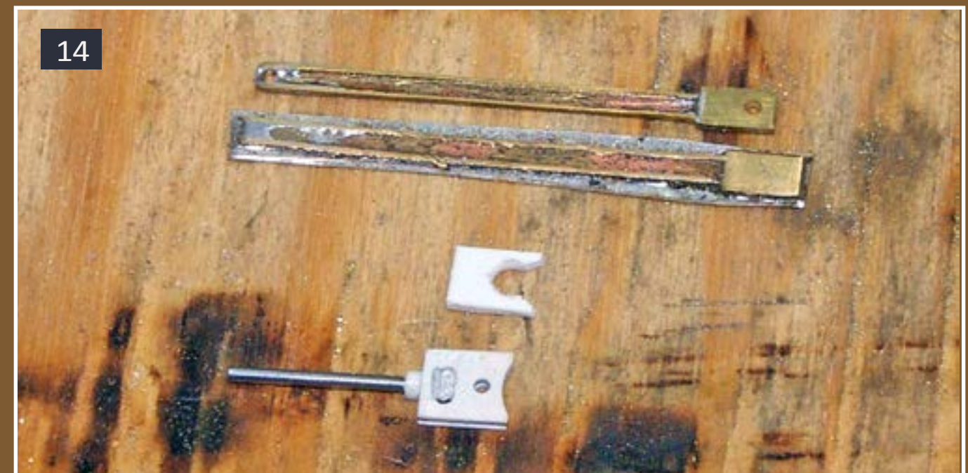
14: The crossheads and rods are built up in layers. Here you can see one of each finished along with some of the pieces that went into it.
