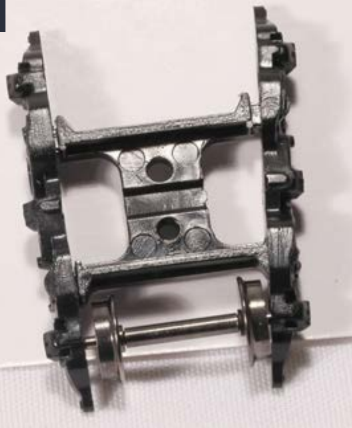
3: Spread the truck frame sides to insert Intermountain metal wheel sets.
