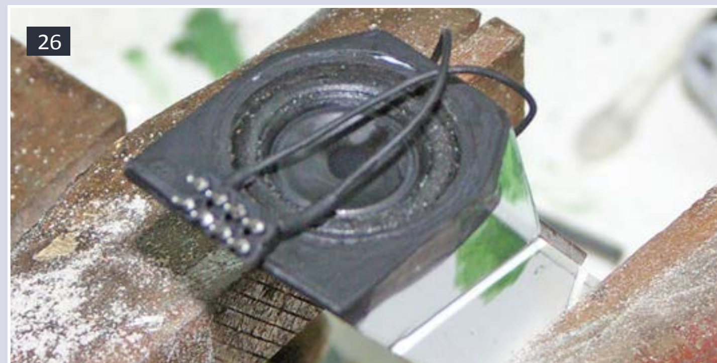
Figure 26: I painted everything flat black to hide it inside the finished model. Only the front face needs paint, of course.
