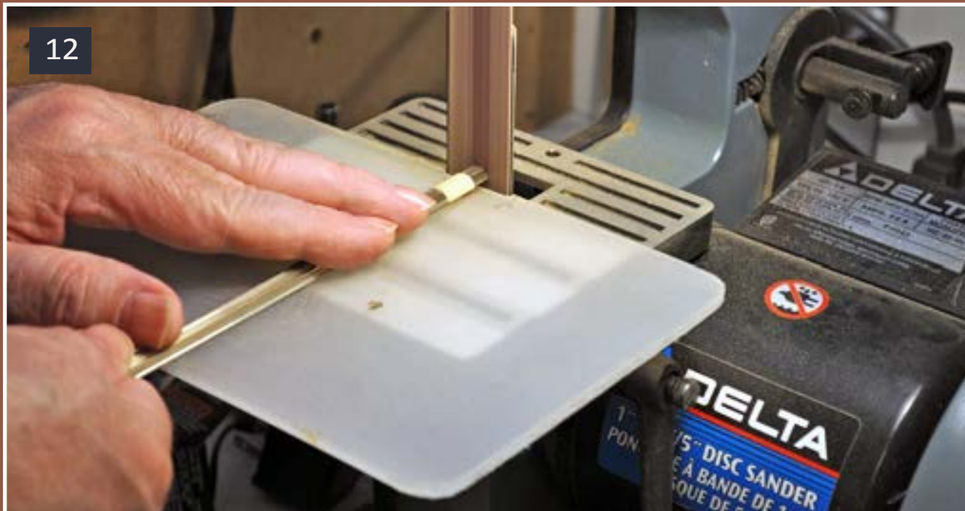
12: I taped the rails together and ground the ends to even up and to remove any burrs.
