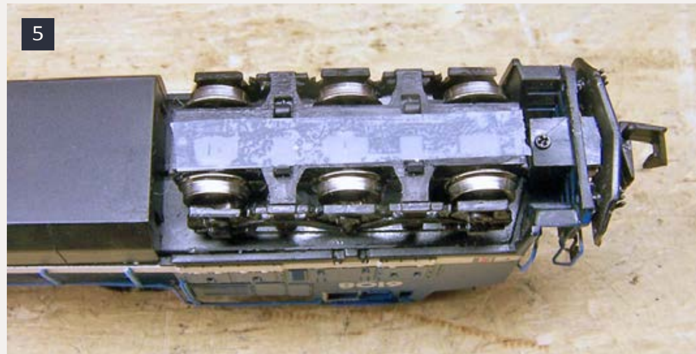
5: A strip of clear Scotch tape keeps layout clag away from locomotive power truck gears and the sticky surface corrals fine particles of grit. Photo by Andrew Kyle.
