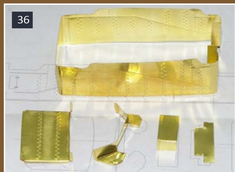
36: The tender tank parts are cut out and folded up, like brass origami. A few bends makes them surprisingly strong.
