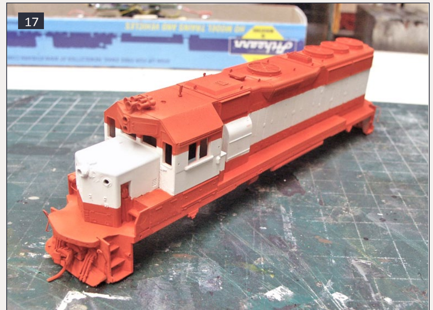
Figure 17: Loco shell after spray painting the Frisco Mandarin Orange (see text for exact color source) and removing the tape masking.
