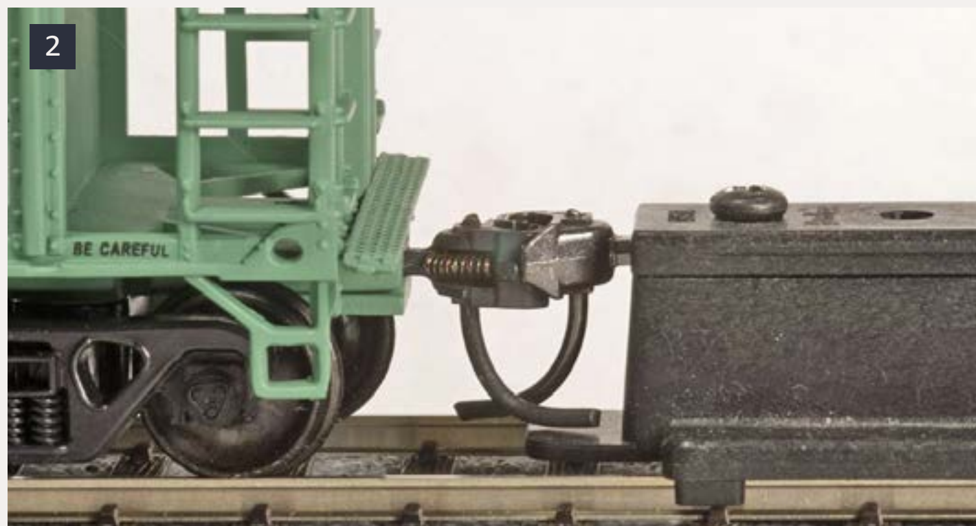
2: A properly mounted coupler's knuckle matches exactly with the height gauge, and there is a gap visible between the bottom of the iron wire trip pin and the foot plate on the gauge, indicating sufficient clearance.
