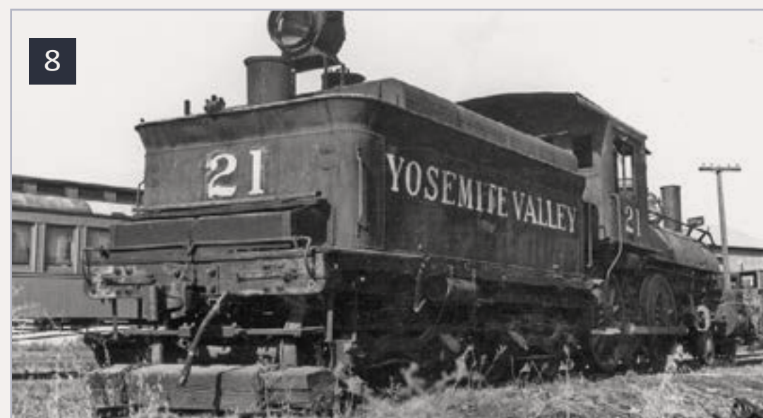
8: The end of the turntable lead next to the Carpenter Shop had another interesting detail which is easy to duplicate. The bumper on this track consists of an old tie chained in place. The photo of the No. 28 is on this same track (Figure 6) and was taken in 1934 and shows the tie on top of the rails. This photo of the out-of-service No. 21 was taken in 1942. By then the bumper had been pushed off of the rails. – Photo by Bob Lunoe
