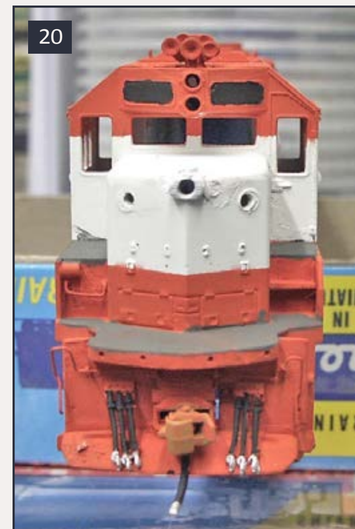
19: Front of the loco before hand-painting of details.
