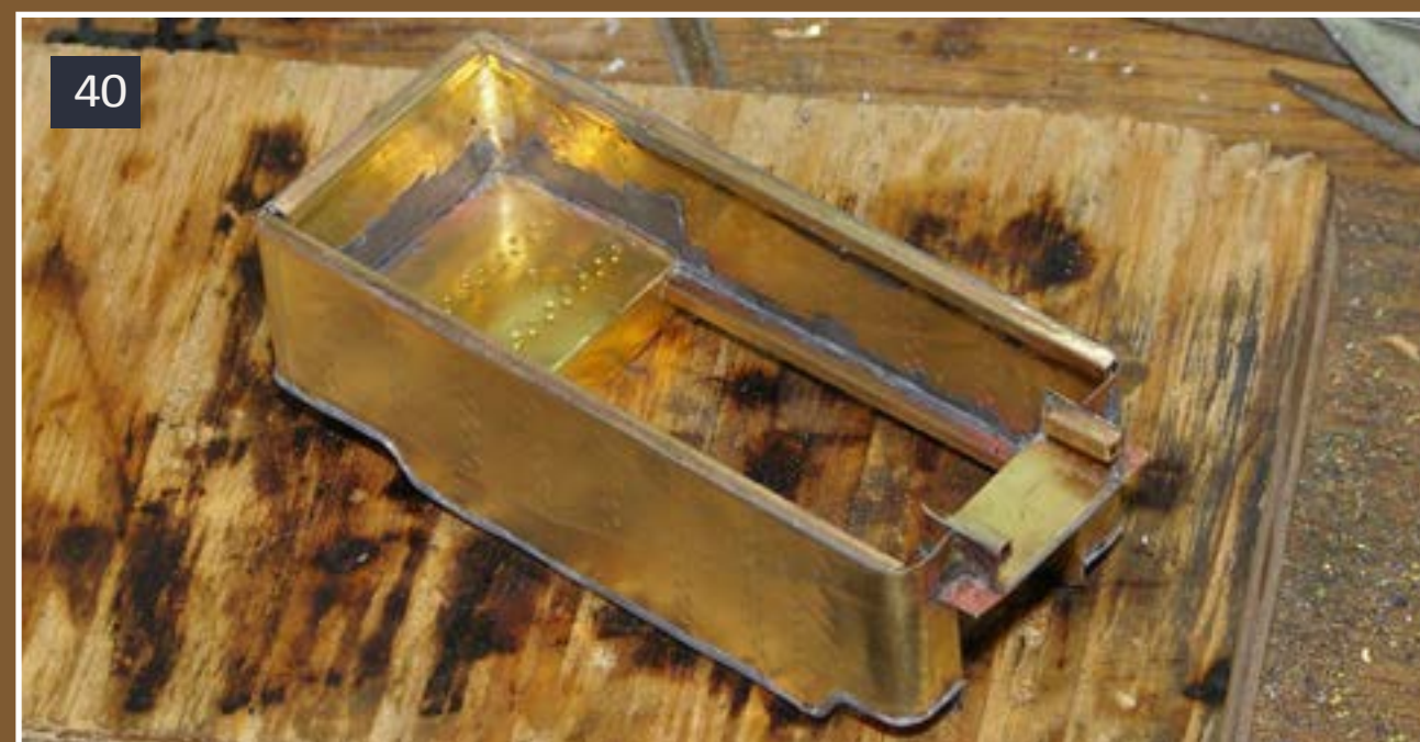
40. Square tubes make the bottom of the tank more rigid, and provide a mounting point to connect the tank and frame.
