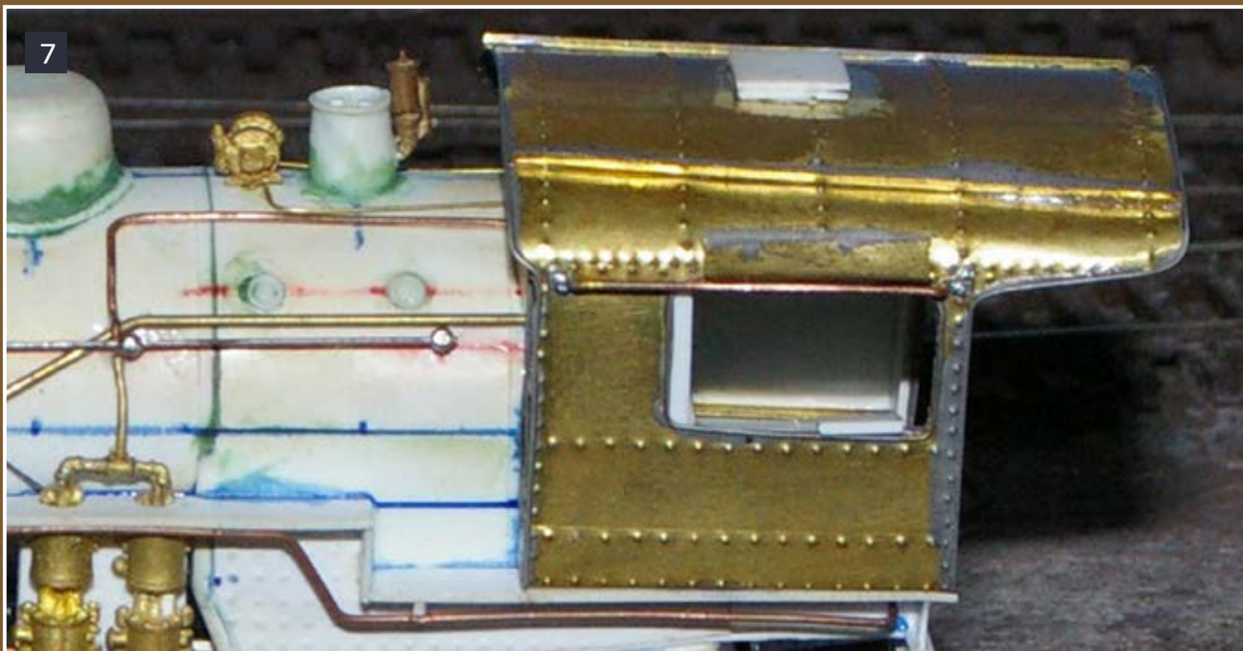
7: The drip rails are angled down toward the rear, to help channel rain away from the doors and windows. On the model, they're just soldered into place, positioned by eye.
