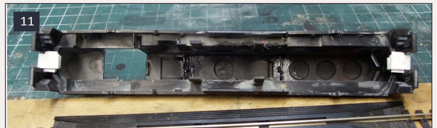
11: Loco shell, with the new styrene coupler pads to allow body-mounting the couplers.
