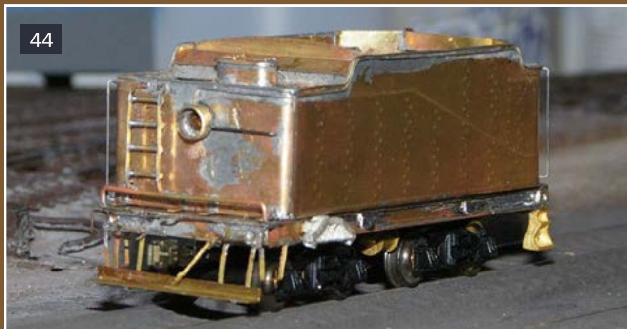
44. I chose a brass air hose on the rear, for added strength. All the details are in place at this point.
