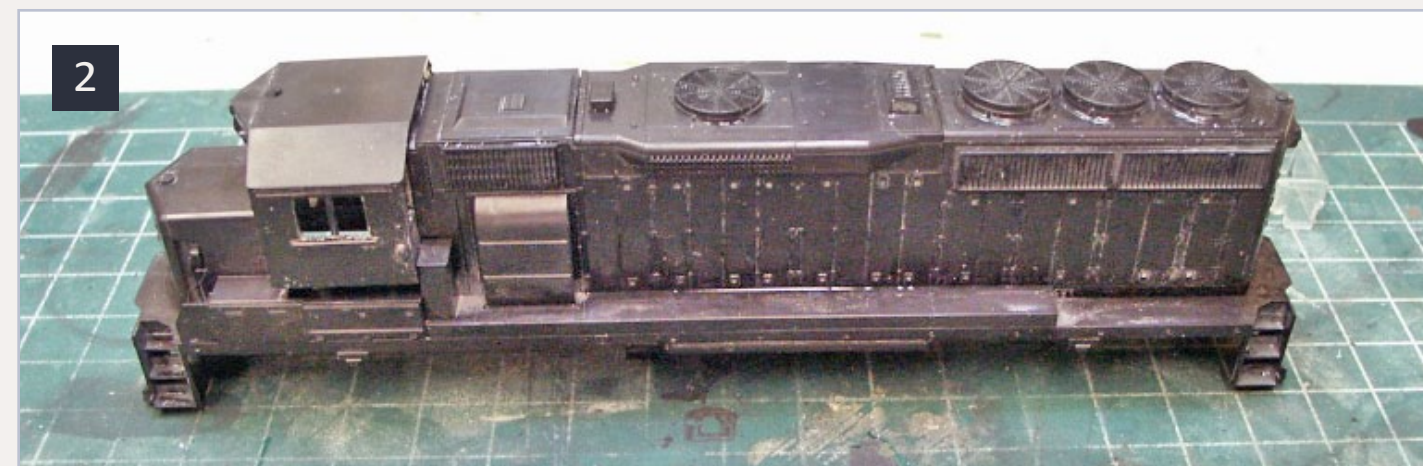
2: The SP GP40-2 shell with paint completely stripped using Castrol Degreaser.
