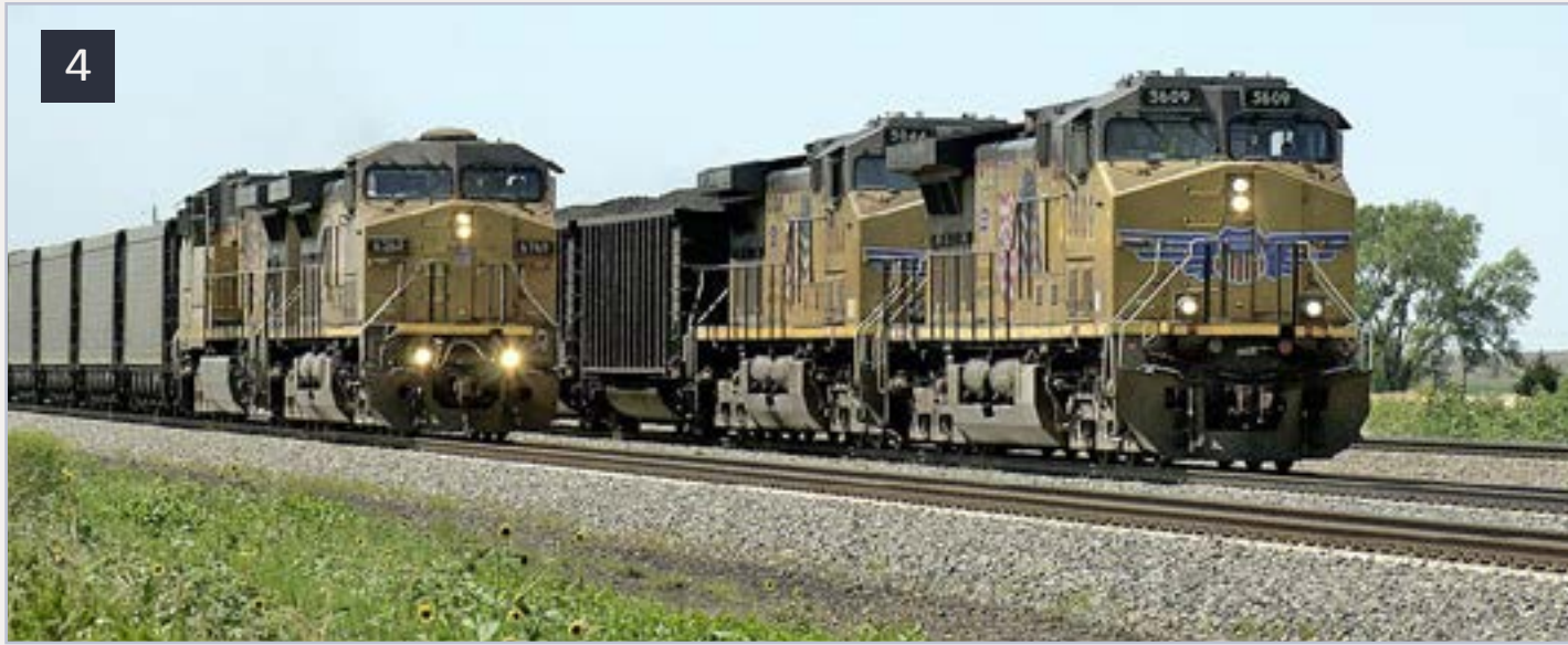
4: Two loaded Union Pacific coal trains, rolling east on the triple track mainline east of North Platte, Neb., clearly show the high-visibility triangular pattern formed by the locomotives' headlights and ditch lights. Photo by Graham Line.
