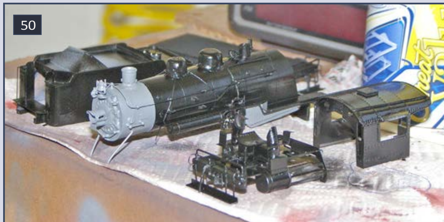
50: Removing the tape shows a nice clean separation, with no touch-up needed.
