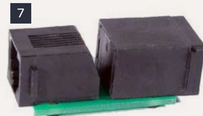
7: UTP-Cat5 adapter from NCE – photo courtesy NCE.
