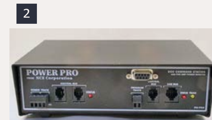
2: NCE's five-amp system box.
