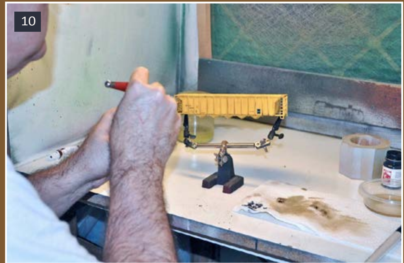
10: Always use a spray booth with an exhaust fan to avoid breathing paint and thinner fumes.
