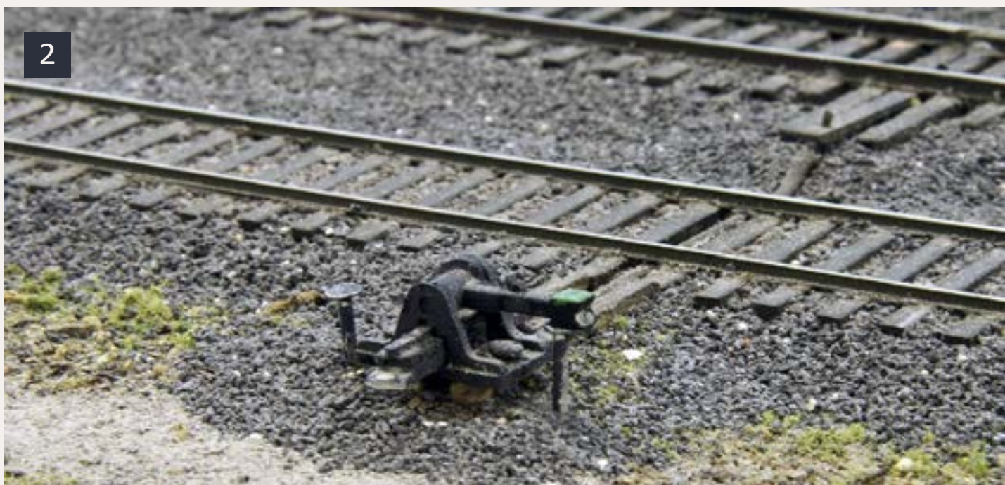
2: Caboose Industries ground throws are very reliable when installed following the package directions. This throw has a remote linkage to control a track often obscured by other traffic.
