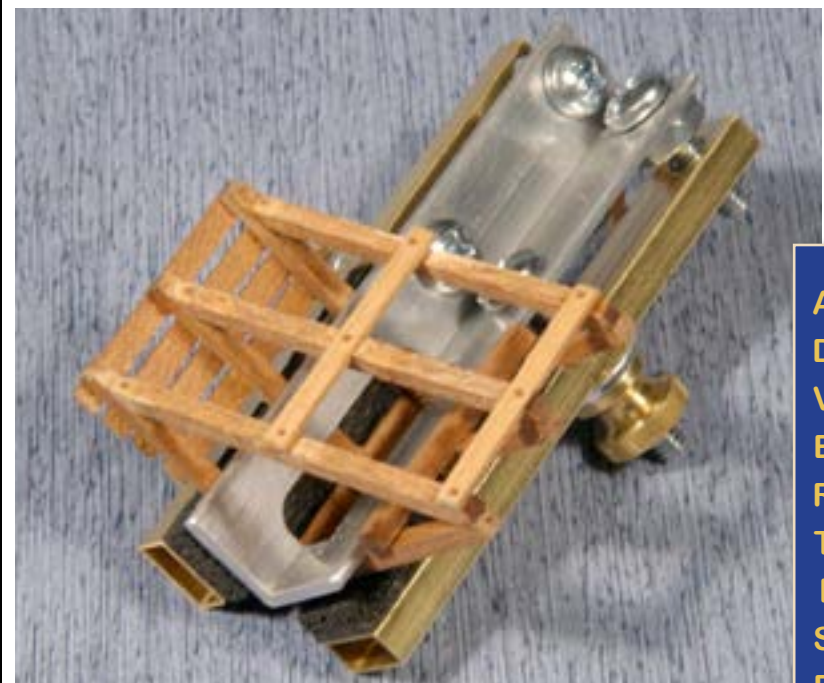
AC-1-1 "Original Right Clamp"™ used for Bulkhead Assembly.
