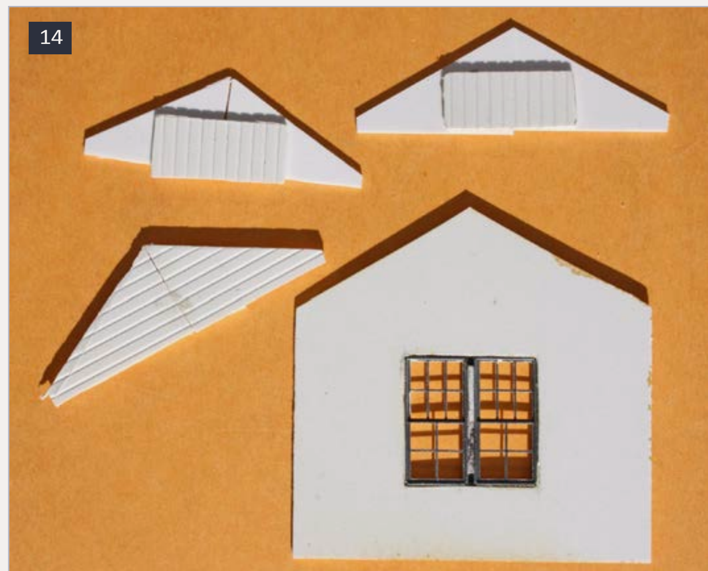
14: Internal roof braces or “formers” were made from the trim pieces above each depot end, plus one made from an interior wall piece, which need not extend above ceiling height. Scrap pieces of styrene splice the halves. An end wall piece is included to demonstrate the common roof angle.
