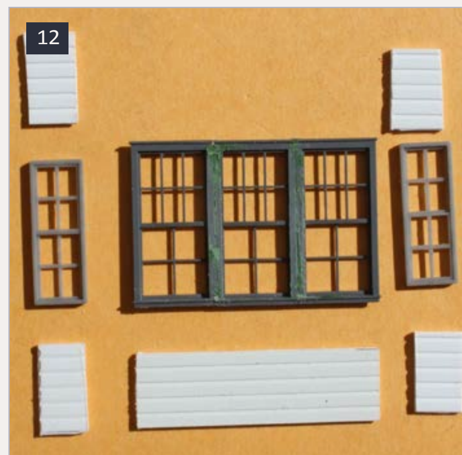
12: All parts of the bay window section of the front wall are here, except the front wall above the windows. The triple-window assembly sets the width of the front wall, and the narrow side windows set the side-wall width. Some minor discrepancies in window dimensions will be concealed when trim boards are attached.
