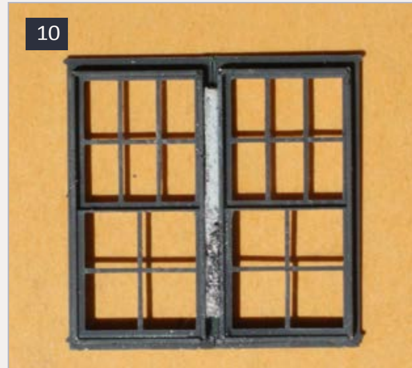
10: The pair of windows in the end wall of the waiting room was glued together with a styrene strip between the two of them, as seen here from the back. The sill and top trim on the mating side edges of the windows were sanded flat before combining them.
