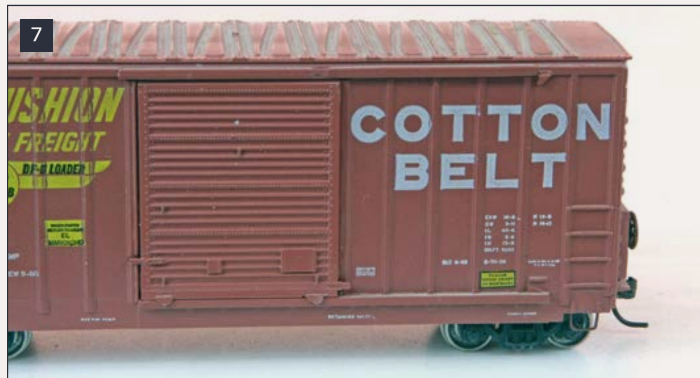
7: Replacing this car's bulky steps with A-Line metal stirrup steps and carving down the bottom runner "door claws" (and gluing the door in place) updates this car's first-glance appearance with only a bit of effort. Once weathered appropriately, this car will blend right in with the more finely-detailed equipment in your roster.
