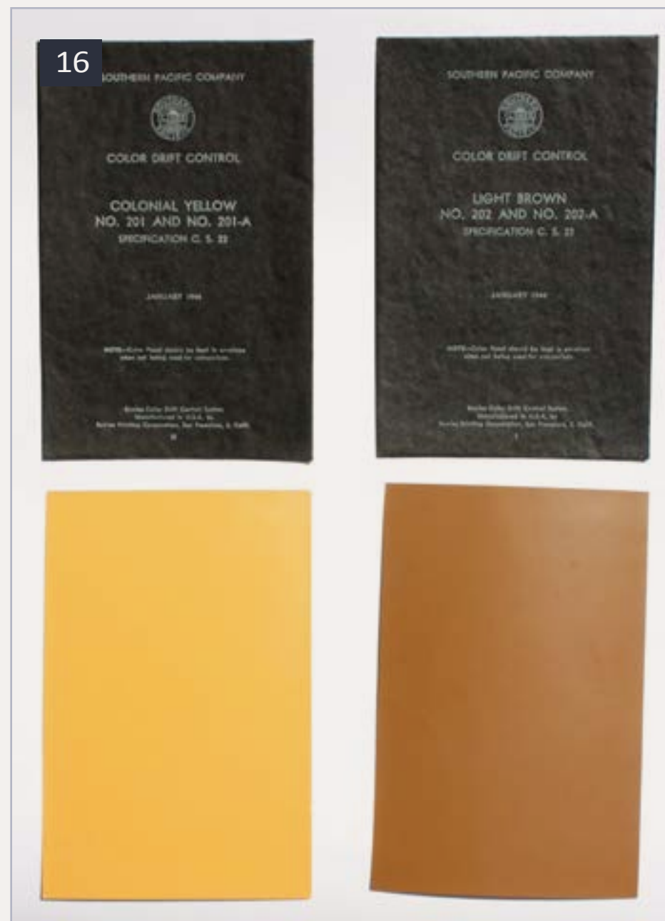
16: Envelopes for Common Standard colors no. 201, Colonial Yellow, and no. 202, Light Brown, alongside the color drift cards, from the 1944 issue of these cards. The Bowles Printing Company of San Francisco issued these for Southern Pacific for decades, some as late as the 1980s.
