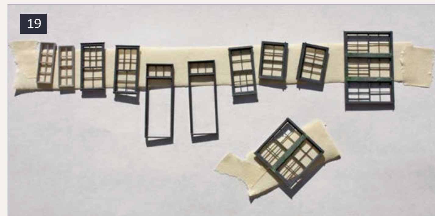
19: All windows, window assemblies, and door frames are shown here, on strips of tape (sticky side up), ready for airbrushing white. Only the door transom would have the white mullions, so the door itself is not painted white.
