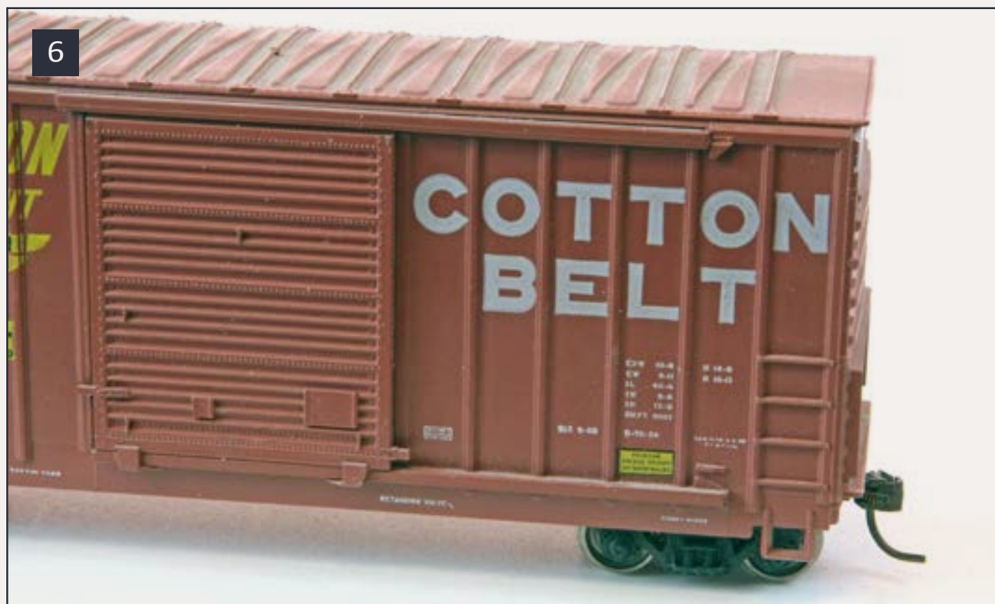
6: Bulky stirrup steps and the huge "door claws" on this 40-foot hi-cube Athearn Blue Box car clearly give away the car's less expensive heritage. While you can find these cars for good prices, no amount of weathering will hide the trainset-level bulky details.
