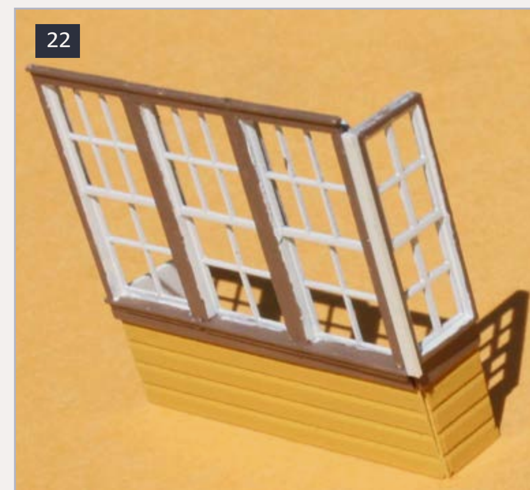
22: In this view, one side window has been glued to the bottom section, and a corner filler strip (white) of scale 2 x 4-inch styrene has been added. The filler strip will be painted brown. Trim strips below the two types of windows are 1 x 4-inch and 1 x 8-inch widths, which match up along their lower edge.
