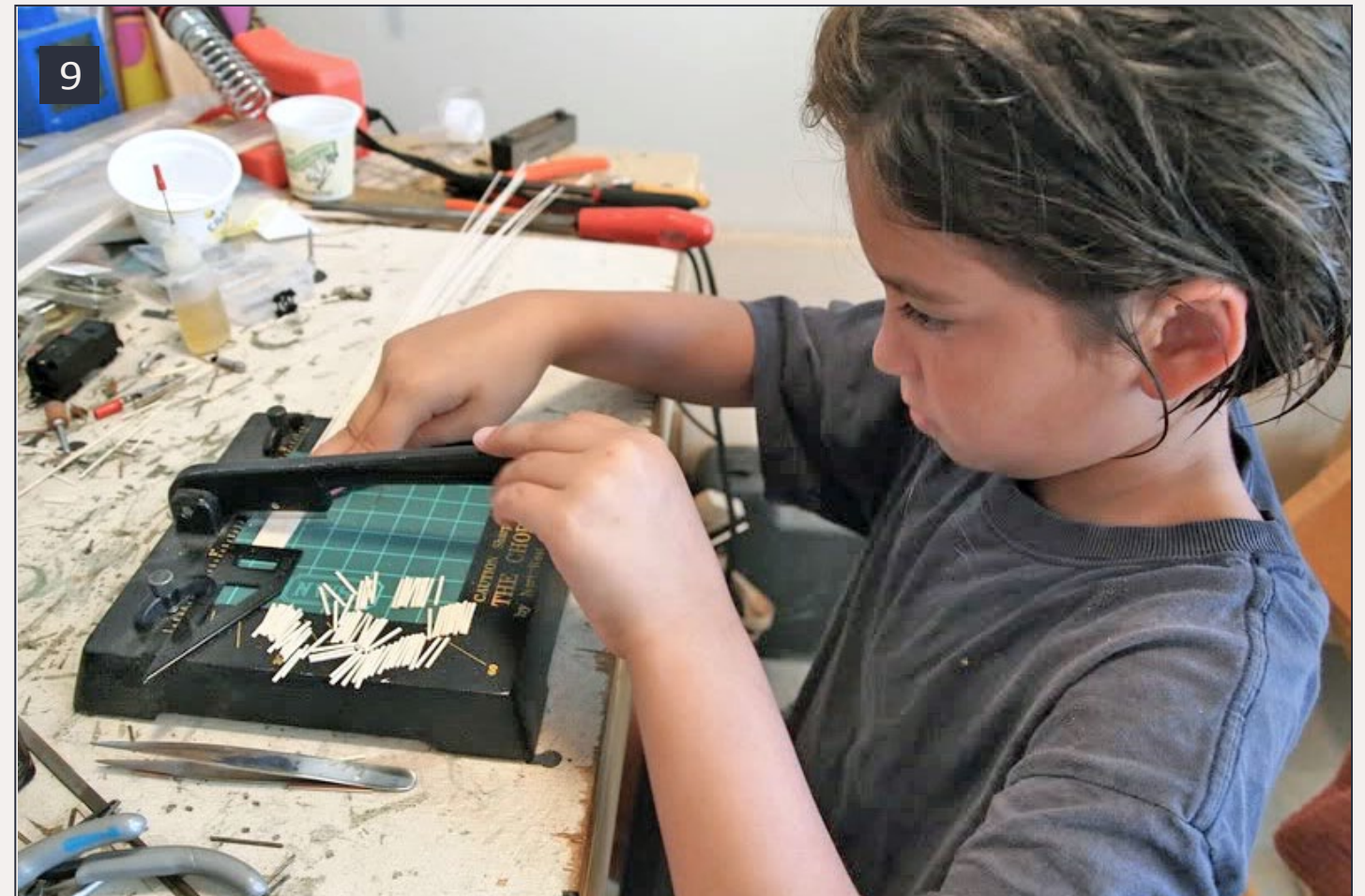
9: My daughter helps me cut replacement ties using our NWSL Chopper II. Busy hands are happy hands!
