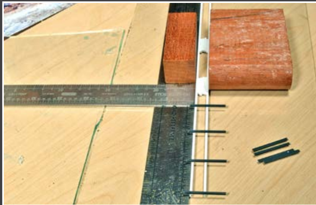
6: Using scale rulers in this way, helps to get exact measurements.
