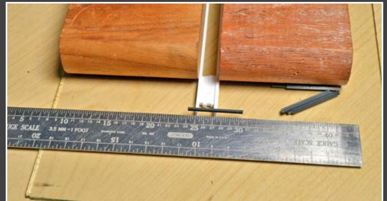
5: A plate glass base helps to keep the I-beams perfectly flat.
