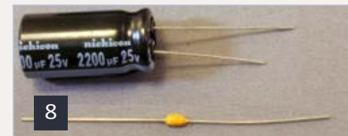
8: Capacitors: top: electrolytic – 2,200 \mu\text{F} at 25 volts bottom: ceramic – 0.1 \mu\text{F} at 50 volts
