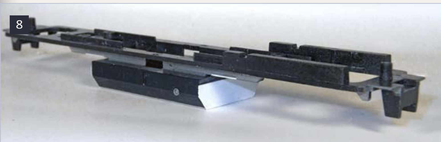
8: Brian Banna's chassis modifications include permanently mounting the fuel tank to the chassis after removing the cast-on air tanks, and drilling holes in the bottom to permit access to the motor mounting screws. He applied new ends and fuel gauges to the tank, and milled the frame rails. Most of this is similar to changes I made on my U18B that was featured in Model Railroad Hobbyist in July 2010.
