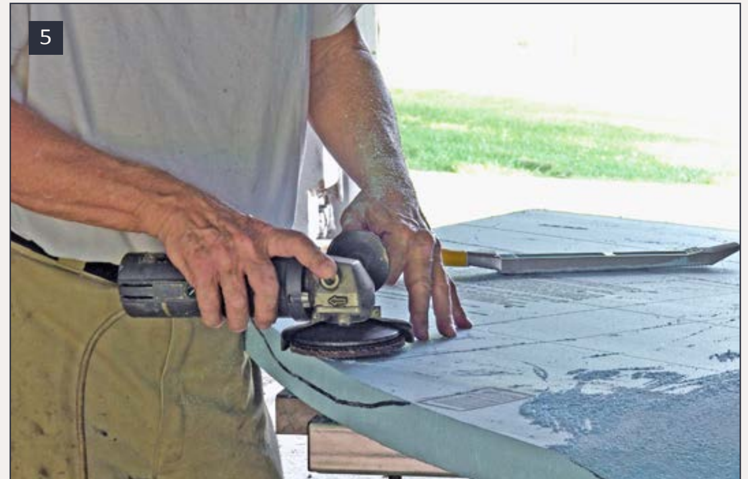
5: Using the sanding disk to rough-carve terrain undulations into Styrofoam board.
