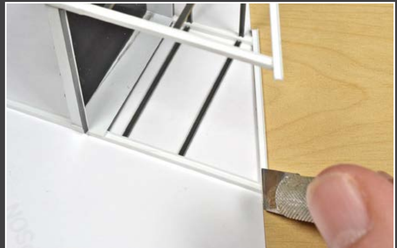
28: Cutting an angle at the top of each vertical I-beam.
