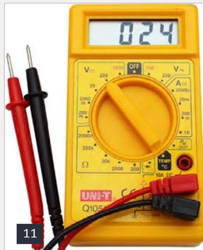
11: Digital Multimeter – photo courtesy of Litchfield Station.
