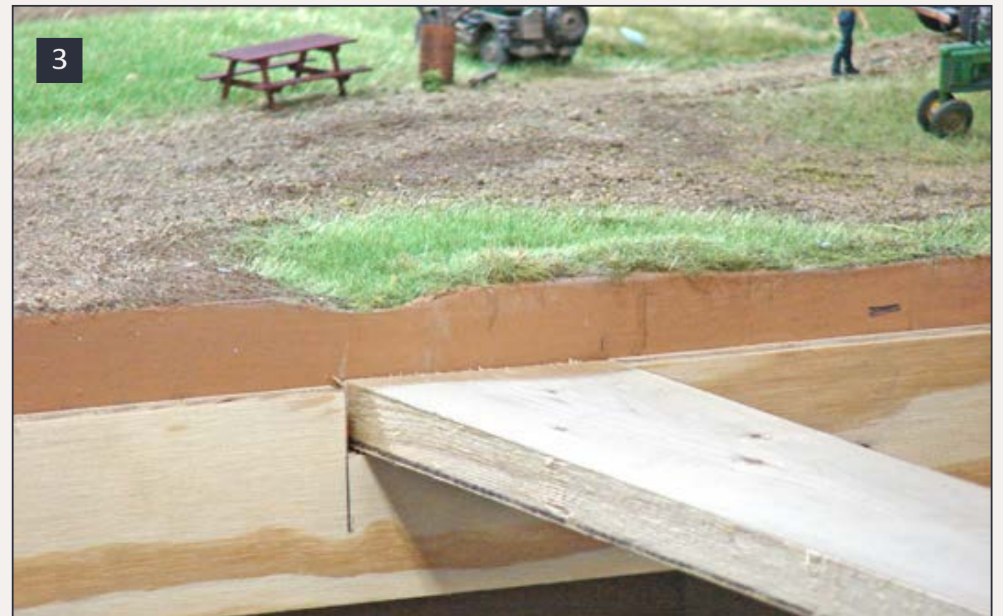
3: Adding notches into the plywood frame to hold the 1x4 support stringers.
