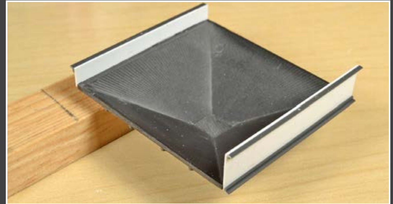
26: Constructing the receiving bin.
