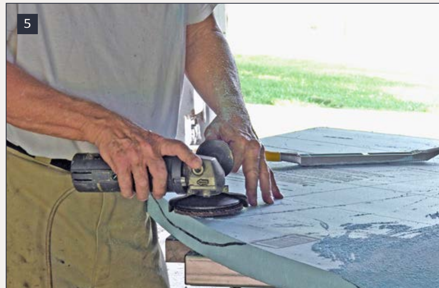
5: Using the sanding disk to rough-carve terrain undulations into Styrofoam board.
