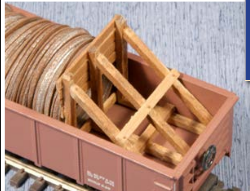
Assembled Bulkhead in gondola with load of ring castings.
