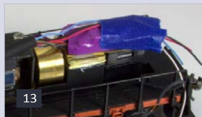
13: The same Atlas S-1 with the decoder installed and partially wired – blue tape holds the headlight wires out of the way.
