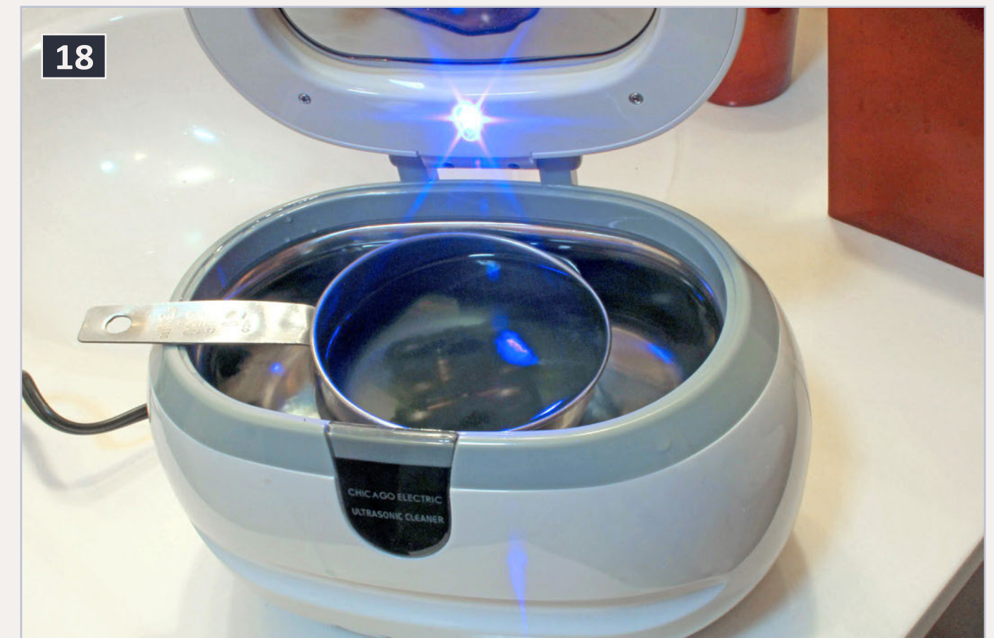
18: Cleaning drive train parts in ultrasonic cleaner.
