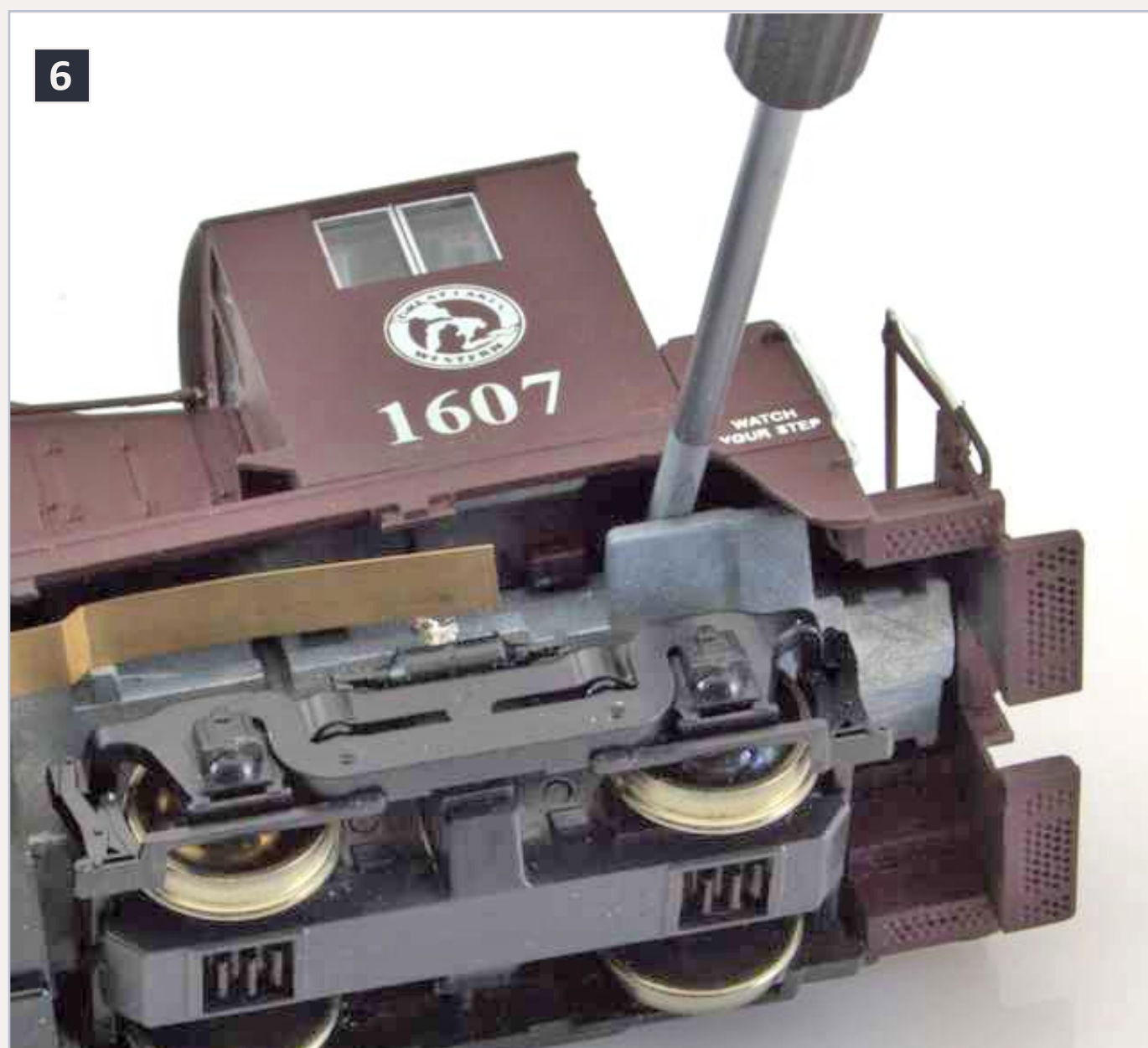
6: Prying the shell off the frame.
