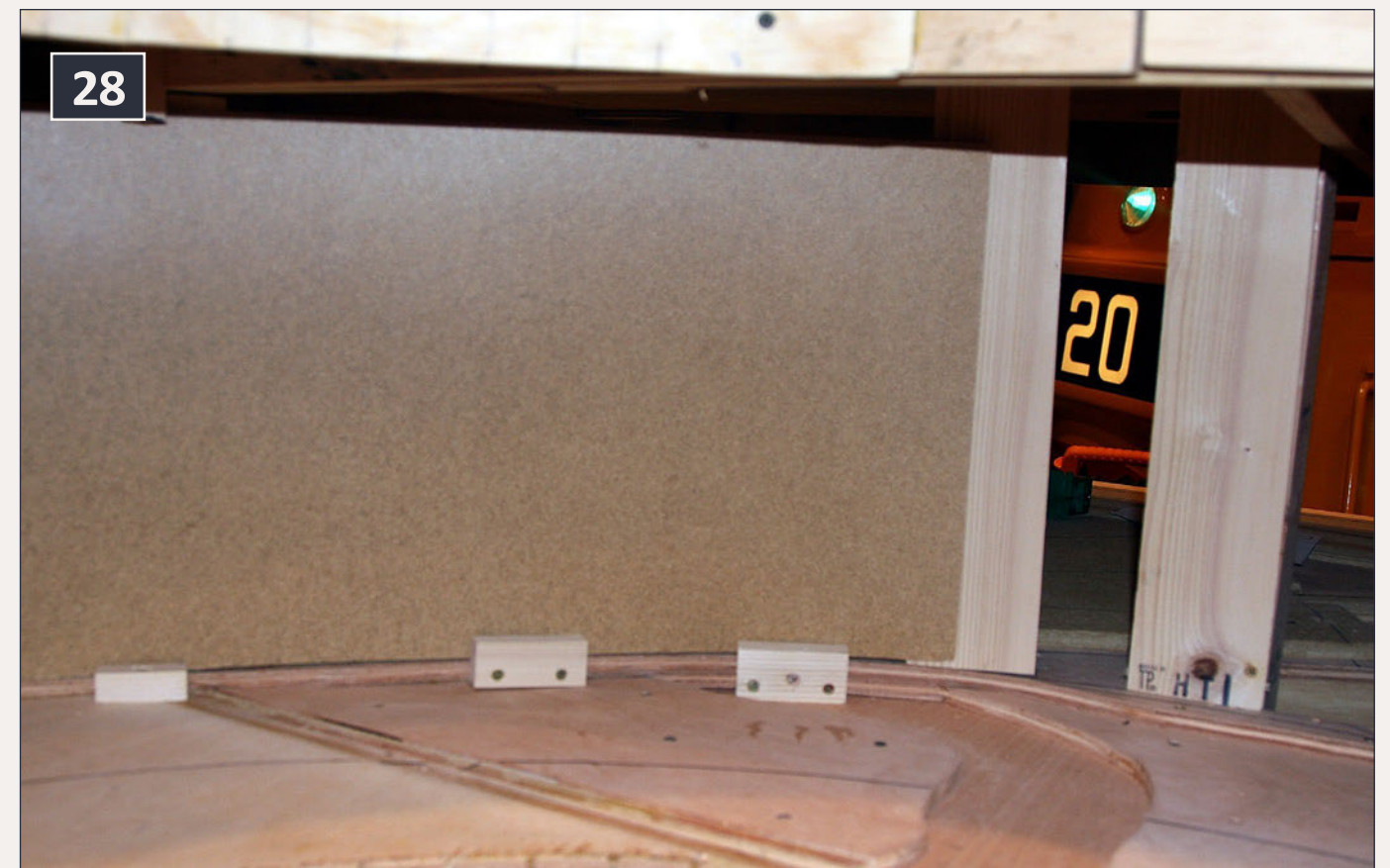
28: Backdrop supports at bottom and behind joint.
