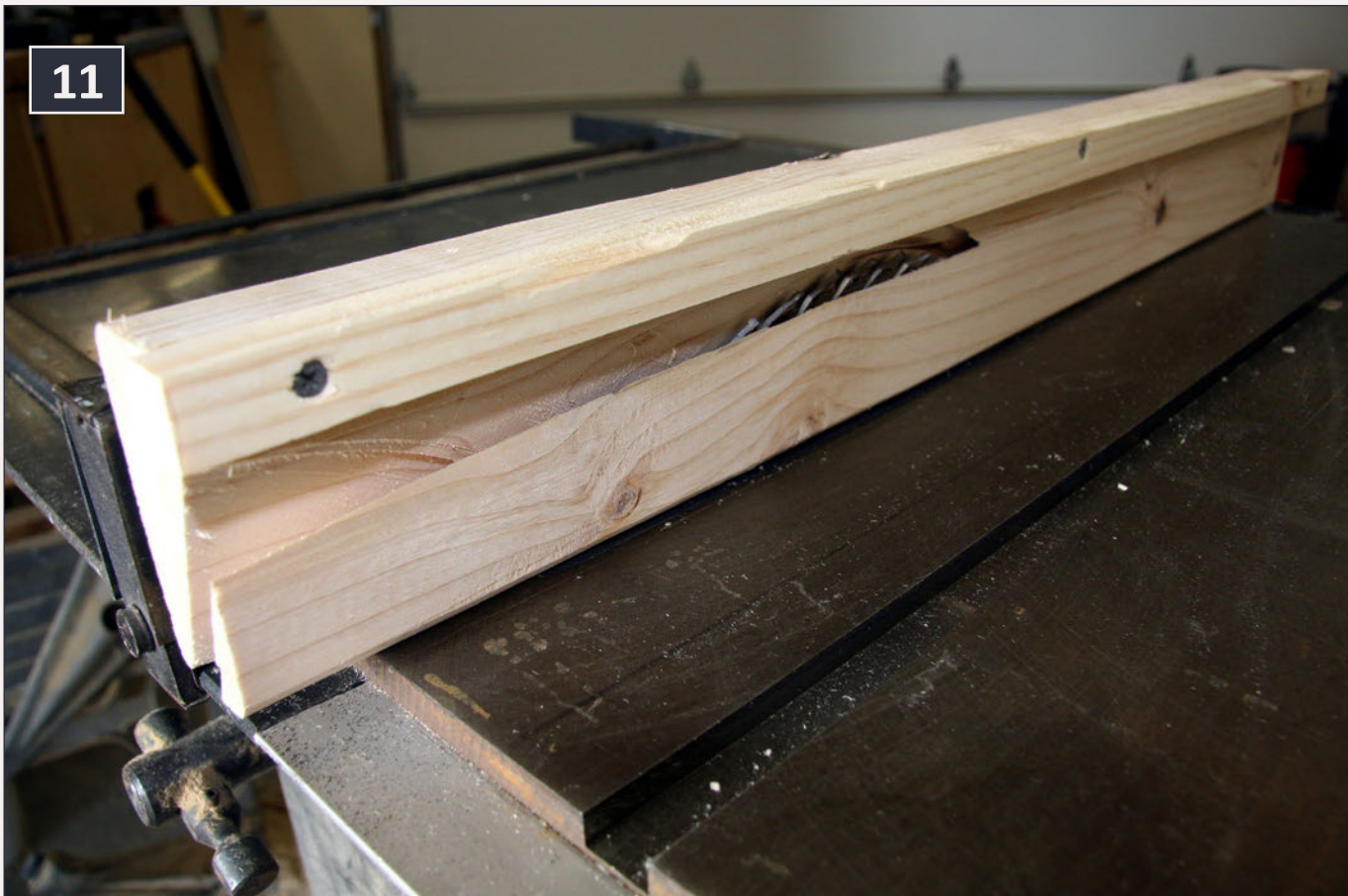
11: Jig for cutting roadbed.
