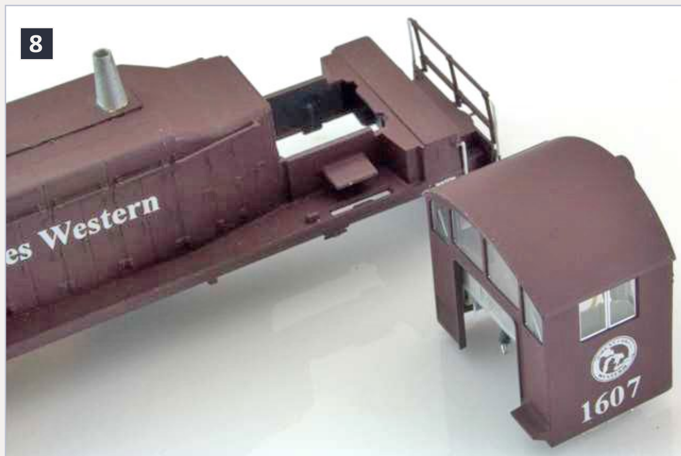
8: Cab separated from shell.
