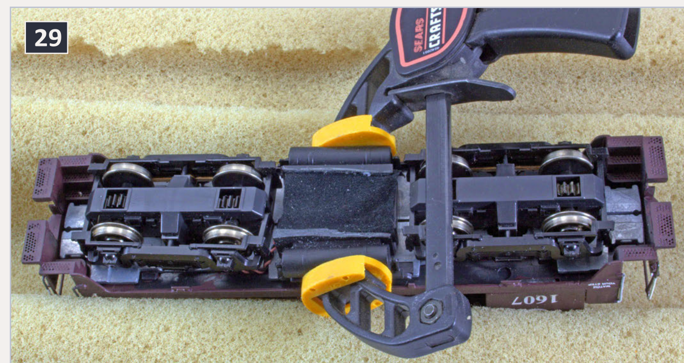
29: Finish the fuel tank with speaker grille cloth and modified plastic parts.
