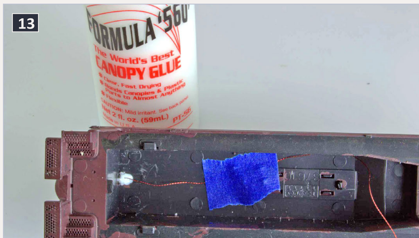
13: Front SMD LED held in place with blue tape while Canopy Glue dries.
