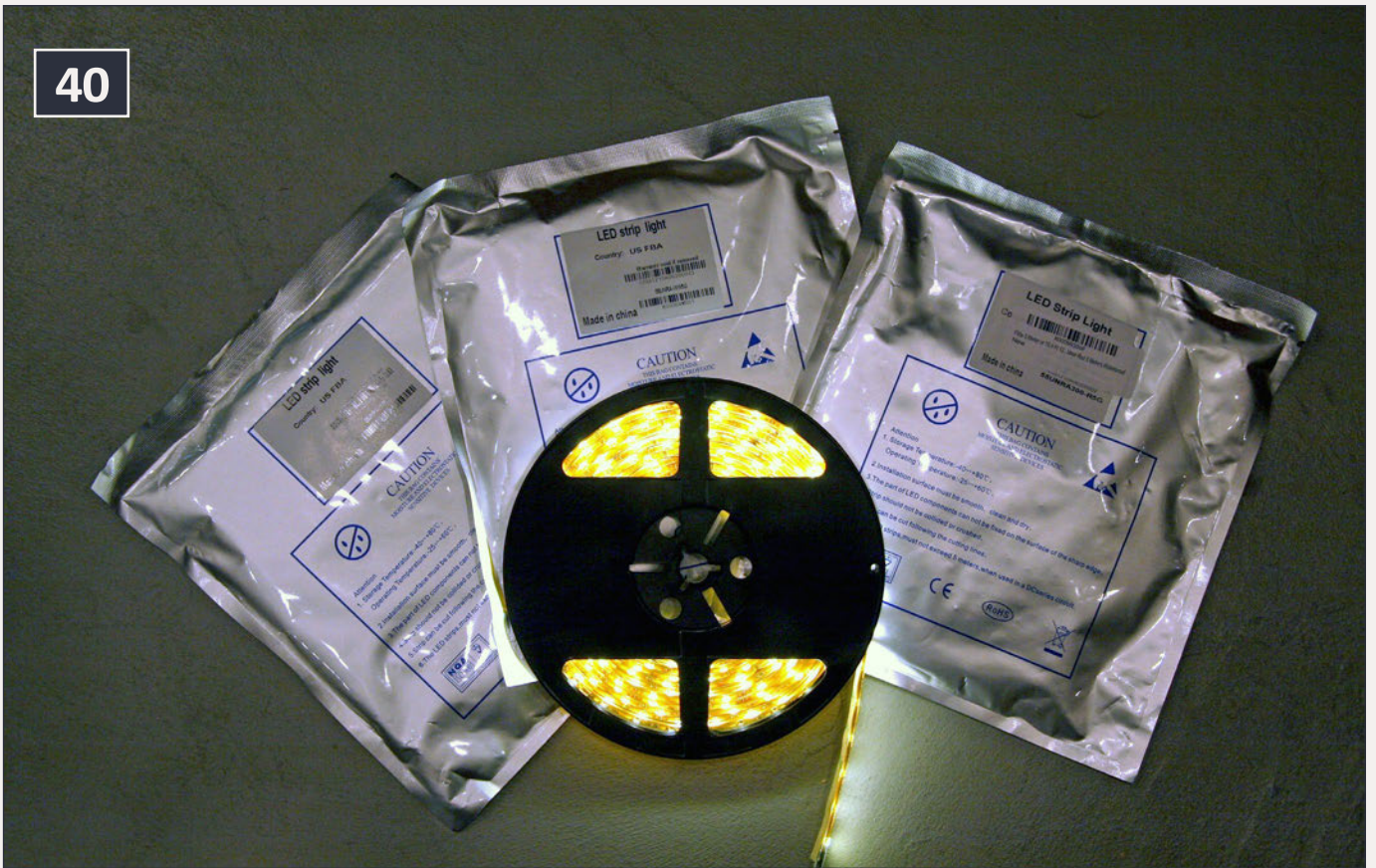
40: LED strip lights, 15' long.
