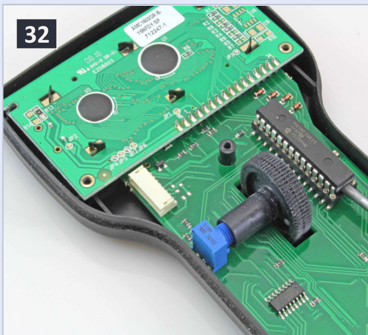
32: Removing the PowerCab chip to upgrade software.
