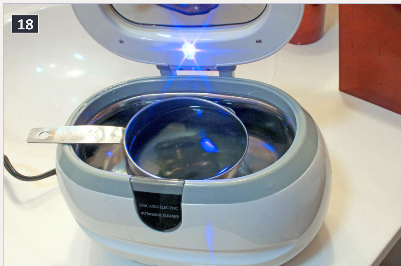
18: Cleaning drive train parts in ultrasonic cleaner.
