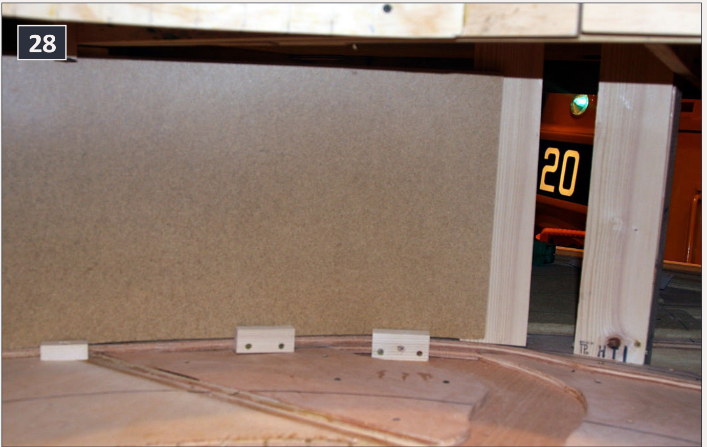
28: Backdrop supports at bottom and behind joint.
