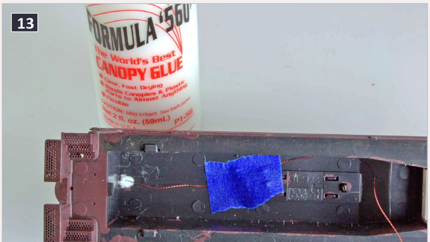
13: Front SMD LED held in place with blue tape while Canopy Glue dries.
