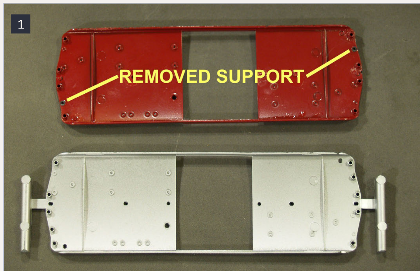
1. Showing removal of the Ladder Rung Support. Can be seen on the top roof, by darker circle where support was removed.
