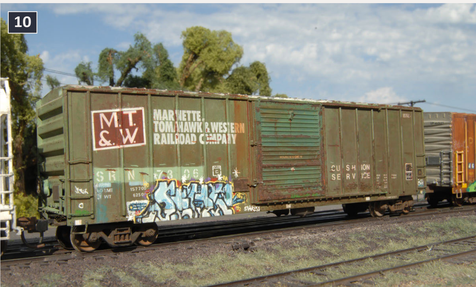
10: This Athearn 50' Pullman Standard box car was finished with PollyScale paint. The decals were custom made. The graffiti was hand-painted.
