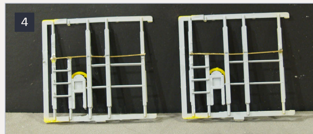
4. The added wire grab across the full width of the ends.
