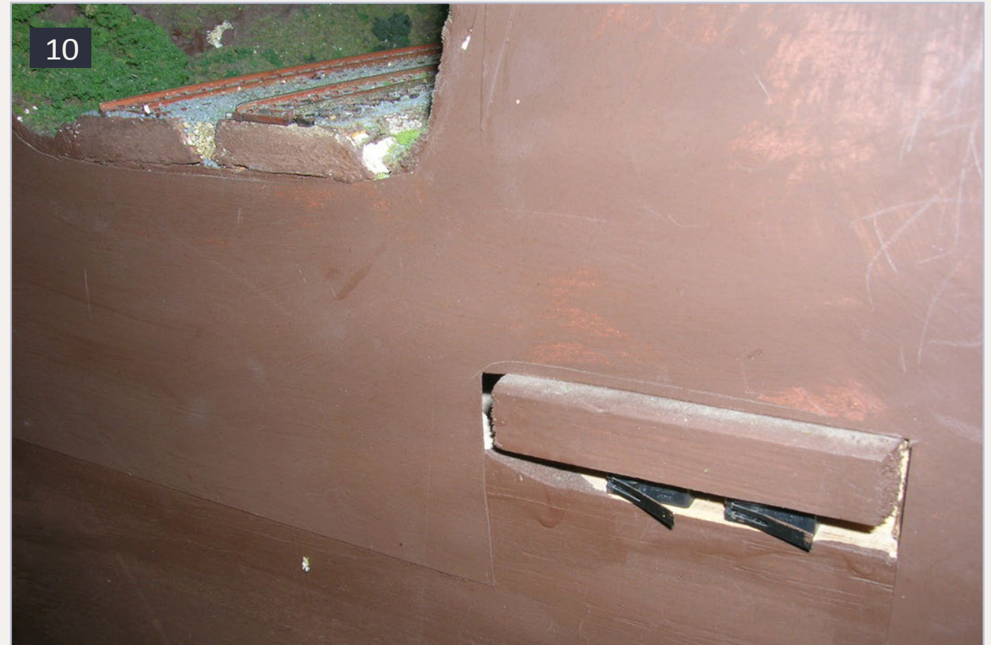
7. Detail of limit switches.
