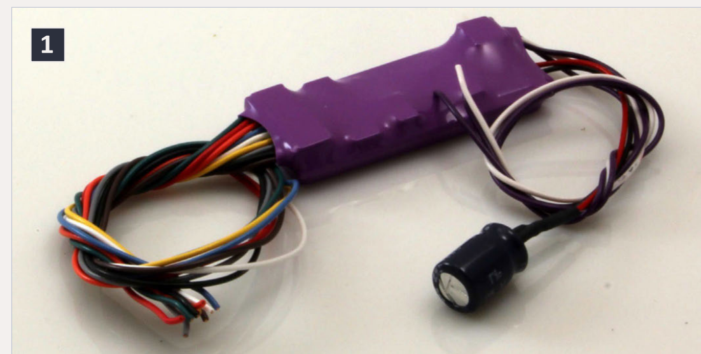
1: Wrapped decoder example – SoundTraxx Tsunami TSU-1000.
