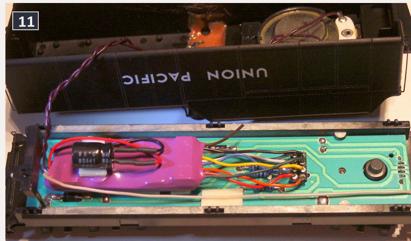
11: Tsunami decoder plugged into a Proto Heritage 2-8-8-2 tender wired to the speaker in the shell.
