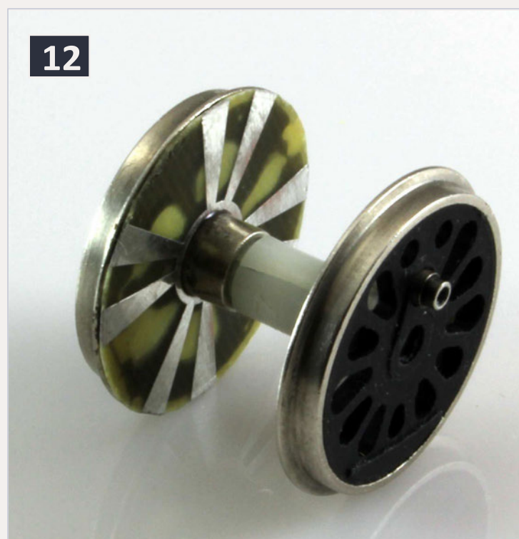
12: SoundTraxx 810038 chuff cam mounted on the inside of an HO steam driver – this is a cam for an articulated style of loco with two sets of cylinders and drivers.
