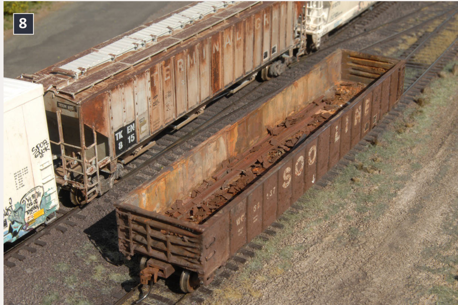
8: This model started life as a Walthers 53 foot Thrall gondola. The sides were replaced with .005 styrene. Sides were bulged /dented before painting. Decals were custom made for Soo Line wording. The interior walls were distressed with a Dremel tool to match the exterior damage to the car. The interior was painted by blotching paint to simulate anything and everything that would be spilled or loaded in this car. The load of Atlas Rail and Monster Modelworks.com scale tie plates were painted with PollyScale paint and Winsor Newton gouache.
