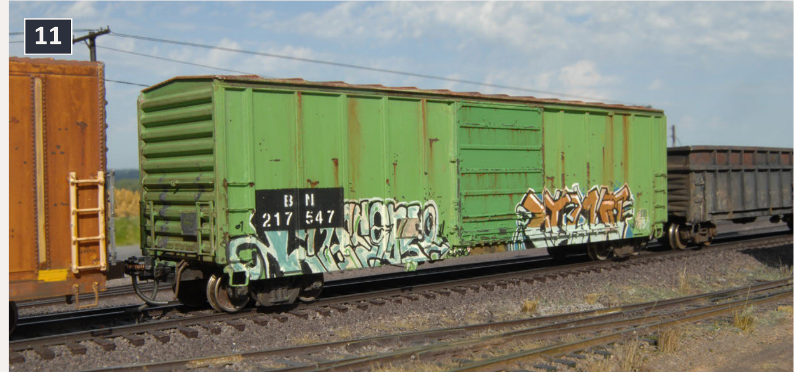
11: This is an Intermountain 5277 Pullman Standard box car custom painted a mixed green color. The graffiti is hand-painted. Microscale number sets were used for the car numbers. Door modifications were made by replacing lower door supports.
