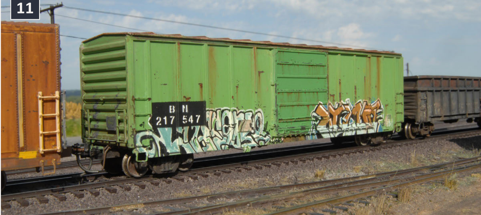
11: This is an Intermountain 5277 Pullman Standard box car custom painted a mixed green color. The graffiti is hand-painted. Microscale number sets were used for the car numbers. Door modifications were made by replacing lower door supports.
