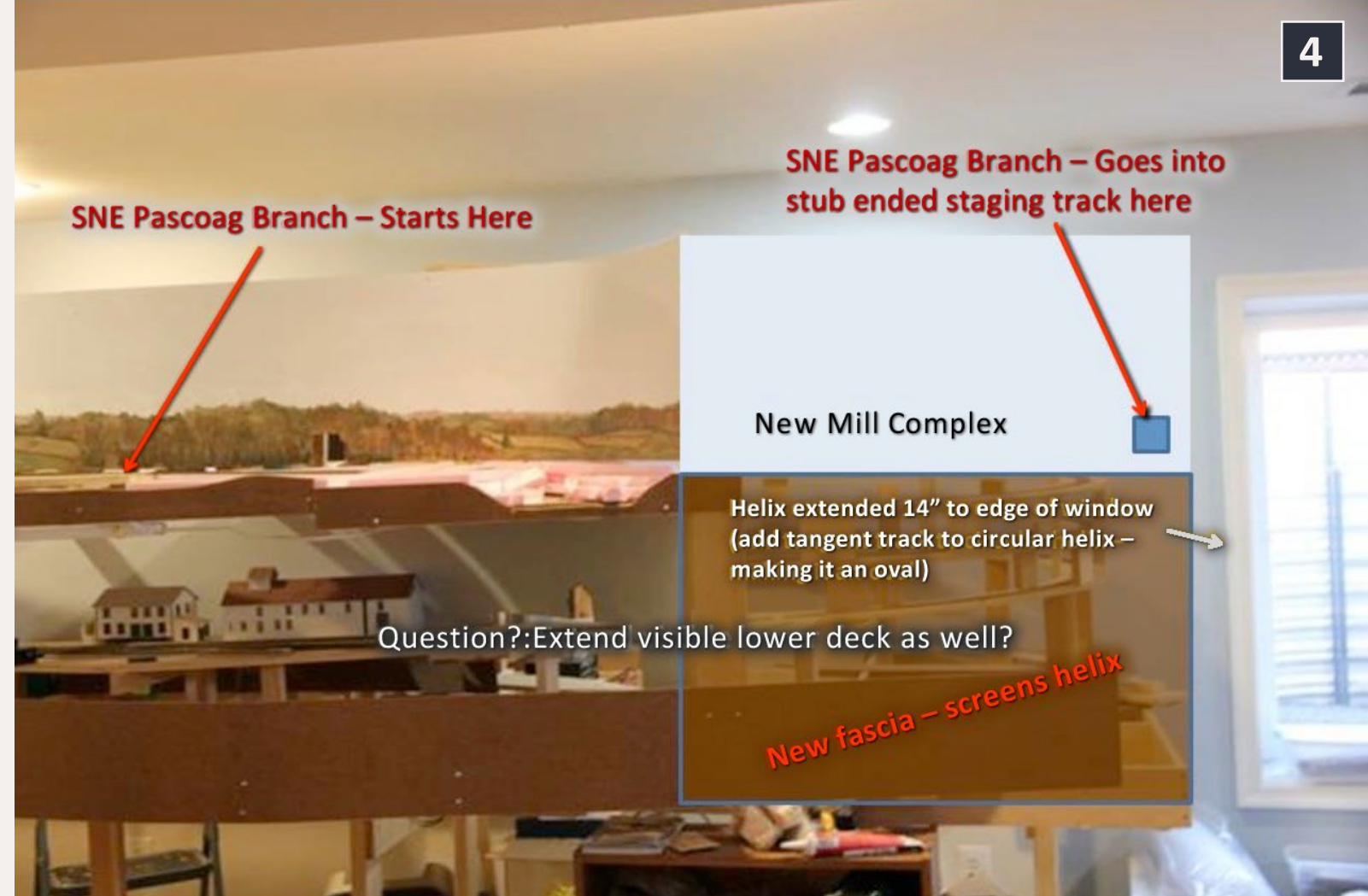
4: Diagram shows the planned changes: Boxing in the helix with an extended fascia and adding a branchline on top, essentially covering the top of the helix with scenery.
