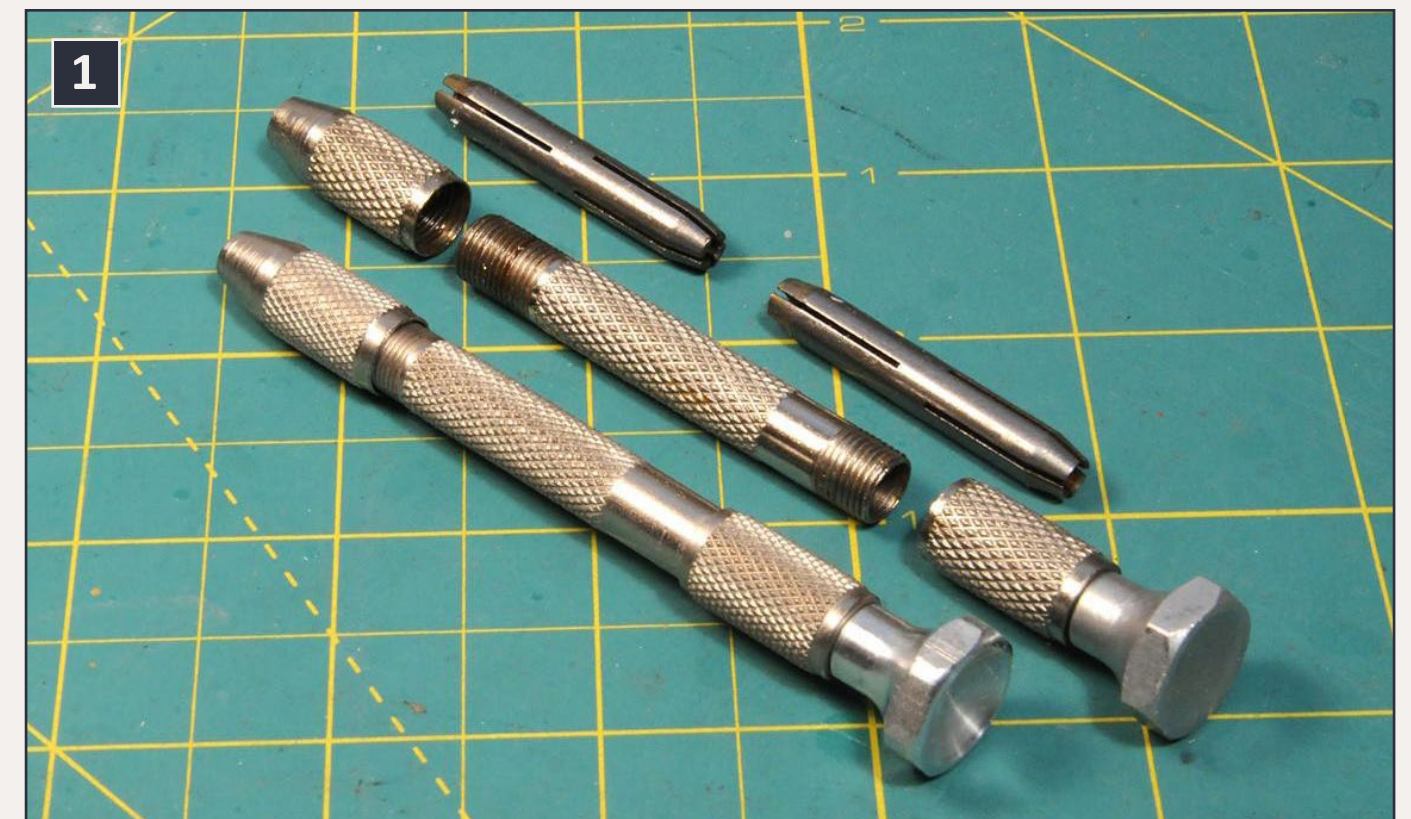
1: Here are two General Tools Swivel Head pin vises. The one on the right has been disassembled to show the collar, body, and swivel head (center) as well as the two double-ended collets (top).
