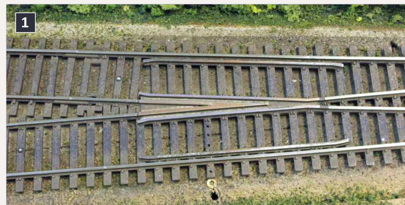
1: Insulated frog turnout – Atlas HO Code 83 #8 frog is insulated between the two black bands. Copper ring nearest the camera is provided to electrify the frog.
