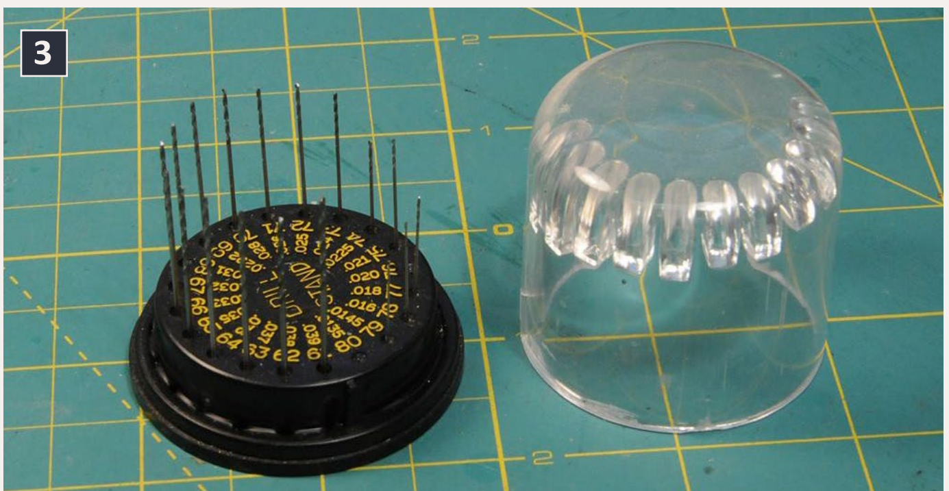
3: A Rogers Drill bit set. The size of each drill bit in inches is next to the drill bit number.
