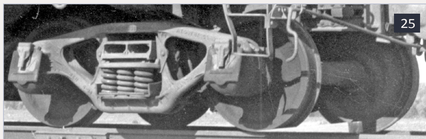
24-25: Two slightly different versions of the ARA 70-ton truck with 5'8" wheelbase, one by Symington and the other by American Steel Foundries. The ASF truck had Barber Lateral Motion devices.
