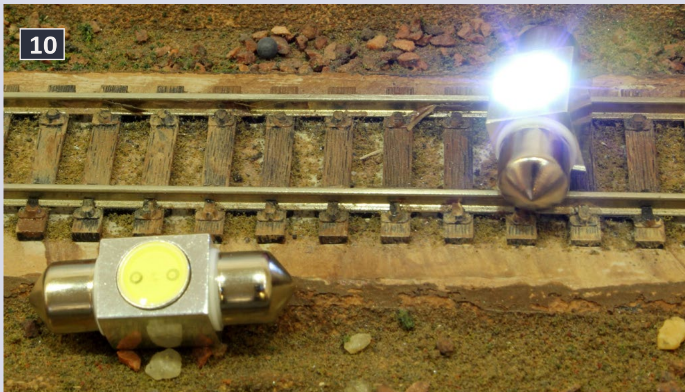
10: LED dome light testing HO track plus one off track for comparison.
