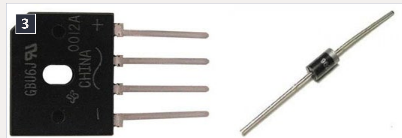
3: Bridge rectifier module vs. discrete diodes.
