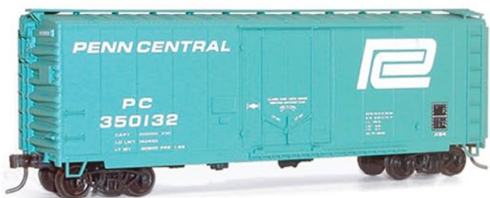
Penn Central Insulated 40' Steel Box Car
