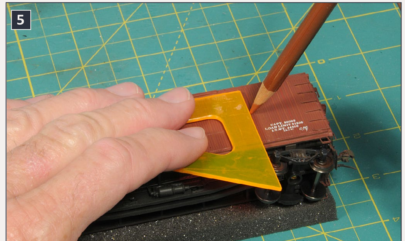
5: Here a small drafting triangle is lightly tucked up against the letterboard of this freight car so that a colored pencil can be streaked downward along the side of the car.
